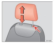
Fig. 91 Adjusting and removing the head restraints
