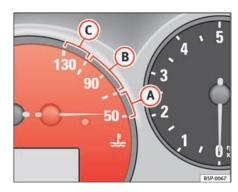
Fig. 34 Details of the instrument panel: Engine coolant temperature gauge
