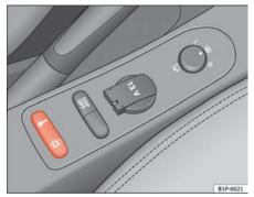
Fig. 59 Detail of rear left door central locking button
