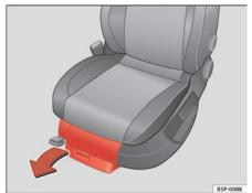
Fig. 97 Stowage area under the front seats
