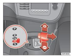
Fig. 121 Changing gear with Tiptronic
