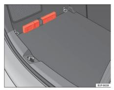
Fig. 103 Housing for the emergency warning triangle in the boot
