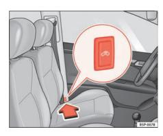
Fig. 66 Button for deactivating the interior monitoring system
