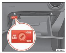
Fig. 25 In the glove box there is key switch for disabling and enabling the airbags on the front passenger side
