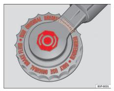
Fig. 143 In the engine compartment: Brake fluid reservoir cover
