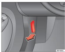
Fig. 134 Detail of the footwell: The release lever for the bonnet is located in the driver side footwell
