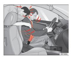
Fig. 9 The unbelted rear passenger is thrown forward violently, hitting the driver wearing a seat helt
