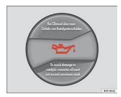
Fig. 138 In the engine compartment: Engine oil filler cap
