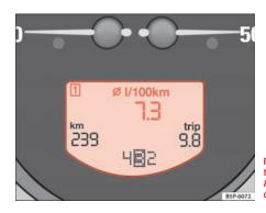
Fig. 41 Digital screen on the instrument panel: Average fuel consumption display
