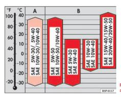
Fig. 136 Types of oil according to temperature
