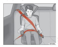
Fig. 29 Forward-facing child seat installed on rear seat
