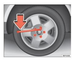
Fig. 148 Changing the wheel: Loosening the wheel bolts
