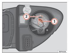
Fig. 160 Main beam headlights
