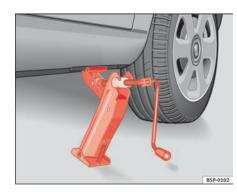
Fig. 150 Fitting the jack
