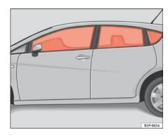
Fig. 24 Deployed curtain airbags
