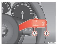
Fig. 40 Windscreen wiper and washer lever: Button
