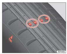
Fig. 144 Tyre tread wear indicators
