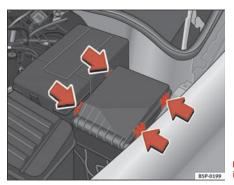
Fig. 154 Fuse box cover in engine compartment
