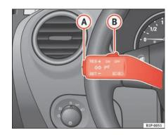
Fig. 123 Turn signal and main beam lever: Switch and rocker switch for CCS
