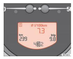
Fig. 39 Digital screen on the instrument panel: Average fuel consumption display
