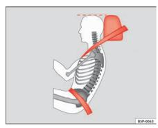
Fig. 90 Viewed from side: Properly adjusted head restraints and proper belt adjustment
