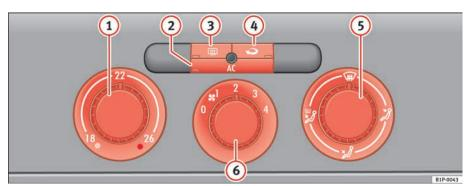
Fig. 106 On the dash panel: Climate controls
