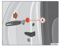
Fig. 58 Locking the doors manually
