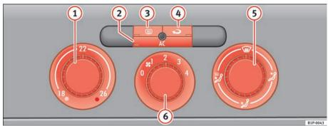
Fig. 108 On the dash panel: Climate controls
