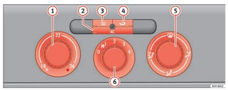
Fig. 107 On the dash panel: Climate controls
