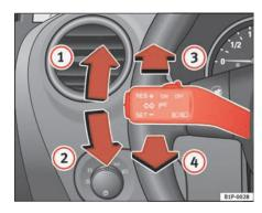
Fig. 78 Turn signal and main beam headlight
