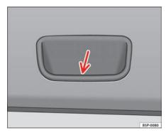
Fig. 68 Detail of the tailgate inner trim: recessed handle for closing the tailgate
