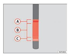
Fig. 137 Engine oil dipstick.
