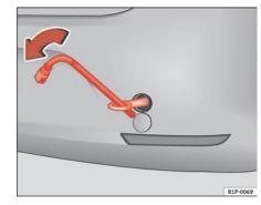
Fig. 175 Fitting the towing ring to the rear of the vehicle
