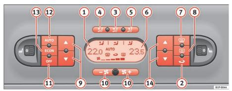
Fig. 110 On the dash panel: 2C Climatronic controls
