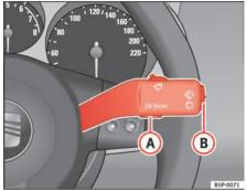
Fig. 38 Windscreen wiper and washer lever: Button
