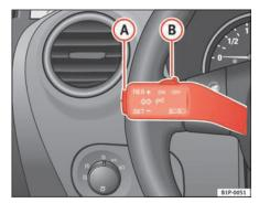
Fig. 124 Turn signal and main beam lever: switch and rocker switch for CCS
