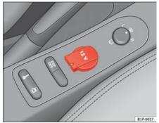
Fig. 101 Socket, centre console, front
