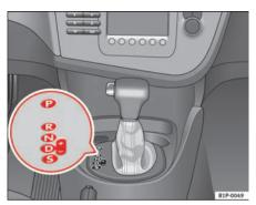
Fig. 117 Automatic gearbox: Selector lever positions
