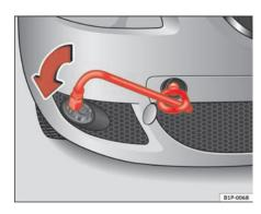
Fig. 174 The front right section of the vehicle: Fitting the front towing eve
