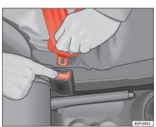
Fig. 15 Removing latch plate from buckle
