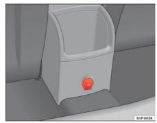
Fig. 102 Socket, centre console, rear
