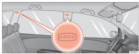
Fig. 23 Location of left curtain airbag
