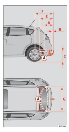
Fig. 132 Attachment points for towing bracket
