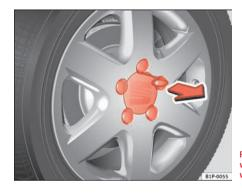
Fig. 147 Changing a wheel: Removing the wheel trim
