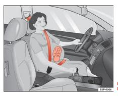
Fig. 14 Positioning seat belts during pregnancy
