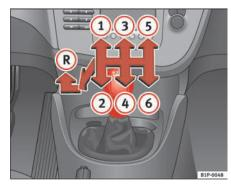
Fig. 116 Detail of the centre console: Shift diagram of a 6-speed manual gearbox
