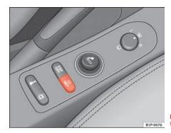
Fig. 47 Centre console: tyre control system button
