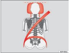
Fig. 89 Viewed from in front: Properly adjusted head restraints and proper belt adjustment
