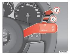
Fig. 86 Window wash and wipe lever: Rear window wiper
