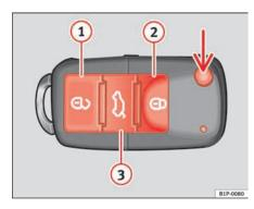
Fig. 65 Battery indicator in the remote control key
