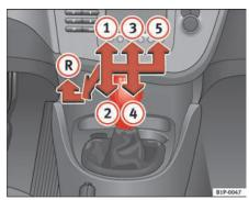
Fig. 115 Detail of the centre console: Shift diagram of a 5-speed manual gearbox
