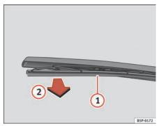
Fig. 142 Changing the rear window wiper blade
