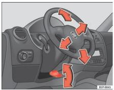
Fig. 111 Adjusting the steering wheel position
