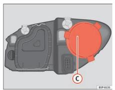
Fig. 159 Main beam headlights
