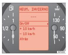
Fig. 45 Digital screen on the instrument panel: winter tyre display
