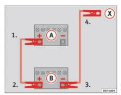
Fig. 173 How to connect the jump leads
