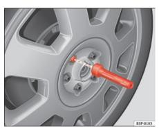
Fig. 151 Wheel change: Hexagon socket in screwdriver handle to turn the wheel bolts after they have been loosened
