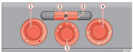
Fig. 105 On the dash panel: Heater controls
