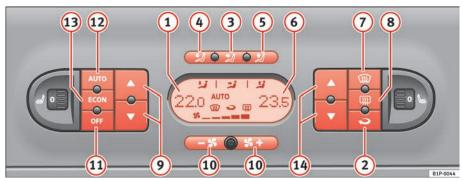
Fig. 109 On the dash panel: 2C Climatronic controls
