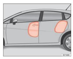
Fig. 22 Illustration of principle: inflated side airbags on left side of vehicle
