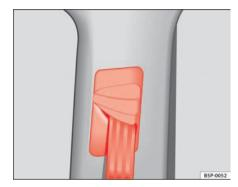
Fig. 16 Location of the belt height adjuster
