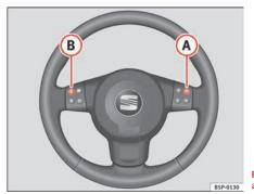
Fig. 57 Steering wheel audio version controls
