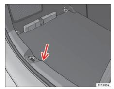
Fig. 146 Luggage compartment. Access to the spare wheel
