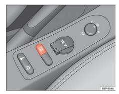
Fig. 113 Detail of the centre console: ESP button
