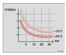
Fig. 131 Fuel consumption in litres per 100 km at two different ambient temperatures
