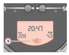
Fig. 36 Detail of instrument panel: Display with Tiptronic gear selection
