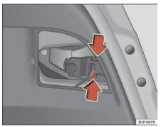
Fig. 165 Removing the lamp holders
