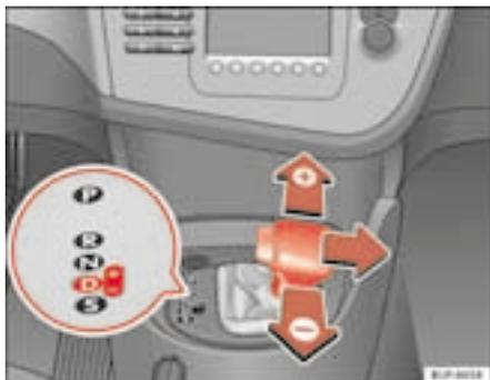
**Fig. 120** Trocar com tiptronic
