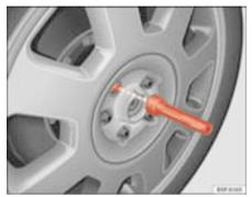
Fig. 155 Changing the wheel: Hexagonal socket tool for the bolts
