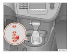
Fig. 116 Centre console: selector lever for automatic gearbox / direct shift gearbox (DSG)
