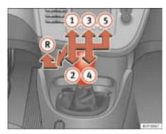
Fig. 114 Centre console: diagram for 5 speed manual gearbox
