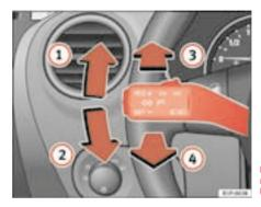
Fig. 76 Turn signal and main beam headlight
