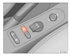
Fig. 112 Centre console: **ESP** button
