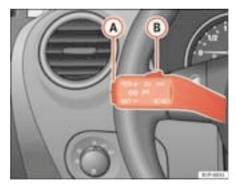
Fig. 125 Turn signal and main beam headlight lever: switch and rocker switch for the cruise control
