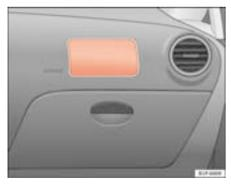
Fig. 18 Front passenger airbag located in dash panel
