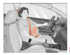
Fig. 14 Positioning seat belts during pregnancy
