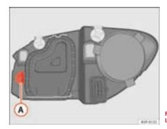
Fig. 160 Turn signal lamps
