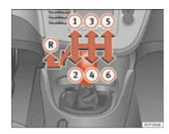
Fig. 115 Centre console: diagram for 6 speed manual gearbox
