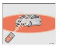
Fig. 64 Range of the remote control
