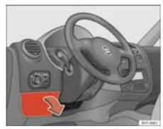
Fig. 157 Left side of dash panel: Fuse box cover
