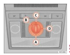
Fig. 70 Roof interior lining: closing the sliding/tilting sunroof
