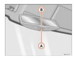
Fig. 85 Automatic antidazzle interior mirror.
