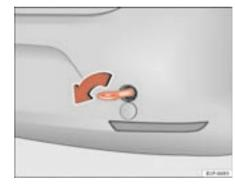
Fig. 179 Fitting the towing ring to the rear of the vehicle
