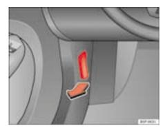
Fig. 138 Details of the driver-side foot well: bonnet release lever
