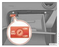
Fig. 25 In the glove compartment: there is key switch for disabling and enabling the airbags on the front passenger side
