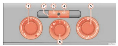
Fig. 106 On the dash panel: Climatic controls
