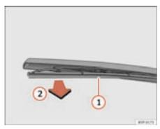
Fig. 146 Changing the rear window wiper blade
