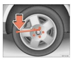
Fig. 152 Changing the wheel: loosening wheel bolts
