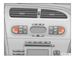
Fig. 91 Thumb wheel for the front seat heating
