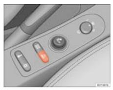
Fig. 47 Centre console: tyre monitor system button
