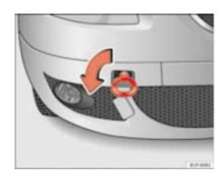
Fig. 178 The front right section of the vehicle: Fitting the front towing ring
