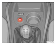
Fig. 75 Instrument panel: switch for hazard warning liahts
