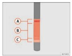
Fig. 141 Engine oil dipstick.
