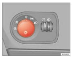
Fig. 72 Description of the instrument panel: lights control, antifog lights and rear antifog light
