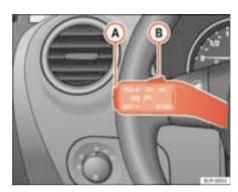
Fig. 123 Turn signal and main beam headlight lever: switch and rocker switch for the cruise control
