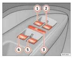
Fig. 68 Detail of the driver's door: controls for front and rear electric windows
