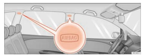
Fig. 23 Location of left curtain airbag
