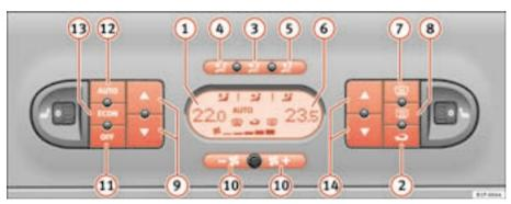
Fig. 109 On the dash panel: 2C Climatronic controls
