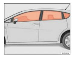
Fig. 24 Deployed curtain airbags
