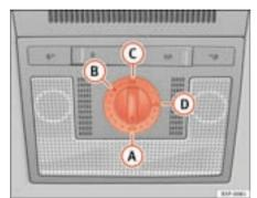
Fig. 69 Roof interior lining: closing the sliding/tilting sunroof
