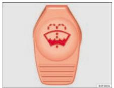
Fig. 144 In the engine compartment: Cap of windscreen washer fluid reservoir.
