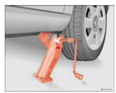
Fig. 154 Fitting the jack
