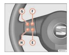
Fig. 53 Controls on the steering wheel
