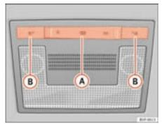
Fig. 77 Interior roof lining: front passenger compartment lighting
