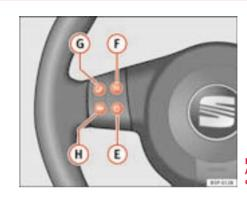
Fig. 55 Steering wheel Audio + Telephone controls
