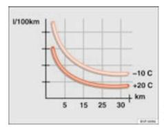
Fig. 135 Fuel consumption in litres per 100 km at two different ambient temperatures
