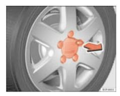
Fig. 151 Changing the wheel: Pull off the hub cap
