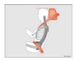
Fig. 88 Side view: headrest and seatbelt correctly adjusted
