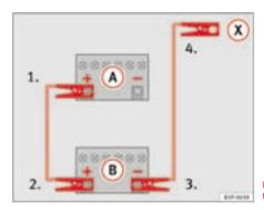
Fig. 177 How to connect the jump leads
