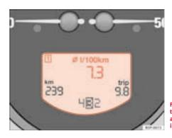
Fig. 41 Digital display in the instrument panel: average fuel consumption indicator.
