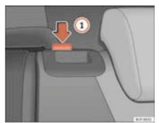
Fig. 93 Folding up the rear seat back
