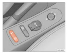
Fig. 59 Centre console: central locking button
