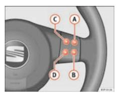
Fig. 48 Controls on the steering wheel
