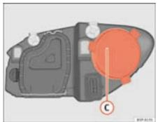
Fig. 163 Main beam headlights
