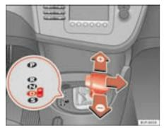
Fig. 120 Changing gear with Tiptronic
