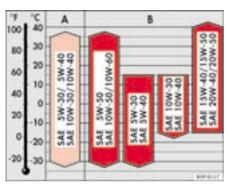
Fig. 140 Types of oil according to temperature
