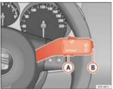
Fig. 42 Windscreen washer lever: button A to confirm the menu option and rocker switch B to change the menu
