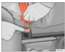
Fig. 15 Removing latch plate from buckle
