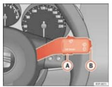
Fig. 44 Windscreen washer lever: button A to confirm the menu option and rocker switch B to change the menu
