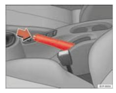
Fig. 121 Handbrake between the front seats
