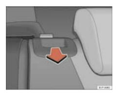
Fig. 92 Folding the seat backrests down
