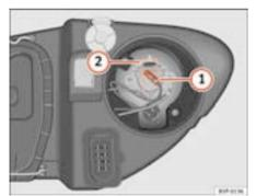
Fig. 164 Main beam headlights
