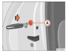
Fig. 58 Locking the doors manually
