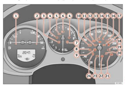
Fig. 46 Instrument panel with warning lamps. Some of the items of equipment listed here are fitted only on certain models/model years or are optional extras.
