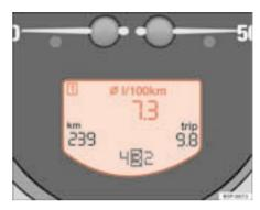
Fig. 39 Digital display in the instrument panel: average fuel consumption indicator
