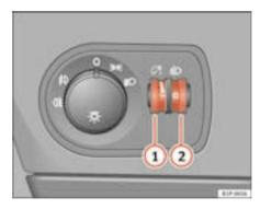
Fig. 74 Instrument panel: regulation for instrument and switch illumination and headlight range control
