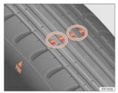
Fig. 148 Tyre tread wear indicators
