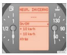
Fig. 45 Digital display in the instrument panel: winter tyres indicator
