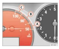
Fig. 34 Instrument panel: engine coolant temperature
