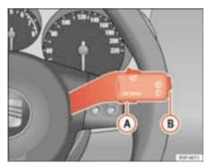
Fig. 40 Windscreen wiper and windscreen wash lever: switch A and rocker switch B
