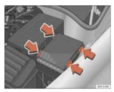
Fig. 158 Fuse box cover in engine compartment
