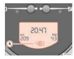
Fig. 36 Description of the instrument panel: screen with Tiptronic gear indicator
