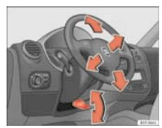
Fig. 110 Adjusting the steering wheel position
