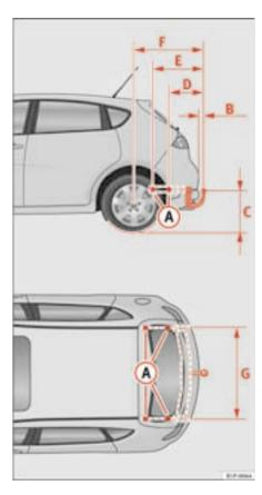
Fig. 136 Attachment points for towing bracket
