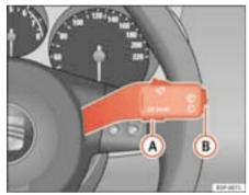
Fig. 38 Windscreen wiper and windscreen wash lever: switch A and rocker switch B
