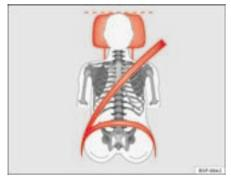
Fig. 87 Front view: headrest and seatbelt correctly adjusted
