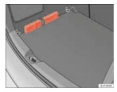
Fig. 102 Housing for the emergency warning triangle in the boot
