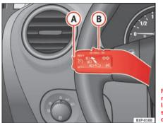
Fig. 127 Turn signal and main beam headlight lever switch and rocker switch for the cruise control
