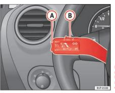
Fig. 126 Turn signal and main beam headlight lever switch and rocker switch for the cruise control
