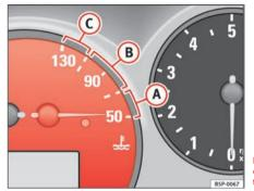
Fig. 34 Instrument panel: engine coolant temperature gauge
