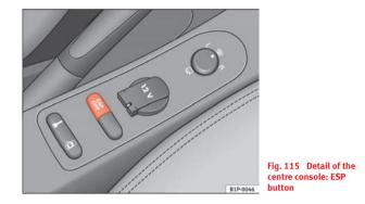
The Electronic Stabilisation Program (ESP) contains the electronic differential lock (EDL) and the traction control system (TCS). The ESP function works together with the ABS. Both warning lamps will light up if the ESP or ABS systems are faulty.
