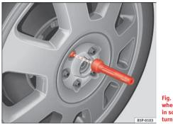
Fig. 158 Changing the wheel: Hexagonal socket in screwdriver handle to turn the wheel bolts
