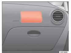
Fig. 18 Front passenger airbag located in dash panel
