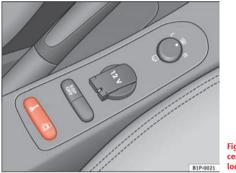
Fig. 59 Detail of the centre console: central locking system button
