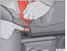
Fig. 15 Removing latch plate from buckle
