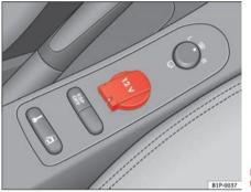
Fig. 101 Power point, front centre console
