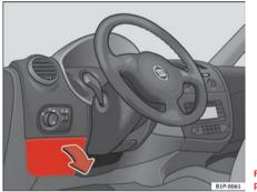
Fig. 160 Left side of dash panel: Fuse box cover
