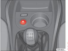
Fig. 76 Instrument panel: switch for hazard warning lights
