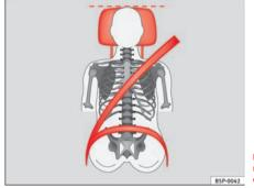
Fig. 88 Front view: head restraints and seat belts correctly adjusted
