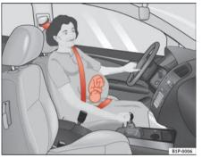
Fig. 14 Positioning seat belts during pregnancy
