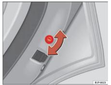
Fig. 61 Child safety lock on the right hand side door This function is independent of the vehicle electronic opening and locking systems. It only affects rear doors. It can only be activated and deactivated manually, as described below:
