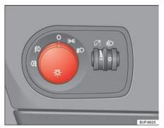
Fig. 72 Detailed view of dash panel lights, fog light and rear fog light control
