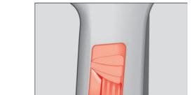
Fig. 16 Location of the belt height adjuster
