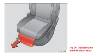
The locker\*  $\Rightarrow$  fig. 96 (A) is opened by pulling on the cover.
