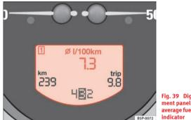
Fig. 39 Digital instrument panel display: average fuel consumption indicator
