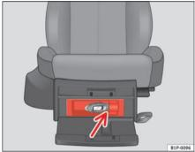
Fig. 104 USB\* connection below passenger seat
