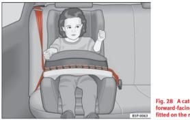
Fig. 28 A category 1 forward-facing child seat fitted on the rear seat.
