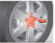
Fig. 154 Changing the wheel: Removing a hub cap
