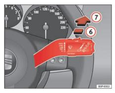
Fig. 85 Windscreen wiper and windscreen wash lever: rear window wiper
