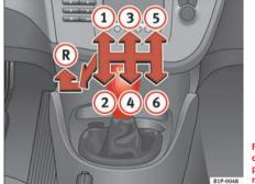
Fig. 118 Detail of the centre console: gear shift pattern of a 6-speed manual gearbox
