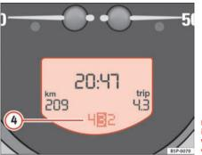
Fig. 36 Detail of the instrument cluster: screen with Tiptronic gear indicator
