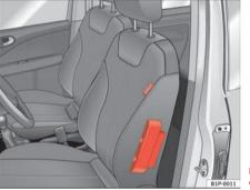
Fig. 21 Side airbag in driver seat
