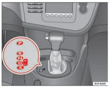
Fig. 119 Centre console: selector lever for automatic gearbox / direct shift gearbox DSG
