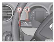
Fig. 136 Indicator and main beam headlight lever: switch and rocker switch for the cruise control
