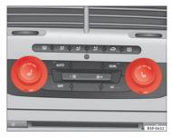
Fig. 93 Front seat heating with Climatronic
