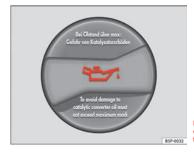
Fig. 146 In the engine compartment: Engine oil filler cap
