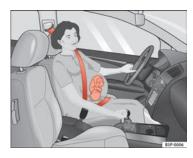
Fig. 14 Positioning seat belts during pregnancy
