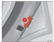
Fig. 61 Child safety lock on the right hand side
