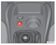
Fig. 76 Instrument panel: switch for hazard warning lights
