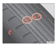
Fig. 153 Tyre tread wear indicators
