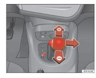
Fig. 128 Changing gear with Tiptronic
