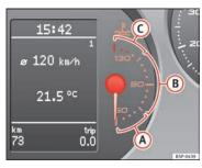
Fig. 34 Dash panel engine coolant temperature gauge
