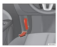
Fig. 142 Detail of footwell area on driver's side: lever for unlocking the bonnet.
