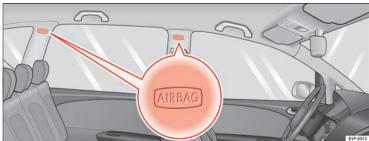
Fig. 23 Location of left curtain airbag
