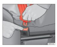
Fig. 15 Removing latch plate from buckle
