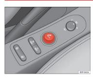
Fig. 100 The cigarette lighter is located in the electric socket on the front of the centre console
