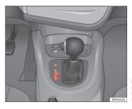
Fig. 124 Centre console: selector lever for automatic gearbox / direct shift gearbox DSG
