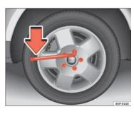
Fig. 157 Changing the wheel: loosen the wheel holts
