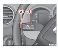
Fig. 134 Indicator and main beam headlight lever: switch and rocker switch for the cruise control
