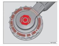
Fig. 152 In the engine compartment: Brake fluid reservoir cover
