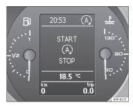
Fig. 121 Display on the dash panel during Start-Stop function operation.
