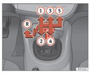
Fig. 122 Detail of the centre console: gear shift pattern of a 5-speed manual gearbox
