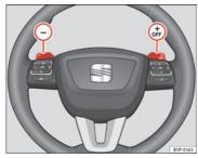
Fig. 129 Steering wheel with levers for automatic gearbox
