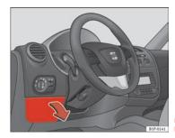
Fig. 162 Left side of dash panel: Fuse box cover
