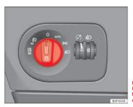
Fig. 72 Detailed view of instrument panel: lights, fog light and rear fog light control
