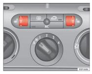
Fig. 92 Thumb wheel for the front seat heating
