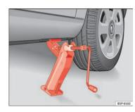
Fig. 159 Fitting the jack
