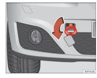
Fig. 183 The front right section of the vehicle: Fitting the front towing
