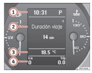
Fig. 37 Digital display in the dash panel
