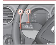
Fig. 135 Indicator and main beam headlight lever: switch and rocker switch for the cruise control
