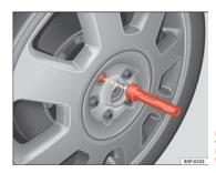
Fig. 160 Changing the wheel: Hexagonal socket in screwdriver handle to turn the wheel bolts
