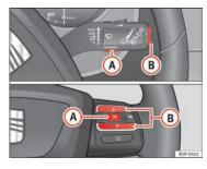
Fig. 39 Rocker buttons A and B. Steering wheel controls.
