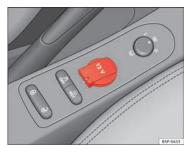
Fig. 101 Socket, centre console, front
