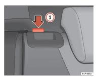
Fig. 95 Folding up the rear seat back
