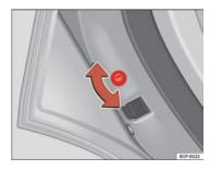
Fig. 60 Child safety lock on the left hand side door
