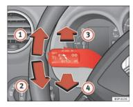
Fig. 77 Indicator and main beam headlight lever
