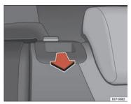
Fig. 94 Folding the seat backrests down
