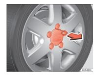
Fig. 156 Changing the wheel: Removing a hub cap
