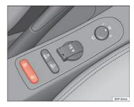
Fig. 58 Detail of the centre console: central locking system button
