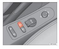
Fig. 117 Detail of the centre console: ESP button
