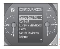
Fig. 47 Multifunction display (MFD) dash panel display.
