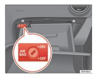
Fig. 25 In the glovebox: key for enabling and disabling front passenger airbag
