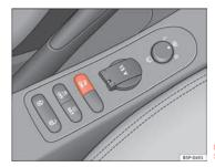
Fig. 131 Centre console: Switch for parking aid
