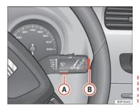
Fig. 43 Windscreen wiper lever: button A to confirm the menu selection and rocker switch B to change the menu
