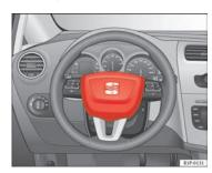
Fig. 17 Driver airbag located in steering wheel
