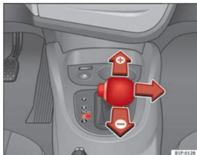
Fig. 127 Engrenar com tiptronic
