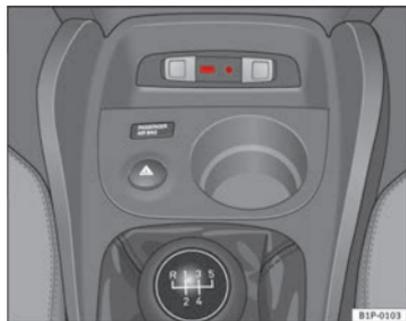
Fig. 103 Conector na consola central
