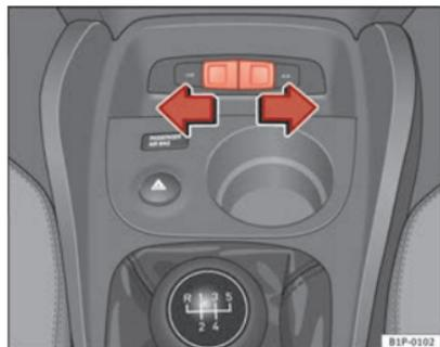
Fig. 102 Abertura do conector na consola central
