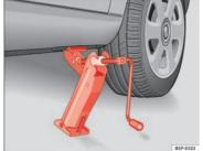
Fig. 158 Fitting the jack
