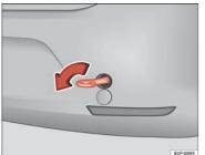
Fig. 183 Fitting the towing eye to the rear of the vehicle
