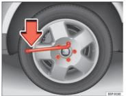
Fig. 156 Changing the wheel: loosen the wheel bolts
