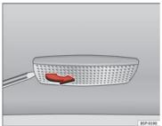
Fig. 178 Removing sun visor light
