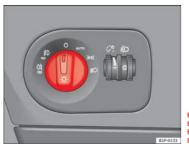
Fig. 71 Detailed view of the dash panel: lights, fog lights and rear fog light switch
