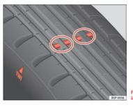
Fig. 152 Tyre tread wear indicators
