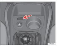
Fig. 26 Warning lamp for deactivated passenger airbag in centre console
