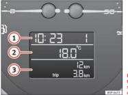
Fig. 36 Detailed view of the instrument panel: screen with different indicators
