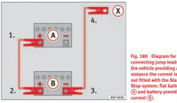
connecting jump leads if the vehicle providing assistance the current is not fitted with the Start-Stop system: flat battery (A) and battery providing current (B).
