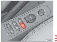
Fig. 118 Centre console: gas system control switch.
