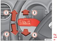
Fig. 76 Turn signal and main beam headlight lev-
