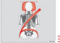
Fig. 12 Correct seat belt and head restraint positions, viewed from front
