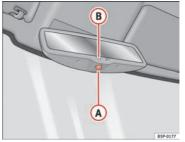
Fig. 85 Automatic antidazzle interior mirror.
