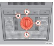
Fig. 68 Roof lining description: sliding/tilting sunroof rotary knob
