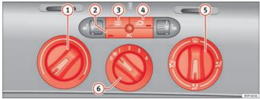
Air recirculation mode  $\Rightarrow$  fig. 109 (a) prevents strong odours in the outside air from entering the vehicle interior, for example when passing through a tunnel or in queuing traffic.
