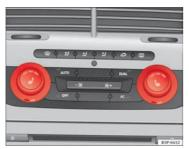
Fig. 92 Front seat heating with Climatronic
