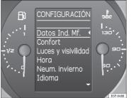
Fig. 47 Multifunction display (MFI) instrument panel display.
