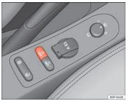
Fig. 116 Detailed view of the centre console: ESC (ESP) button
