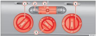
Fig. 106 Heating controls on the dash panel
