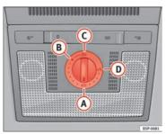
Fig. 69 Roof lining description: sliding/tilting sunroof rotary knob
