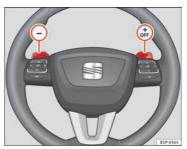
Fig. 128 Steering wheel with levers for automatic gearbox
