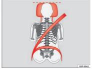
Fig. 87 Front view: head restraints and seat belts correctly adjusted
