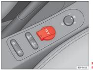
Fig. 100 Power socket, front centre console
