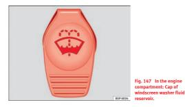
The **windscreen washer** and the **headlight washers** are supplied with fluid from the windscreen washer fluid container in the engine compartment.
