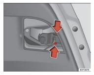
Fig. 172 Removing the bulb holder
