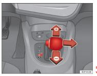
Fig. 127 Changing gear with tiptronic
