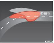
Fig. 74 Cornering lighting using adaptive headlights
