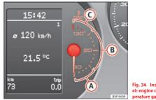
Fig. 34 Instrument panel: engine coolant temperature gauge
