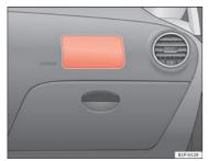
Fig. 18 Front passenger airbag located in dash panel The front airbag for the driver is located in the steering wheel  $\Rightarrow$  fig. 17 and the airbag for the front passenger is located in the dash panel  $\Rightarrow$  fig. 18. Airbags are identified by the word "AIRBAG".
