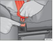
Fig. 15 Removing latch plate from buckle
