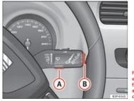
Fig. 43 Windscreen wiper lever: button A to confirm the menu selection and rocker switch B to change the menu
