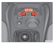
Fig. 102 Opening connector on centre console
