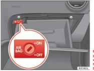
Fig. 25 In the glove compartment: switch for activating and deactivating the front passenger airbag
