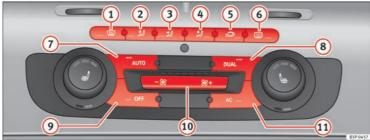
457 Fig. 110 On the dash panel: 2C Climatronic controls
