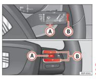
Fig. 41 Rocker buttons A and B. Steering wheel controls.
