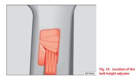
The seat belt adjuster for the front seats can be used to adjust the proper belt position at the shoulder.
