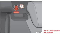
Fold the backrest back and push the backrest firmly into the lock. The red marking should no longer be visible ⇒ fig. 94.
