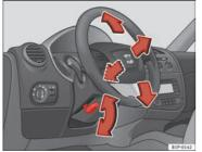
Fig. 114 Adjusting the steering wheel position
