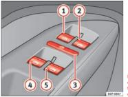
Fig. 67 Detail of the driver door: controls for the front and rear windows
