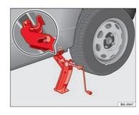
Fig. 144 Fitting the jack
