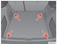
Fig. 93 Location of fastening rings in luggage compartment
