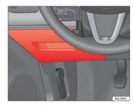
Fig. 146 Fuses in the dash panel
