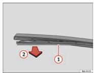
Fig. 137 Changing the rear window wiper blade
