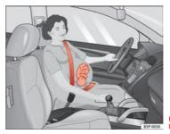
Fig. 14 Positioning seat belts during pregnancy
