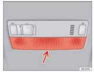
Fig. 165 Front reading light
