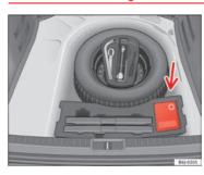
Fig. 91 Housing for the first-aid kit in the luggage compartment.
