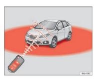
Fig. 47 Range of the remote control
