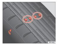
Fig. 139 Tyre tread wear indicators
