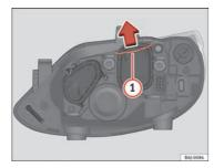
Fig. 151 Dipped beam headlights
