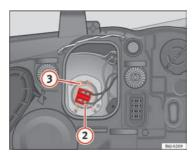
Fig. 152 Dipped beam headlights
