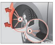
Fig. 172 Fog light: access to the connector and to the light bulb holder
