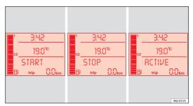
Fig. 113 Display on the instrument panel during Start-Stop function operation.
