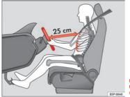
Fig. 1 The correct distance between driver and steering wheel
