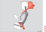
Fig. 4 Correctly adjusted head restraint viewed from the side Adjust the head restraint correctly in order to achieve maximum protection.
