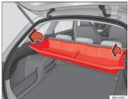
Fig. 100 Removing storage compartment
