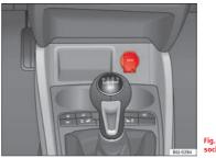
Fig. 90 Front power socket
