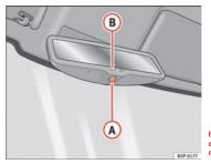
Fig. 69 Automatic antidazzle interior rear vision mirror.
