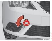
Fig. 190 Fitting the towline anchorage to front of the vehicle
