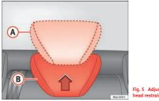
Fig. 5 Adjusting the rear head restraints
