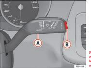
Fig. 35 Windscreen wiper and windscreen wash lever: button A and rocker switch B
