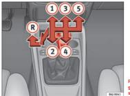
Fig. 114 Centre Console: gear shift pattern of a 5speed manual gearbox
