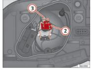
Fig. 158 Dipped beam/ main beam, single headlight
