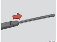
Fig. 142 Removing the rear window wiper blade
