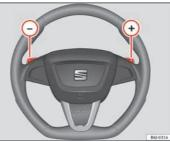
Fig. 120 Steering wheel with paddle levers for automatic gearbox
