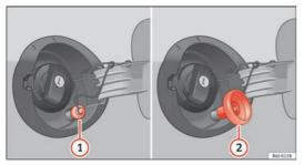
Fig. 131 Fuel tank open with LPG filler neck and adapter
