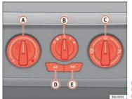
Fig. 105 Air conditioning controls on the dash panel
