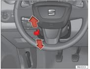
Fig. 108 Steering column height adjustment
