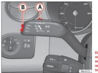
Fig. 126 Turn signal and main beam headlight lever: switch and rocker switch for the cruise control
