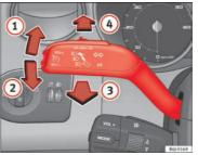
Fig. 62 Turn signal and main beam headlight lever
