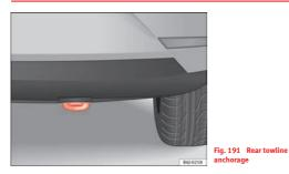
There is a towline anchorage at the rear on the right below the rear bumper.
