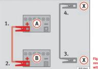
Fig. 189 Diagram of connections for vehicles with Start-Stop system.
