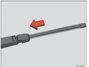
Fig. 143 Fitting the rear window wiper blade
