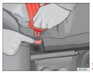
Fig. 15 Remove latch plate from buckle
