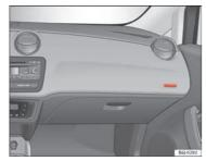
Fig. 17 Front passenger airbag located in dash panel The front airbag for the driver is located in the steering wheel  $\Rightarrow$  Fig. 16 and the airbag for the front passenger is located in the dash panel  $\Rightarrow$  Fig. 17. Airbags are identified by the word "AIRBAG".
