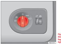
Fig. 56 Detailed view of the dash panel: lights, fog lights and rear fog light switch
