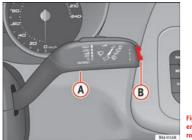
Fig. 34 Windscreen wiper lever: button A and rocker switch B
