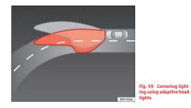
This cornering light gives better illumination of the side of the road and the corner area. The dynamic lighting is controlled automatically according to speed and the steering wheel angle.
