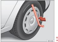
Fig. 147 Remove the complete hub cap
