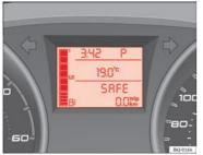
Fig. 36 Digital display: Gearbox lever position for automatic gearbox.
