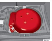
Fig. 132 LPG tank in spare wheel well
