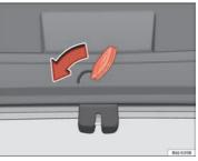
Fig. 51 IBIZA ST: Unlocking the rear lid manually There is a groove in the luggage compartment allowing access to the emergency opening mechanism.
