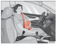
Fig. 14 Positioning seat belts during pregnancy
