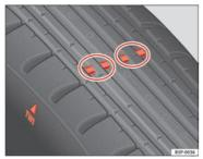
Fig. 145 Tyre tread wear indicators
