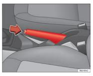
Fig. 122 Handbrake between the front seats
