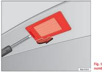
Fig. 184 Remove the number plate light.
