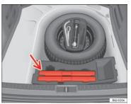
Fig. 94 Housing for the emergency warning triangle in the luggage compartment.
