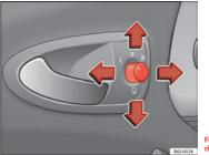
Fig. 70 Controls of exterior mirrors
