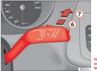
Fig. 68 Windscreen wiper and windscreen wash lever: rear window wiper
