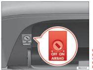
Fig. 21 In the glove compartment: switch for activating and deactivating the front passenger airbag
