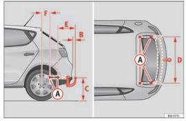
Fig. 129 IBIZA / IBIZA SC: Attachment points for towing bracket
