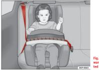
Fig. 24 A category 1 forward-facing child seat fitted on the rear seat
