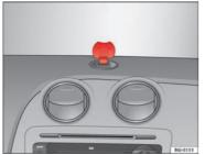
Fig. 83 Bracket with open cover for placing the navigator.
