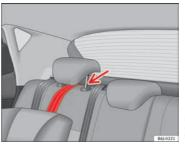
Fig. 28 Retainer strap: correct adjustment and fitting
