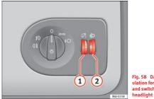
Fig. 58 Dash panel: regulation for instrument and switch lighting and headlight range control
