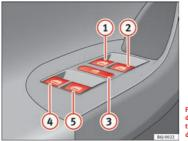
Fig. 52 Detail of the driver door: controls for the front and rear windows (5-door vehicles)
