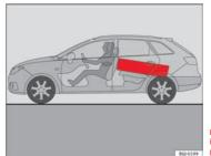
Fig. 96 Position heavy items as far forward as possible. To maintain safe handling on the road, please observe the following points:
