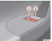
Fig. 53 Detail of the driver door: controls for the front windows (3door vehicles)
