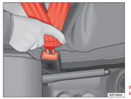
Fig. 11 Belt buckle and latch plate of seat belt
