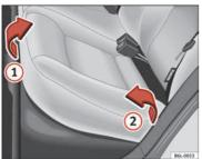
Fig. 77 Folding up the rear seat cushion
