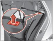
Fig. 78 Button for unlocking the rear backrest
