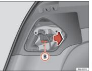
Fig. 180 Removing the bulb holder
