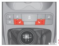
Fig. 76 Front seats heating switch
