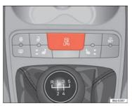
Fig. 111 Centre console: gas system control switch.
