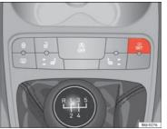
Fig. 40 Centre console: tyre monitor system button
