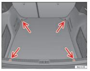
Fig. 97 Location of fastening rings in luggage compartment
