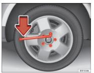
Fig. 148 Changing a wheel: loosen the wheel bolts
