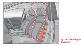
The side airbags are located in the driver seat and front passenger seat backrests  $\Rightarrow$  Fig. 20. The locations are identified by the text "AIRBAG" in the upper region of the backrests.
