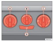
Fig. 103 Heating controls on the dash panel
