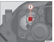
Fig. 164 Main beam headlights
