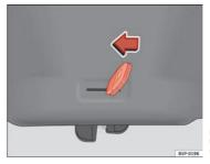
Fig. 50 IBIZA / IBIZA SC: Unlocking the rear lid manually
