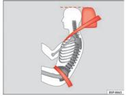
Fig. 13 Correct seat belt and head restraint positions, viewed from side
