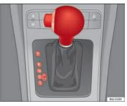
Fig. 119 Changing gear with tiptronic
