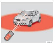
Fig. 47 Range of the radio frequency remote control
