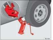
Fig. 150 Fitting the jack
