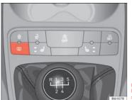
Fig. 60 Centre console: heated rear window switch
