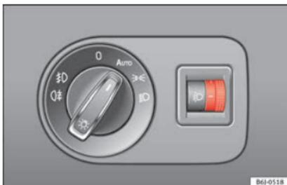
Fig. 134 Dash panel: headlight range control
