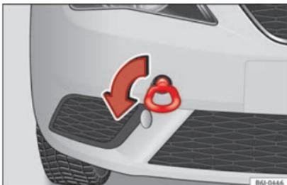
**Fig. 90** Towline anchorage at the front of the vehicle
