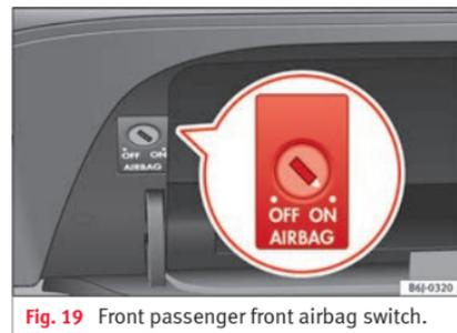
**Fig. 19** Front passenger front airbag switch.
