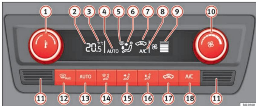
**Fig. 167** Climatronic: controls.
