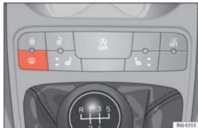
**Fig. 136** Centre console: heated rear window switch.
