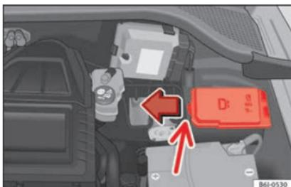
**Fig. 58** In the engine compartment: fuse box cover
