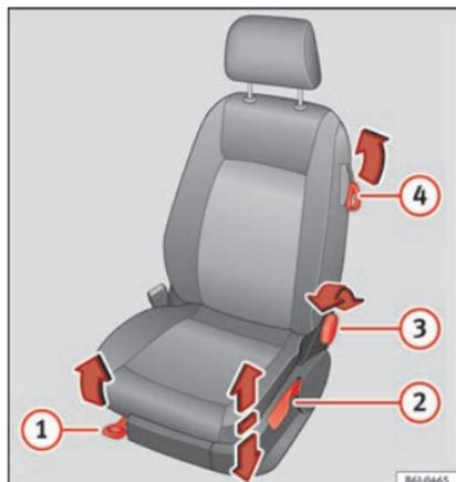
Fig. 11 Front seats: manual seat adjustment.
