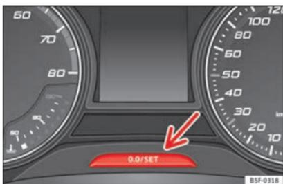
**Fig. 122** Instrument panel: odometer and reset button.
