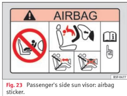
**Fig. 23** Passenger's side sun visor: airbag sticker.
