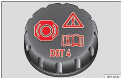
**Fig. 55** Engine compartment: brake fluid reservoir cap
