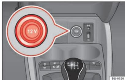
Fig. 154 Front power socket.
