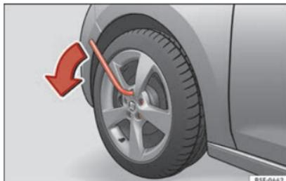
**Fig. 65** Wheel: loosen the wheel bolts.
