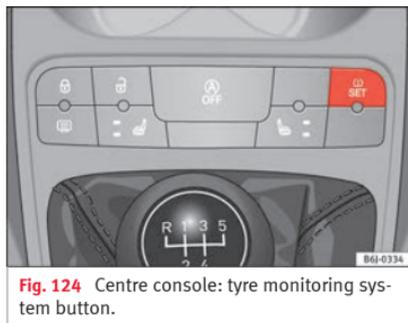
Fig. 124 Centre console: tyre monitoring system button.
