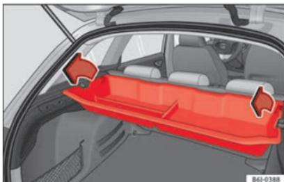
**Fig. 160** Luggage compartment: removing storage compartment.
