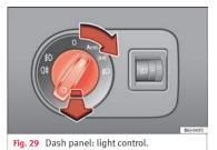
Turn the switch to the required position »» Fig. 29.
