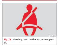
The control lamp illuminates to remind the driver to fasten his seat belt.
