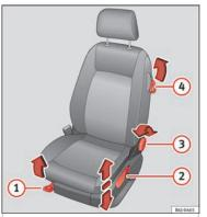
Fig. 10 Front seats: manual seat adjustment.
