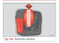
The selector lever lock in position P or N prevents gears from being engaged inadvertently, which would cause the vehicle to move.
