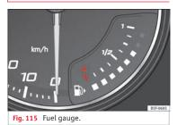
The display (6) **\*\*** Fig. 113 only works when the ignition is switched on. When the display reaches the reserve mark, the lower diode lights up in red and the control lamp  $\mathbb{B}$  appears **\*\*** page 94. When the fuel level is very low, the lower diode flashes in red. The distance to empty fuel level is displayed on the instrument panel (3) **\*\* Fig. 113**.
