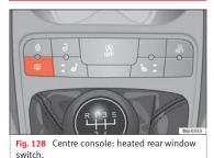
The heated rear window only works when the engine is running. When it is switched on, a lamp lights up on the switch.
