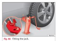
Place the jack\* (vehicle tools) on firm ground. If necessary use a large, strong board or similar support. If the surface is slippery (for example tiles) place the jack on a rubber mat or similar to prevent it from slipping » △.
