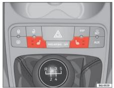
Fig. 68 Front seats heating switch
