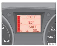
Fig. 34 Digital display: Selector lever position for the automatic gearbox.
