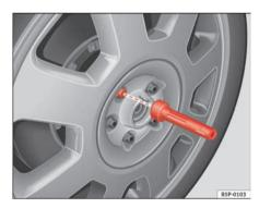
Fig. 138 Changing the wheel: Hexagonal socket in screwdriver handle to turn the wheel bolts
