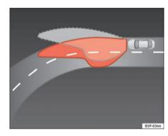
Fig. 52 Cornering lighting using self-directional headlights
