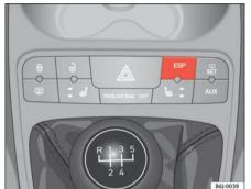
Fig. 92 Detail of the centre console: ESP button
