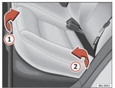
Fig. 69 Folding up the rear seat cushion
