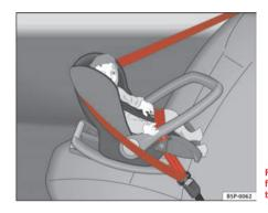
Fig. 25 A group 0 rearfacing child seat fitted on the rear seat.
