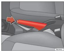
Fig. 101 Handbrake between the front seats
