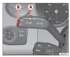
Fig. 106 Indicator and main beam headlight lever: switch and rocker switch for the cruise control
