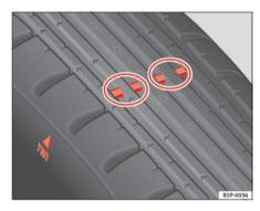
Fig. 132 Tyre tread wear indicators
