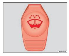
Fig. 128 In the engine compartment: Cap of windscreen washer fluid reservoir.
