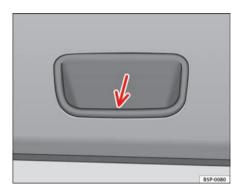
Fig. 45 Detail of the inside of the tailgate: hand grip
