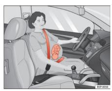
Fig. 14 Positioning seat belts during pregnancy
