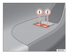
Fig. 47 Detail of driver door: controls for the front windows.
