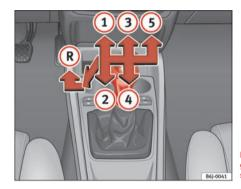
Fig. 94 Centre Console: gear shift pattern of a 5speed manual gearbox
