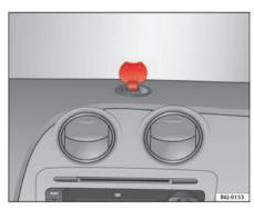
Fig. 74 Bracket with open cover for placing the navigator.
