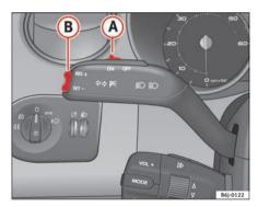
Fig. 105 Turn signal and main beam headlight lever switch and rocker switch for the cruise control
