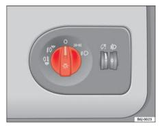
Fig. 50 Detailed view of dash panel: lights, fog light and rear fog light control
