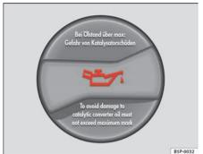
Fig. 126 In the engine compartment: Engine oil filler cap
