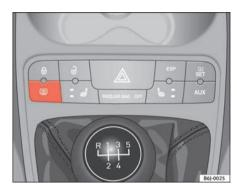
Fig. 53 Centre console: heated rear window switch
