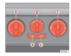
Fig. 89 Air conditioning controls on the instrument panel
