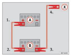
Fig. 163 How to connect the jump leads
