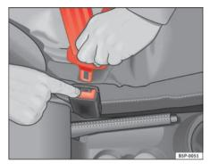
Fig. 15 Removing latch plate from buckle
