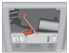
Fig. 49 Emergency operation of the panoramic/ tilting roof
