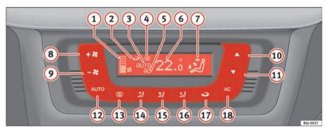
Fig. 90 Climatronic controls on the instrument panel
