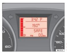
Fig. 100 Automatic gearbox: Display in the dash panel
