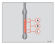
Fig. 125 Engine oil dipstick
