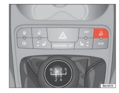
Fig. 37 Centre console: tyre monitor system button
