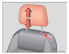
Fig. 66 Adjusting and removing the head restraints
