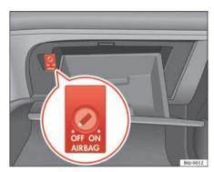
Fig. 23 In the glovebox: key for enabling and disabling front passenger airbag
