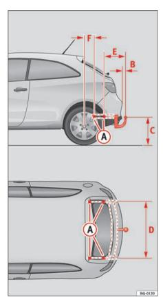
Fig. 120 Attachment points for towing bracket
