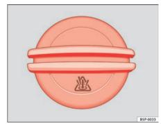
Fig. 127 In the engine compartment: Coolant expansion tank cap
