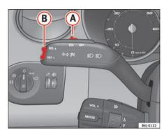
Fig. 103 Indicator and main beam headlight lever: switch and rocker switch for the cruise control
