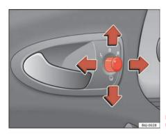
Fig. 63 Controls of exterior mirrors
