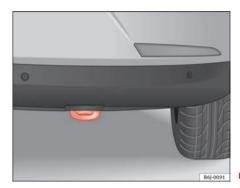
Fig. 165 Rear towing ring
