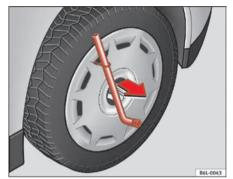
Fig. 134 Remove the complete hub cap
