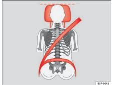
Fig. 64 Front view: head restraints and seat belts correctly adjusted
