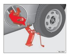
Fig. 137 Fitting the jack
