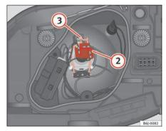
Fig. 152 Dipped beam / main beam, single light
