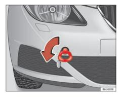
Fig. 164 Fitting the towing eye to the rear of the vehicle
