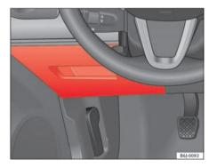
Fig. 140 Fuses in the dash panel
