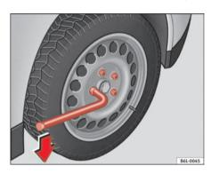
Fig. 135 Changing the wheel: loosen the wheel holts
