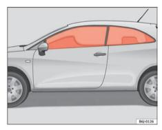
Fig. 22 Deployed curtain airbags
