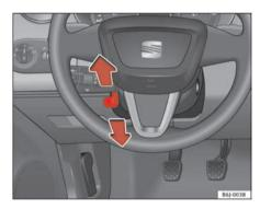
Fig. 91 Steering column height adjustment
