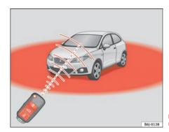
Fig. 43 Range of the remote control:
