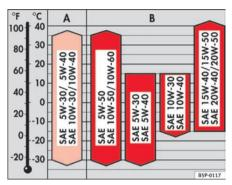
Fig. 124 Types of oil according to temperature
