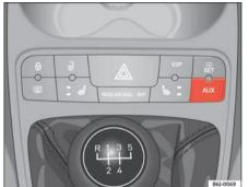
Fig. 82 AUX connection on the central console (depending on the equipment)
