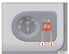
Fig. 51 Instrument panel: regulation for instrument and switch illumination and headlight range control
