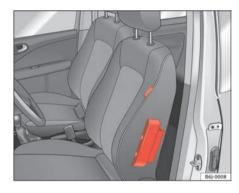
Fig. 19 Side airbag in driver seat
