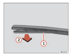
Fig. 130 Changing the rear window wiper blade
