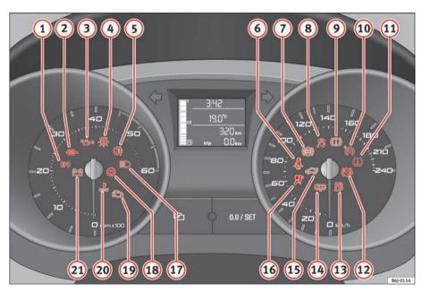
Fig. 36 Instrument panel with warning lamps. Some of the items of equipment listed here are fitted only on certain models/model years or are optional extras.
