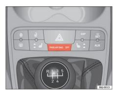
Fig. 24 Warning lamp for deactivated passenger airbag in centre console
