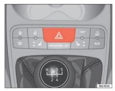
Fig. 54 Centre console: switch for hazard warning lights
