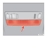
Fig. 147 Front reading light
