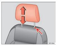
Fig. 66 Adjusting and removing the head restraints
