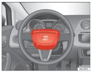
Fig. 16 Driver airbag located in steering wheel
