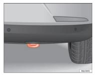
Fig. 152 Rear towing ring
