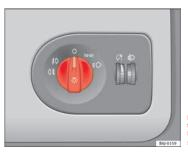
Fig. 49 Detailed view of the dash panel: lights, fog lights and rear fog light switch
