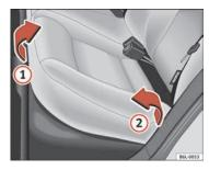
Fig. 69 Folding up the rear seat cushion
