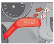
Fig. 61 Windscreen wiper and windscreen wash lever: rear window wiper
