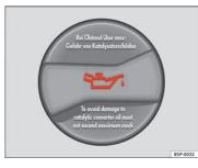
Fig. 114 In the engine compartment: Engine oil filler cap
