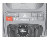
Fig. 53 Centre console: heated rear window switch
