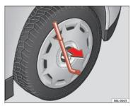
Fig. 122 Remove the complete hub cap
