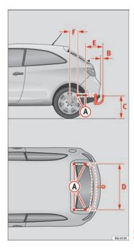
Fig. 108 Attachment points for towing bracket
