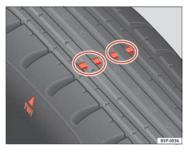
Fig. 120 Tyre tread wear indicators
