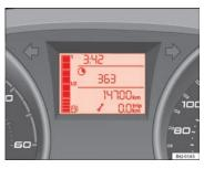
Fig. 34 Service interval display
