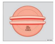
Fig. 115 In the engine compartment: Coolant expansion tank cap
