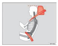
Fig. 4 Properly adjusted head restraint viewed from the side
