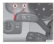
Fig. 105 Turn signal and main beam headlight lever: switch and rocker switch for the cruise
