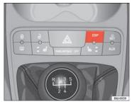
Fig. 92 Detailed view of the centre console: ESP button
