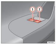
Fig. 46 Detail of the driver door: controls for the front windows.
