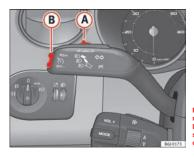
Fig. 104 Turn signal and main beam headlight lever: switch and rocker switch for the cruise control
