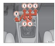
Fig. 94 Centre Console: gear shift pattern of a 5speed manual gearbox
