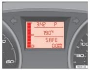
Fig. 101 Automatic gearbox: Instrument panel display
