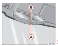
Fig. 62 Automatic antidazzle interior mirror.
