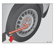
Fig. 123 Changing the wheel: loosen the wheel holts
