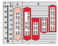
Fig. 112 Types of oil according to temperature
