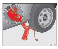
Fig. 125 Fitting the jack
