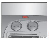
Fig. 73 Mounting bracket for navigator on dash panel.
