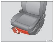
Fig. 75 Storage compartment under the front passenger seat
