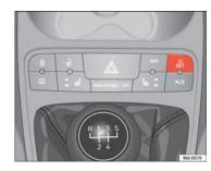
Fig. 36 Centre console: tyre monitor system
