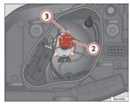
Fig. 139 Dipped beam/main beam, single headlight
