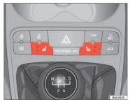
Fig. 68 Front seats heating switch
