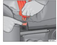
Fig. 15 Removing latch plate from buckle
