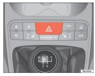
Fig. 54 Centre console: switch for hazard warning
