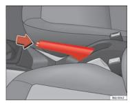
Fig. 102 Handbrake between the front seats
