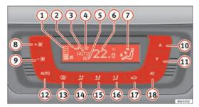
Fig. 90 Climatronic controls on the dash panel
