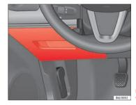
Fig. 128 Fuses in the dash panel
