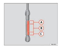
Fig. 113 Engine oil dipstick
