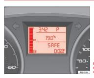
Fig. 33 Digital display: Gear lever position for automatic gearbox.
