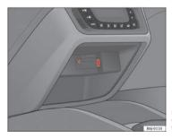
Fig. 83 AUX/USB\* input connection (depending on the equipment)
