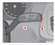
Fig. 31 Windscreen wiper lever: button A and rocker switch B
