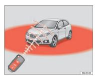
Fig. 42 Range of the remote control
