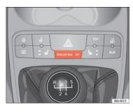
Fig. 22 Warning lamp for deactivated passenger airbag in centre console
