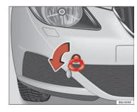
Fig. 151 Fitting the towing eye to front rear of the vehicle
