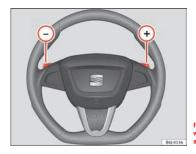
Fig. 100 Steering wheel with paddle levers for automatic gearbox
