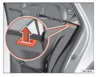
Fig. 70 Button for unlocking the rear backrest
