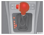
Fig. 99 Changing gear with tiptronic
