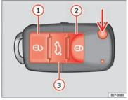
Fig. 41 Assignment of buttons on the remote control key
