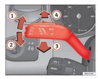
Fig. 55 Turn signal and main beam headlight
