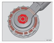
Fig. 119 In the engine compartment: Brake fluid reservoir cover
