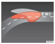
Fig. 52 Cornering lighting using adaptive headlights
