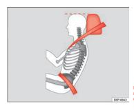
Fig. 65 Side view: head restraints and seat belts correctly adjusted
