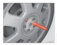
Fig. 126 Changing the wheel: Hexagonal socket in screwdriver handle to turn the wheel bolts
