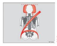
Fig. 12 Correct seat belt and head restraint positions, viewed from front
