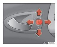
Fig. 63 Controls of exterior mirrors
