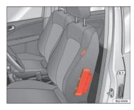
Fig. 19 Side airbag in driver seat
