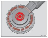
Fig. 129 In the engine compartment: Brake fluid reservoir cover
