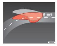
Fig. 56 Cornering lighting using adaptive headlights
