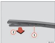
Fig. 128 Changing the rear window wiper blade
