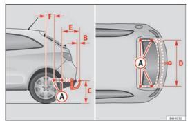
Fig. 116 Attachment points for towing bracket
