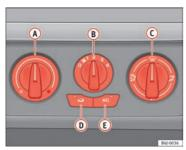
Fig. 92 Air conditioning controls on the dash panel
