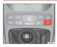
Fig. 86 AUX connection on the central console (depending on the equip-
