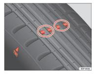
Fig. 130 Tyre tread wear indicators
