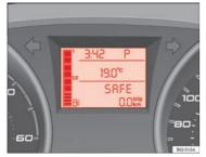
Fig. 104 Automatic gearbox: Instrument panel display
