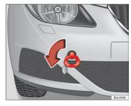
Fig. 161 Fitting the towing eye to front rear of
