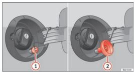
Fig. 118 Fuel tank open with LPG filler neck and adapter.
