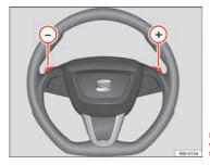
Fig. 107 Steering wheel with paddle levers for automatic gearbox
