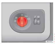
Fig. 53 Detailed view of the dash panel: lights, fog lights and rear fog light switch
