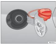
Fig. 117 Tank flap open
