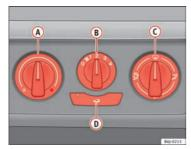
Fig. 89 Heating controls on the dash panel
