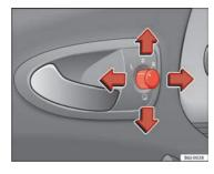
Fig. 67 Controls of exterior mirrors
