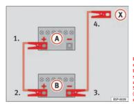
Fig. 159 Diagram for connecting jump leads if the vehicle providing assistance the current is not fitted with the Start-Stop system: flat battery (A) and battery providing current (B).
