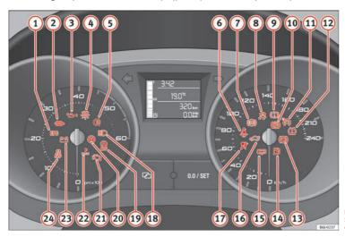
Fig. 38 Instrument panel warning and indicator lamps. Some of the items of equipment listed here are fitted only on certain model versions or are optional extras.
