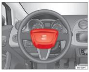
Fig. 16 Driver airbag located in steering wheel
