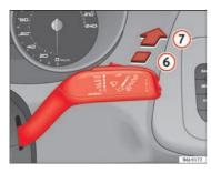
Fig. 65 Windscreen wiper and windscreen wash lever: rear window wiper
