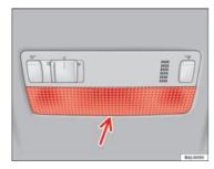
Fig. 156 Front reading light
