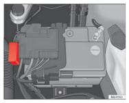
Fig. 138 Fuses in engine compartment
