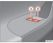
Fig. 50 Detail of the driver door: controls for the front windows.
