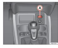
Fig. 98 Centre console: gas system control
