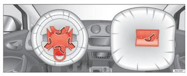
Fig. 19 Airbag covers reacting when the front airbags are triggered
