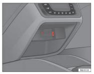
Fig. 87 AUX/USB\* input connection (depending on the equipment)
