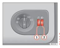
Fig. 55 Dash panel: regulation for instrument and switch illumination and headlight range control
