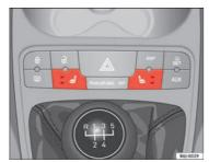
Fig. 72 Front seats heating switch
