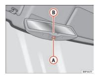
Fig. 66 Automatic antidazzle interior mirror.
