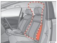
Fig. 20 Side airbag in driver seat
