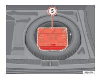
Fig. 165 For vehicles with the battery in the luggage compartment.
