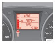
Fig. 31 Instrument panel: gas gauge.
