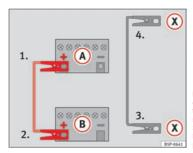
Fig. 160 Diagram for connecting jump leads if the vehicle providing assistance is fitted with the Start-Stop system: flat battery (A) and battery providing current (B).
