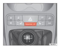
Fig. 22 Warning lamp for deactivated passenger airbag in centre console
