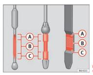
Fig. 123 Engine oil dipstick
