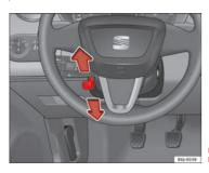
Fig. 95 Steering column height adjustment
