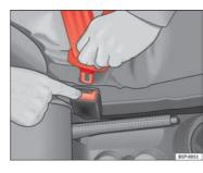
Fig. 15 Removing latch plate from buckle
