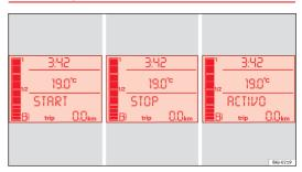
Fig. 100 Display on the instrument panel during Start-Stop function operation.
