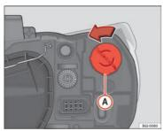
Fig. 146 Single turn signal lamp
