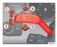
Fig. 59 Turn signal and main beam headlight lever
