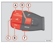
Fig. 42 Audio + Telephone Control
