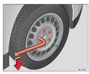
Fig. 133 Changing the wheel: loosen the wheel bolts
