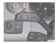
Fig. 110 Turn signal and main beam headlight lever: switch and rocker switch for the cruise con-
