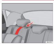
Fig. 28 Retainer strap: correct adjustment and fitting
