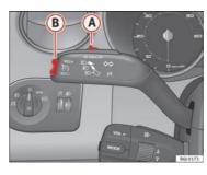
Fig. 112 Turn signal and main beam headlight lever: switch and rocker switch for the cruise control
