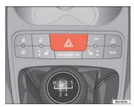
Fig. 58 Centre console: switch for hazard warning lights
