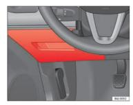
Fig. 137 Fuses in the dash panel
