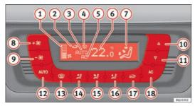
Fig. 94 Climatronic controls on the dash panel
