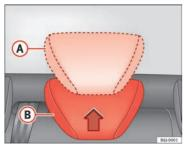
Fig. 5 Adjusting the rear head restraints
