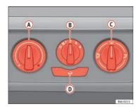
Fig. 90 Heating controls on the dash panel
