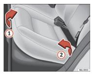
Fig. 73 Folding up the rear seat cushion
