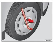
Fig. 132 Remove the complete hub cap
