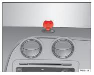
Fig. 78 Bracket with open cover for placing the navigator.
