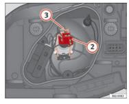
Fig. 148 Dipped beam/ main beam, single headlight
