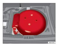
Fig. 119 LPG tank spare wheel well
