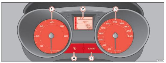
Fig. 30 Detailed view of the dash panel: instrument panel
