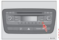
Fig. 87 AUX connection on the central console (depending on the equipment)
