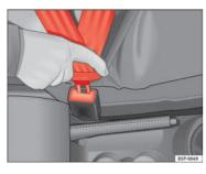
Fig. 11 Belt buckle and latch plate of seat belt
