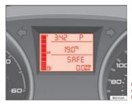
Fig. 109 Automatic gearbox: Instrument panel display
