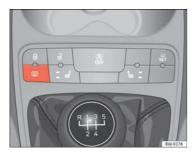
Fig. 57 Centre console: heated rear window switch
