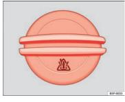
Fig. 128 In the engine compartment: Coolant expansion tank cap
