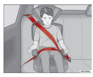
Fig. 25 Forward-facing child seat installed on rear seat
