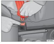
Fig. 15 Remove latch plate from buckle
