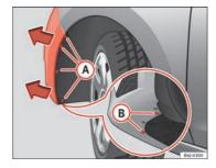
Fig. 162 Fog light: access to the connector and to the light bulb holder
