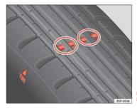
Fig. 135 Tyre tread wear indicators
