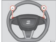
Fig. 108 Steering wheel with paddle levers for automatic gearbox
