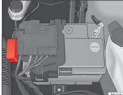
Fig. 143 In the engine compartment: fuse box cover
