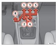
Fig. 102 Centre Console: gear shift pattern of a 5speed manual gearbox
