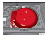
Fig. 122 LPG tank in spare wheel well
