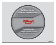
Fig. 127 In the engine compartment: Engine oil filler cap
