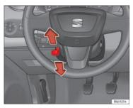
Fig. 96 Steering column height adjustment
