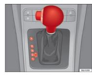
Fig. 107 Changing gear with tiptronic
