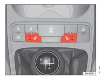
Fig. 72 Front seats heating switch
