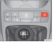
Fig. 40 Centre console: tyre monitor system button
