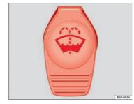
Fig. 129 In the engine compartment: Cap of windscreen washer fluid reservoir
