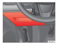
Fig. 142 Left side of dash panel fuse box cover
