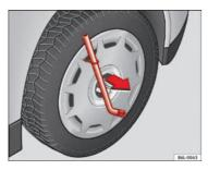
Fig. 137 Remove the complete hub cap
