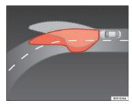
Fig. 56 Cornering lighting using adaptive headlights
