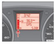
Fig. 31 Instrument panel: gas gauge.
