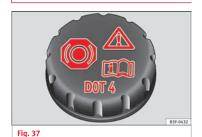
The brake fluid reservoir is located in the engine compartment **»** page 168.
