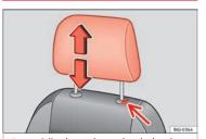
Fig. 99 Adjusting and removing the head restraints.
