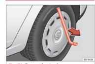
Fig. 158 Remove the wheel cover.
