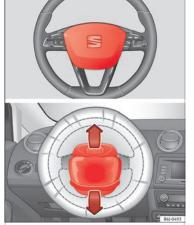
Fig. 17 Driver airbag located in steering wheel.
