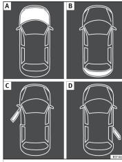
Fig. 40 A: bonnet open; B: rear lid open; C: front left door open; D: rear right door open (5-door vehicles only).
