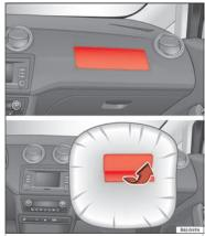
**Fig. 18** Front passenger airbag located in dash panel.
