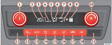
Fig. 167 Climatronic: controls.
