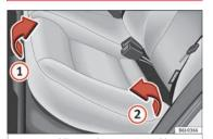
Fig. 143 Folding up the rear seat cushion.
