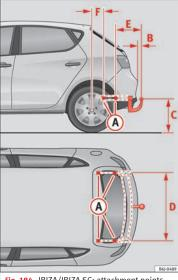
**Fig. 184** IBIZA/IBIZA SC: attachment points for towing bracket.
