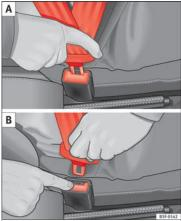
Fig. 13 Positioning and removing the seat belt buckle.
