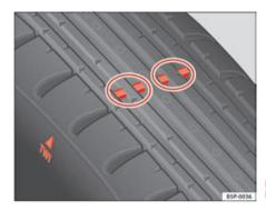
Fig. 135 Tyre tread wear indicators
