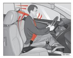
Fig. 11 Driver wearing the seat belt correctly: is restrained by the belt when braking sharply
