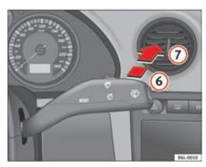
Fig. 68 Windscreen wiper and windscreen wash lever: rear window wiper
