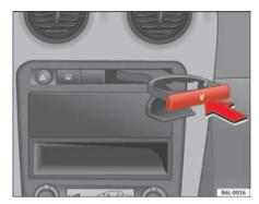
Fig. 83 Front cup holder in the centre console
