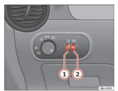
Fig. 58 Instrument panel: regulators for instrument and control illumination and headlight range control
