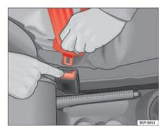
Fig. 16 Removing latch plate from buckle
