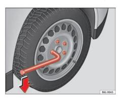
Fig. 142 Changing the wheel: loosen the wheel bolts
