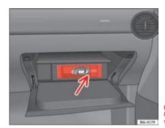
Fig. 89 USB connection\* in glove box on passenger side
