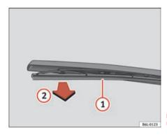
Fig. 133 Changing the rear window wiper blade
