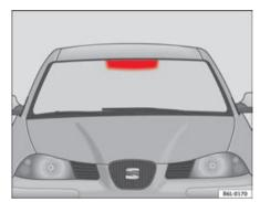
Fig. 69 Location of the electronic pricing device
