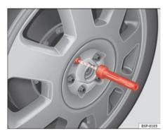
Fig. 145 Changing the wheel: hexagonal socket in screwdriver handle to turn the wheel bolts after they have been loosened
