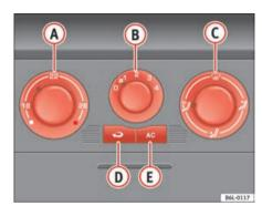
Fig. 95 On the instrument panel: air conditioner controls
