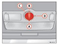
Fig. 54 Detail of the roof lining: rotary control for sliding sun roof/ deflector
