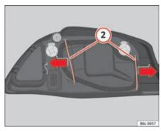
Fig. 151 Dipped headlight lamp
