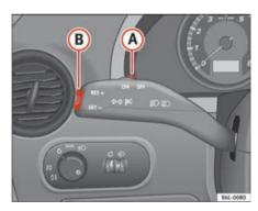
Fig. 110 Turn signal and main beam headlight lever switch and rocker switch for the cruise control
