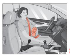
Fig. 15 Positioning seat belts during pregnancy
