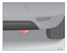
Fig. 176 Rear towing ring
