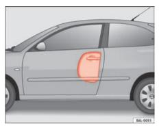
Fig. 22 Inflated side airbag on left side of vehicle
