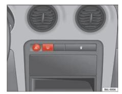
Fig. 59 Instrument panel: heated rear window switch
