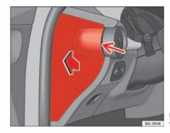
Fig. 147 Fuses in the dash panel
