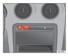
Fig. 60 Instrument panel: switch for hazard warning
