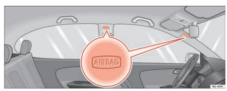
Fig. 23 Location of left curtain airbag
