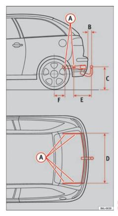
Fig. 124 Attachment points for towing bracket
