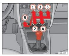
Fig. 101 Centre Console: gear shift pattern of a 5-speed manual gearbox
