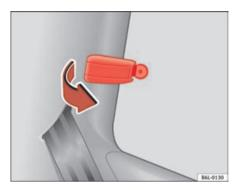
Fig. 53 Release lever for mechanical vent wing
