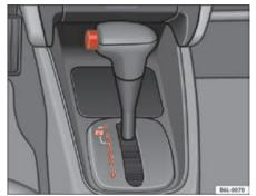
Fig. 102 Centre console: Automatic gearbox selector lever
