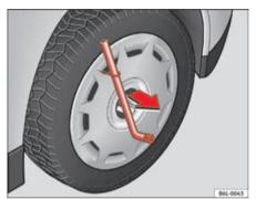
Fig. 141 Remove the complete hub cap
