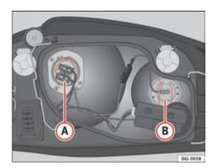
Fig. 152 Dipped headlight lamp
