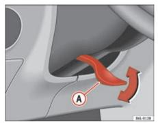
Fig. 97 Adjusting the steering wheel position
