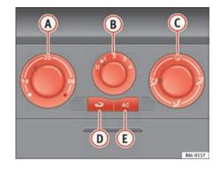
Fig. 94 On the instrument panel: air conditioner controls
