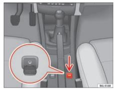
Fig. 87 Auxiliary audio connection
