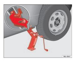
Fig. 144 Fitting the jack
