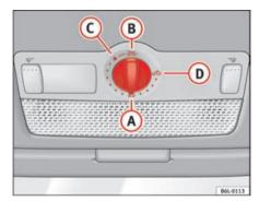
Fig. 55 Detail of the roof lining: rotary control for sliding sun roof/ deflector
