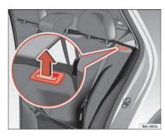
Fig. 78 Button for unlocking the rear back-rest
