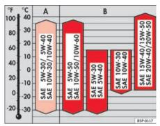
Fig. 127 Types of oil according to temperature
