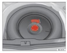
Fig. 139 Securing the defective wheel in the spare wheel well
