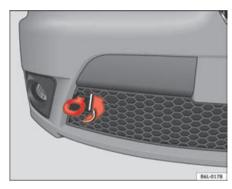
Fig. 175 Towing eye at the front of the vehicle
