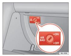
Fig. 25 In the glove compartment: switch for enabling and disabling front passenger airbag
