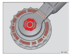
Fig. 134 In the engine compartment: Brake fluid reservoir cover
