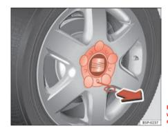
Fig. 140 Changing the wheel: Removing a hub
