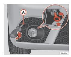
Fig. 172 Towing eye at the front of the vehicle
