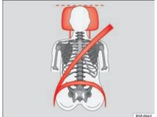
Fig. 72 Front view: head restraints and seat belts correctly adjusted
