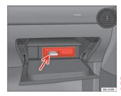
Fig. 88 iPod connection in glove box on passenger
