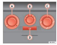
Fig. 91 On the dash panel: Heater controls
