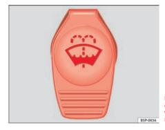
Fig. 131 In the engine compartment: Cap of windscreen washer fluid reservoir.
