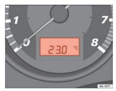
Fig. 38 Digital instrument panel display: outside temperature display.
