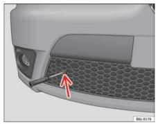
Fig. 173 Eye cover on the central lower grille
