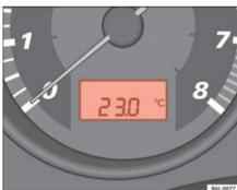
Fig. 36 Digital instrument panel display: Outside temperature display
