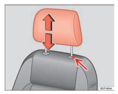
Fig. 74 Adjusting and removing the head restraints
