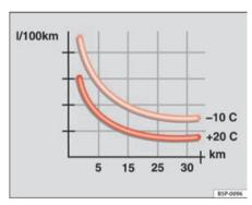
Fig. 123 Fuel consumption in litres per 100 km at two different ambient temperatures
