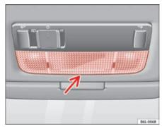
Fig. 168 Front reading light
