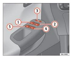
Fig. 52 Detail of driver door: controls for the front and rear windows
