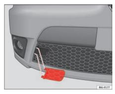
Fig. 174 Eye cover on the central lower grille
