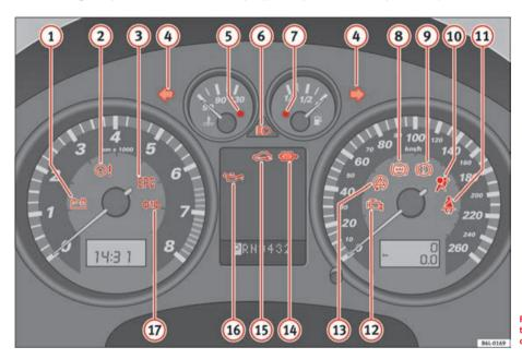
Fig. 40 Instrument panel with warning lamps. Some of the items of equipment listed here are fitted only on certain models/model years or are optional extras.
