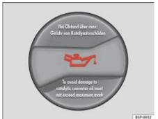
Fig. 129 In the engine compartment: Engine oil filler cap
