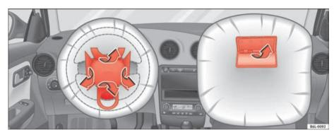
Fig. 20 Airbag covers reacting when the airbags are triggered
