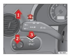
Fig. 61 Turn signal and main beam headlight
