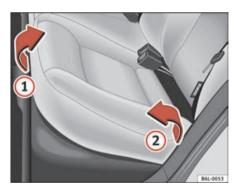
Fig. 77 Folding up the rear seat cushion
