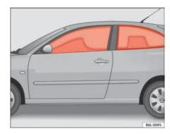
Fig. 24 Deployed curtain airbags
