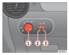
Fig. 57 Detail of the instrument panel: light controls, fog light and rear fog light control
