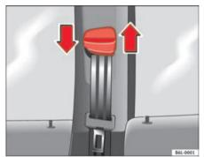
Fig. 6 Location of the belt height adjuster
