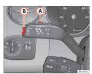
Fig. 107 Turn signal and main beam headlight lever: switch and rocker switch for the cruise control
