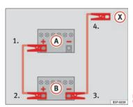
Fig. 150 How to connect the jump leads
