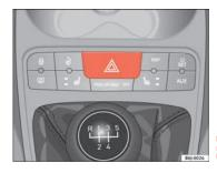
Fig. 55 Centre console: switch for hazard warning
