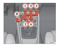
Fig. 95 Centre Console: gear shift pattern of a 5speed manual gearbox
