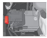
Fig. 131 Fuses in engine compartment
