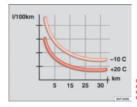
Fig. 109 Fuel consumption in litres per 100 km at two different ambient temperatures
