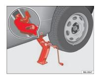
Fig. 127 Fitting the jack
