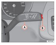
Fig. 32 Windscreen wiper and windscreen wash lever: button A and rocker switch B
