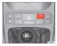
Fig. 93 Detailed view of the centre console: ESP button.
