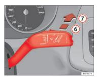
Fig. 62 Windscreen wiper and windscreen wash lever: rear window wiper
