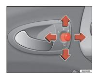
Fig. 64 Controls of exterior mirrors
