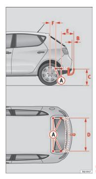
Fig. 110 Attachment points for towing bracket
