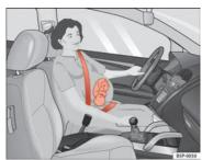
Fig. 14 Positioning seat belts during pregnancy
