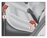
Fig. 70 Folding up the rear seat cushion
