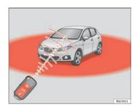
Fig. 43 Range of the remote control
