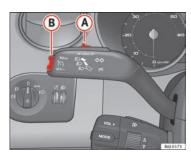
Fig. 106 Turn signal and main beam headlight lever: switch and rocker switch for the cruise control
