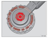
Fig. 121 In the engine compartment: Brake fluid reservoir cover
