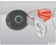
Fig. 111 Tank flap open
