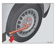
Fig. 125 Changing the wheel: loosen the wheel holts
