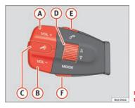
Fig. 38 Audio + Telephone Control
