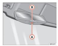
Fig. 63 Automatic antidazzle interior mirror.
