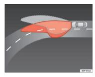
Fig. 53 Cornering lighting using adaptive headlights
