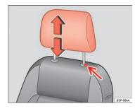
Fig. 67 Adjusting and removing the head restraints
