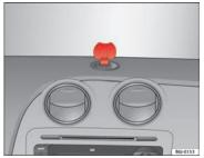
Fig. 75 Bracket with open cover for placing the navigator.
