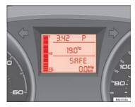
Fig. 102 Automatic gearbox: Instrument panel display
