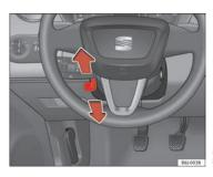
Fig. 92 Steering column height adjustment
