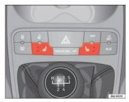
Fig. 69 Front seats heating switch
