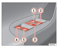
Fig. 47 Detail of the driver door: controls for the front and rear windows
