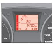
Fig. 34 Service interval display
