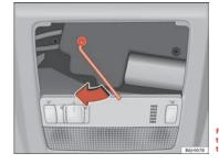
Fig. 49 Emergency operation of the panorama/ tilting roof
