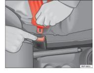
Fig. 15 Removing latch plate from buckle
