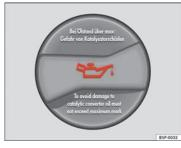
Fig. 116 In the engine compartment: Engine oil filler cap
