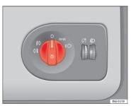
Fig. 50 Detailed view of the dash panel: lights, fog lights and rear fog light switch
