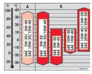
Fig. 114 Types of oil according to temperature
