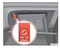
Fig. 21 In the glove compartment: key for enabling and disabling front passenger airbag
