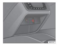
Fig. 84 AUX/USB\* input connection (depending on the equipment)
