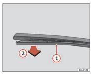
Fig. 120 Changing the rear window wiper blade
