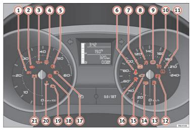
Fig. 35 Instrument panel control and warning lamps. Some of the items of equipment listed here are fitted only on certain model versions or are optional extras.
