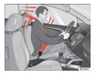
Fig. 10 A driver wearing the seat belt properly: is secured by the belt in sharp braking
