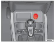
Fig. 82 Front power socket
