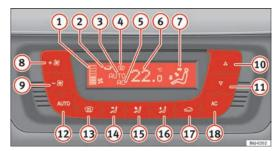
Fig. 91 Climatronic controls on the dash panel
