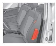
Fig. 19 Side airbag in driver seat
