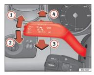
Fig. 56 Turn signal and main beam headlight lever
