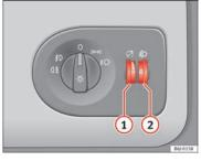
Fig. 52 Dash panel: regulation for instrument and switch illumination and headlight range control
