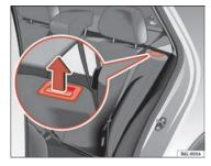
Fig. 71 Button for unlocking the rear back-rest
