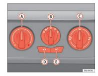
Fig. 89 Air conditioning controls on the dash panel
