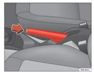
Fig. 103 Handbrake between the front seats
