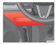
Fig. 130 Fuses in the dash panel
