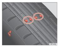
Fig. 122 Tyre tread wear indicators
