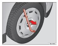
Fig. 124 Remove the complete hub cap
