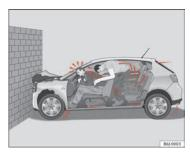
Fig. 7 The vehicle hits the wall: the occupants are not wearing seat belts
