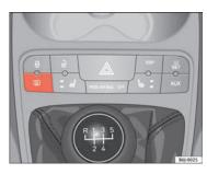
Fig. 54 Centre console: heated rear window switch
