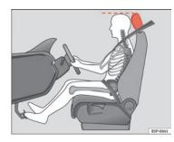
Fig. 2 Proper head restraint position for driver
