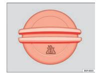
Fig. 117 In the engine compartment: Coolant expansion tank cap
