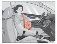
Fig. 14 Positioning seat belts during pregnancy
