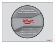
Fig. 125 In the engine compartment: Engine oil filler cap
