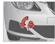
Fig. 160 Fitting the towing eye to front rear of
