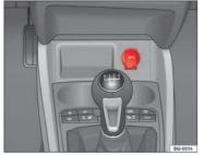
Fig. 86 Front power socket
