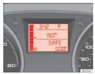
Fig. 36 Digital display: Gear lever position for automatic gearbox.
