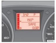
Fig. 105 Automatic gearbox: Instrument panel display
