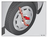
Fig. 133 Remove the complete hub cap
