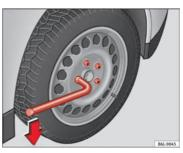
Fig. 134 Changing the wheel: loosen the wheel holts
