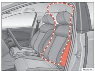
Fig. 20 Side airbag in driver seat
