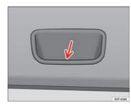
Fig. 49 Detail of the inside of the tailgate: hand grip
