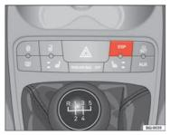
Fig. 97 Detailed view of the centre console: ESP button.
