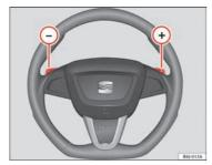
Fig. 108 Steering wheel with paddle levers for automatic gearbox
