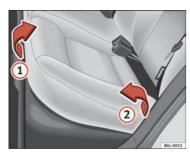
Fig. 74 Folding up the rear seat cushion
