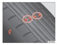
Fig. 131 Tyre tread wear indicators
