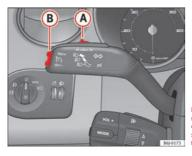
Fig. 112 Turn signal and main beam headlight lever: switch and rocker switch for the cruise control
