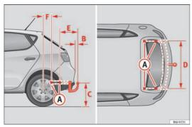
Fig. 117 Attachment points for towing bracket
