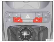
Fig. 73 Front seats heating switch
