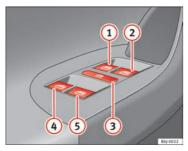
Fig. 51 Detail of the driver door: controls for the front and rear windows
