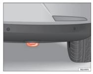
Fig. 161 Rear towing ring
