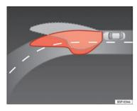
Fig. 57 Cornering lighting using adaptive headlights
