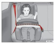
Fig. 24 A category 1 forward-facing child seat fitted on the rear seat.
