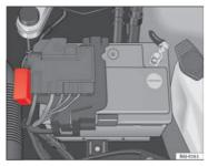
Fig. 139 Fuses in engine compartment
