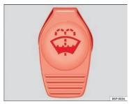
Fig. 127 In the engine compartment: Cap of windscreen washer fluid reservoir.
