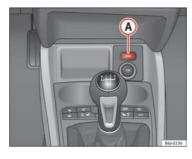
Fig. 99 Centre console: gas system control switch.
