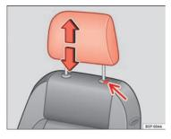
Fig. 71 Adjusting and removing the head restraints
