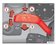
Fig. 60 Turn signal and main beam headlight lever
