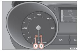
Fig. 39 Instrument panel indicator and warning lamps in vehicles with LPG.
