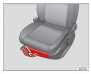
Fig. 80 Storage compartment under the front passenger seat
