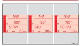
Fig. 101 Display on the instrument panel during Start-Stop function operation.
