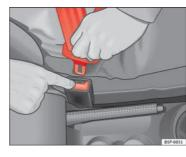
Fig. 15 Removing latch plate from buckle
