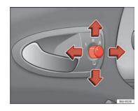
Fig. 68 Controls of exterior mirrors
