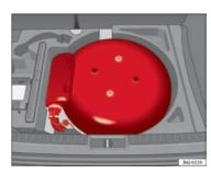
Fig. 120 LPG tank in spare wheel well
