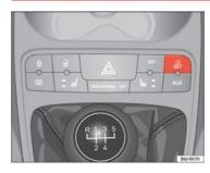
Fig. 40 Centre console: tyre monitor system but-
