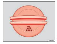
Fig. 126 In the engine compartment: Coolant expansion tank cap
