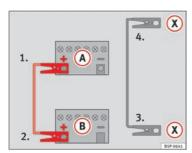
Fig. 159 Diagram for connecting jump leads if the vehicle providing assistance is fitted with the Start-Stop system: flat battery (a) and battery providing current (a).
