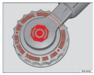
Fig. 130 In the engine compartment: Brake fluid reservoir cover
