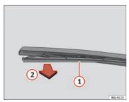
Fig. 129 Changing the rear window wiper blade
