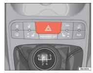
Fig. 59 Centre console: switch for hazard warning lights
