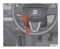
Fig. 96 Steering column height adjustment
