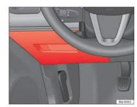
Fig. 138 Fuses in the dash panel
