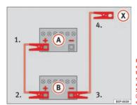
Fig. 158 Diagram for connecting jump leads if the vehicle providing assistance the current is not fitted with the Start-Stop system: flat battery (A) and battery providing current (B).
