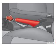
Fig. 110 Handbrake between the front seats
