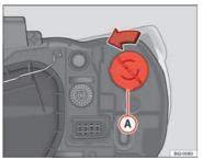
Fig. 147 Single turn signal lamp
