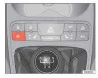
Fig. 58 Centre console: heated rear window switch
