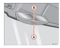
Fig. 67 Automatic antidazzle interior mirror.
