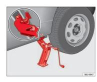
Fig. 136 Fitting the jack
