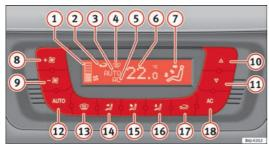
Fig. 95 Climatronic controls on the dash panel
