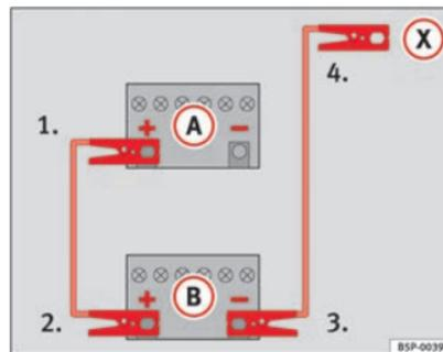
Fig. 168 Diagram for connecting jump leads if the vehicle providing assistance is not fitted with the Start-Stop system: flat battery (A) and battery providing current (B).
