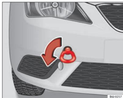
Fig. 170 Fitting the towing eye to front rear of the vehicle
