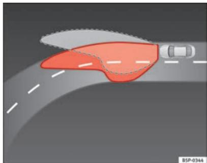
Fig. 57 Cornering lighting using adaptive headlights
