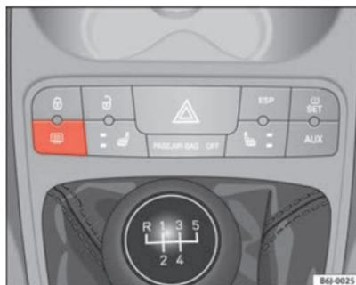
**Fig. 58 Centre console: heated rear window switch**
