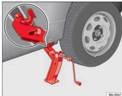
**Fig. 139** Fitting the jack
