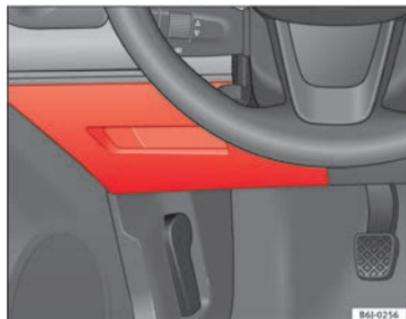
Fig. 141 Fuses in the dash panel
