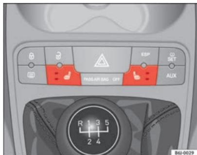
**Fig. 73** Front seats heating switch
