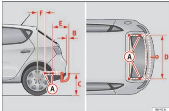
Fig. 118 Attachment points for towing bracket
