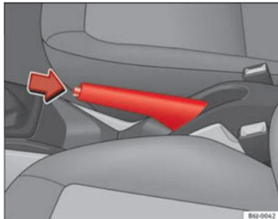
**Fig. 111 Handbrake between the front seats**
