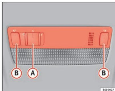
Fig. 62 Front reading light
