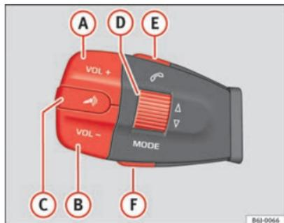
Fig. 42 Audio + Telephone Control
