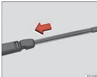
Fig. 132 Fitting the rear window wiper blade ▶
