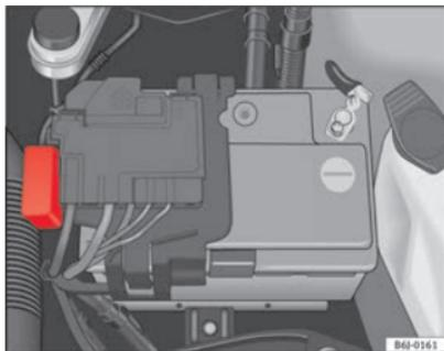
Fig. 142 Fuses in engine compartment
