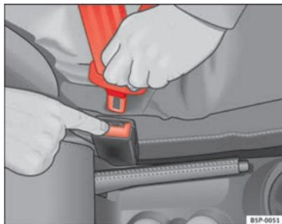
Fig. 15 Removing latch plate from buckle
