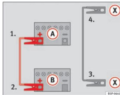
Fig. 169 Diagram for connecting jump leads if the vehicle providing assistance is fitted with the Start-Stop system: flat battery (A) and battery providing current (B).
