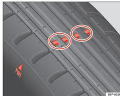
Fig. 134 Tyre tread wear indicators
