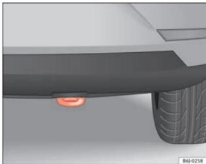
Fig. 171 Rear towing ring
