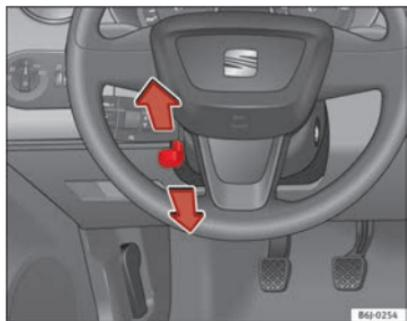
**Fig. 97** Steering column height adjustment
