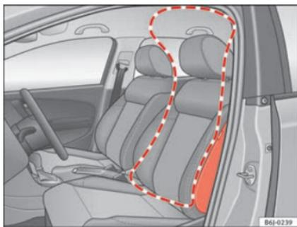
**Fig. 20 Side airbag in driver seat**
