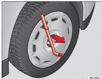
Fig. 136 Remove the complete hub cap
