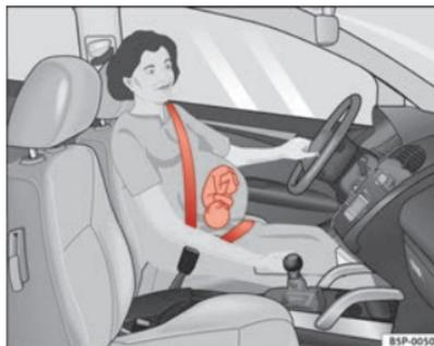
Fig. 14 Positioning seat belts during pregnancy ▶
