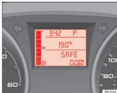
Fig. 106 Automatic gearbox: Instrument panel display
