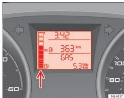
Fig. 31 Instrument panel: gas gauge.
