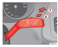
Fig. 66 Windscreen wiper and windscreen wash lever: rear window wiper
