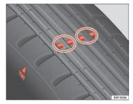
Fig. 136 Tyre tread wear indicators
