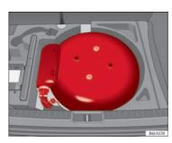
Fig. 123 LPG tank in spare wheel well
