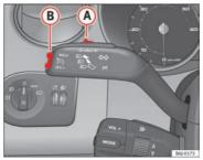
Fig. 118 Turn signal and main beam headlight lever: switch and rocker switch for the cruise con-
