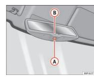
Fig. 67 Automatic antidazzle interior rear vision mirror.
