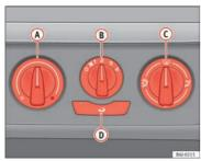
Fig. 91 Heating controls on the dash panel
