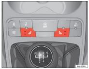
Fig. 73 Front seats heating switch
