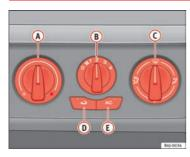
Fig. 95 Air conditioning controls on the dash panel
