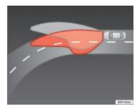
Fig. 57 Cornering lighting using adaptive headlights
