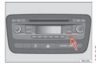
Fig. 88 AUX connection in the centre console (depending on the equipment)
