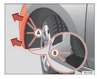
Fig. 163 Fog light: access to the connector and to the light bulb holder
