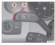
Fig. 116 Turn signal and main beam headlight lever: switch and rocker switch for the cruise control
