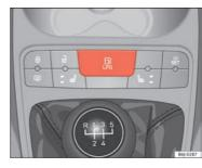
Fig. 100 Centre console: gas system control switch.
