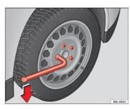
Fig. 139 Changing a wheel: loosen the wheel bolts
