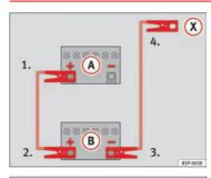
Fig. 172 Diagram of connections for vehicles without Start Stop system
