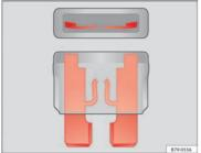
Fig. 145 Image of a blown fuse
