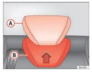
Fig. 5 Adjusting the rear head restraints
