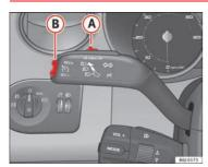
Fig. 117 Turn signal and main beam headlight lever: switch and rocker switch for the cruise control
