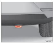
Fig. 175 Rear towline anchorage
