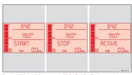
Fig. 102 Display on the instrument panel during Start-Stop function operation.
