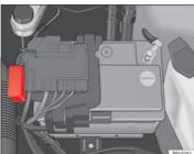
Fig. 144 In the engine compartment: fuse box cover
