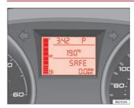
Fig. 36 Digital display: Gearbox lever position for automatic gearbox.
