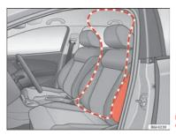
Fig. 20 Side airbag in driver seat
