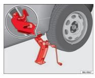
Fig. 141 Fitting the jack
