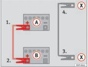
Fig. 173 Diagram of connections for vehicles with Start Stop system
