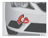
Fig. 174 Fitting the towline anchorage to front of the vehicle
