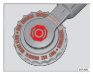
Fig. 135 In the engine compartment: Brake fluid reservoir cover
