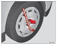
Fig. 138 Remove the complete hub cap
