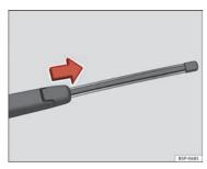
Fig. 133 Removing the rear window wiper blade
