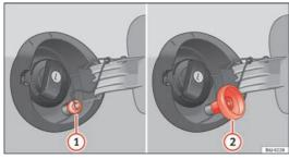
Fig. 122 Fuel tank open with LPG filler neck and adapter
