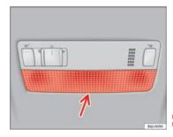
Fig. 169 Front reading light
