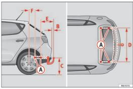
Fig. 120 Attachment points for towing bracket
