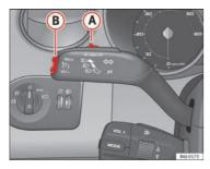
Fig. 115 Turn signal and main beam headlight lever: switch and rocker switch for the cruise control
