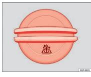
Fig. 129 In the engine compartment: Coolant expansion tank cap
