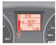
Fig. 31 Instrument panel: gas gauge.
