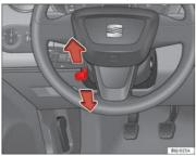
Fig. 97 Steering column height adjustment
