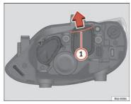
Fig. 156 Dipped beam headlights
