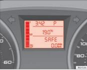
Fig. 106 Automatic gearbox: Instrument panel display
