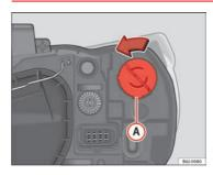
Fig. 147 Single turn signal lamp
