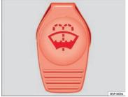
Fig. 130 In the engine compartment: Cap of windscreen washer fluid reservoir
