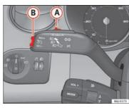
Fig. 114 Turn signal and main beam headlight lever: switch and rocker switch for the cruise con-
