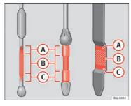
Fig. 127 Engine oil dipstick
