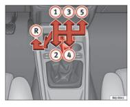
Fig. 103 Centre Console: gear shift pattern of a 5speed manual gearbox
