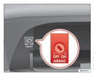
Fig. 21 In the glove compartment: switch for activating and deactivating the front passenger airbag
