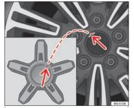
Fig. 80 Fitting the central wheel trim.
