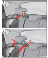
Fig. 37 Retainer strap: adjustment and assembly according to the Top Tether belt.
