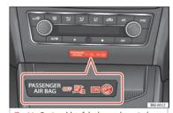
Fig. 24 Centre side of dash panel: control lamp for deactivated front passenger airbag in centre console.
