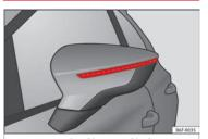
Fig. 120 Turn signal integrated in the rear view mirror
