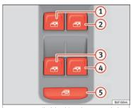
Fig. 146 Detail of the driver door: controls for the front and rear windows (vehicles with front and rear electric windows).
