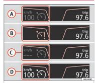
Fig. 187 Instrument panel display: CCS status indications.
