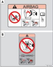
Fig. 29 Airbag stickers - version 1: on the passenger-side sun blind (A) and on the rear frame of the front passenger's door (B).
