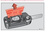
Fig. 138 Vehicle key: opening the battery compartment.
