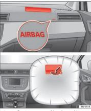
Fig. 22 Front passenger airbag located in dash panel.
