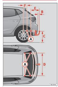
Fig. 226 Attachment points for towing bracket.
