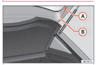
Fig. 167 In the luggage compartment: removing and installing the rear shelf.
