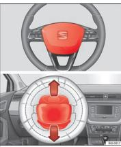
Fig. 21 Driver airbag located in steering wheel.
