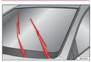
Fig. 91 Wipers in service position.
