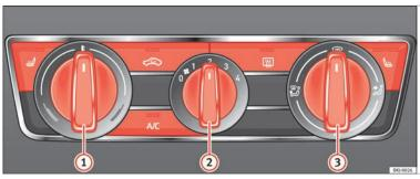
Fig. 63 In the centre console: Manual air conditioning controls.
