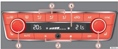
Fig. 62 In the centre console: Climatronic controls
