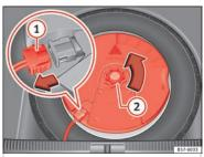
**Fig. 235** In the luggage compartment: remove the subwoofer.
