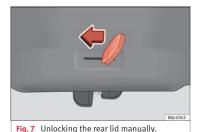
This allows the vehicle to be opened if the central locking does not work (for example, if the battery is flat).
