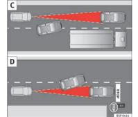
Fig. 202 (C) Vehicle changing lanes. (D) One vehicle turning and another stationary.
