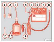
Fig. 107 Standard representation: contents of the anti-puncture kit.
