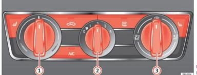
**Fig. 175** Air conditioning controls on the dash panel.
