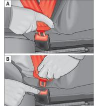
Fig. 103 Positioning and removing the seat belt buckle
