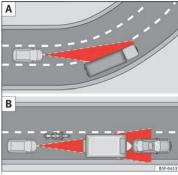
Fig. 201 (A) Vehicle on a bend. (B) Motorcyclist ahead out of range of the radar sensor.
