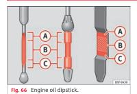
The level is measured using the dipstick located in the engine compartment
