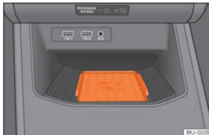
**Fig. 215** Consola central: Connectivity Box
