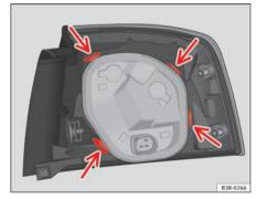
Fig. 223 Securing the bulb holder in the rear light unit
