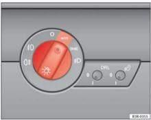
Fig. 86 Detailed view of instrument panel: Light switch
