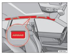
Fig. 25 Location of left curtain airbag
