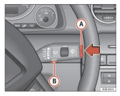
Fig. 58 Windscreen wiper lever: Function selector switch
