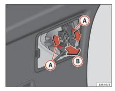
Fig. 228 Remove the bulb holder
