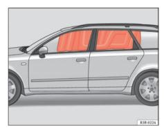
Fig. 26 Deployed curtain airbags
