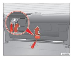
Fig. 76 Detail of the tailgate: emergency unlocking mechanism
