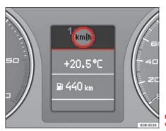
Fig. 56 Display: Speed warning function
