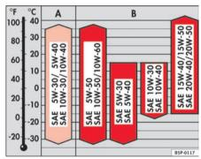
Fig. 172 Types of oil according to temperature
