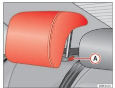
Fig. 5 Outer rear seats: Head restraints
