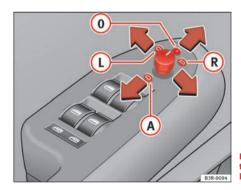
Fig. 105 Detailed view of the armrest: Adjuster knob
