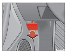
Fig. 170 Detail of footwell area on driver's side: lever for unlocking the bonnet.
