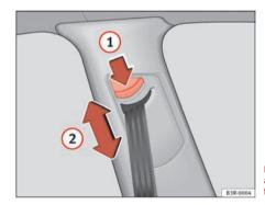
Fig. 16 Belt height adjustment - top guide fitting
