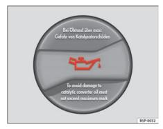
Fig. 174 In the engine compartment: Engine oil filler cap
