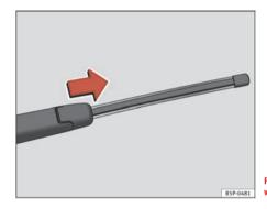
Fig. 179 Remove rear window wiper blade
