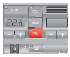
Fig. 142 Button for automatic air recirculation
