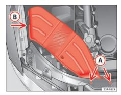
Fig. 210 Air duct on right side of vehicle
