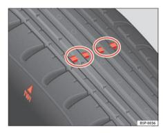
Fig. 183 Tyre tread wear indicators
