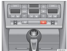
Fig. 98 Switch for heated rear window
