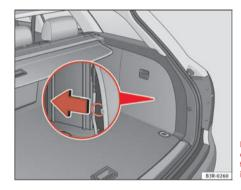
Fig. 169 Luggage compartment: Releasing the fuel tank flap by hand in case of emergency
