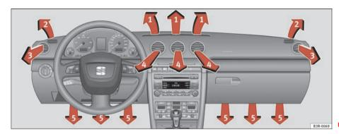
Fig. 143 Instrument panel: Location of air outlets
