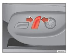
Fig. 109 Front seat: Backrest adjuster switch
