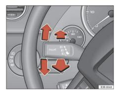
Fig. 93 Turn signal and main beam headlight
