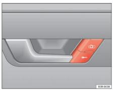
Fig. 71 Detail of driver door: Central locking switch
