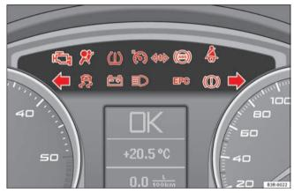
Fig. 44 Instrument panel with warning and indicator lamps
