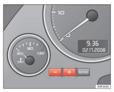
Fig. 88 Instrument panel lighting
