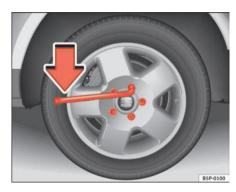
Fig. 189 Changing the wheel: Loosen the wheel belts
