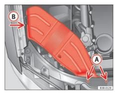
Fig. 211 Air duct on right side of vehicle
