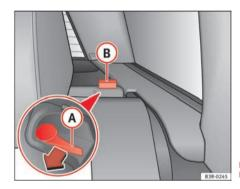
Fig. 127 Backrest release lever
