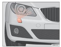
Fig. 103 Headlight with extended washer jet
