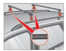
Fig. 130 Attachment points for cross bars
