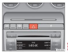
Fig. 92 Centre console: Switch for hazard warning lights
