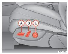
Fig. 107 Front seat: Adjuster controls
