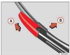
Fig. 177 Removing the wiper blade
