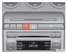
Fig. 150 Centre console: switch for parking aid
