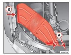
Fig. 198 Air duct on right side of vehicle
