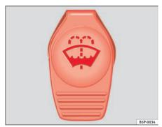
Fig. 176 In the engine compartment: Cap of windscreen washer fluid reservoir.
