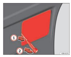
Fig. 227 Remove the cover of the tailgate trim
