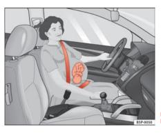
Fig. 14 Positioning seat belts during pregnancy
