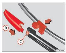
Fig. 178 Fitting the wiper blade
