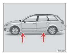
Fig. 190 Changing the wheel: The jacking points
