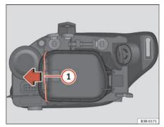
Fig. 206 Side light bulb (outside of vehicle)
