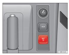
Fig. 182 Detailed view of the centre console: Button for the tyre pressure monitoring system
