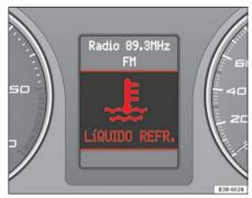
Fig. 54 Display: Coolant level warning
