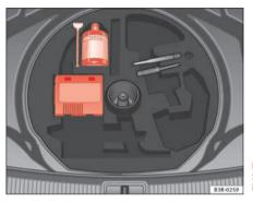
Fig. 187 Tyre Mobility System under floor panel in luggage compartment
