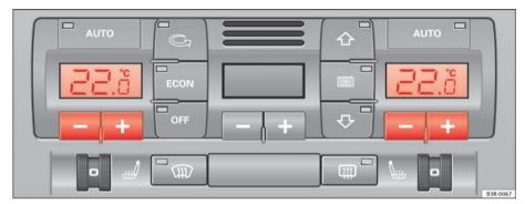
Fig. 141 Climate control controls
