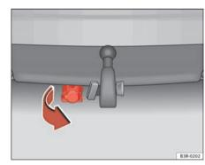
Fig. 163 Rear bumper: Pulling down the connecting socket
