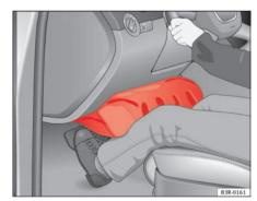
Fig. 22 Inflated airbags protect in a frontal collision
