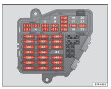
Fig. 197 Schematic drawing of fuse box at the left-hand end of instrument panel: Fuses (without fuse cover)
