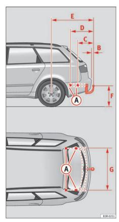
Fig. 166 Attachment points for towing bracket
