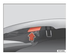
Fig. 171 Release catch under the bonnet
