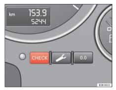
Fig. 53 Instrument panel: CHECK button
