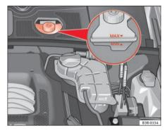
Fig. 181 Engine compartment: markings on brake fluid reservoir
