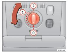
Fig. 82 Details of headliner: Rotary sun roof control
