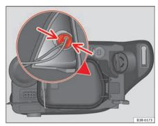
Fig. 207 Side light bulb (outside of vehicle)
