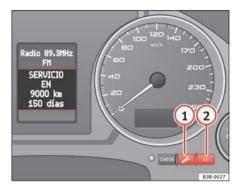
Fig. 52 Detailed view of the instrument panel: Service indicator
