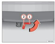
Fig. 165 Rear bumper: fitting the cover piece
