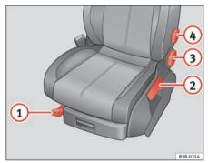
Fig. 106 Adjuster controls on driver's seat
