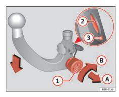
Fig. 160 Removable towing bracket: Setting the spring mechanism to the "ready" position
