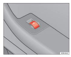
Fig. 81 Switch on front passenger's door
