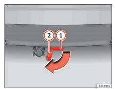
Fig. 157 Rear bumper: Open the cover piece
