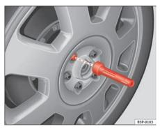
Fig. 192 Changing the wheel: Hexagonal socket in screwdriver handle to turn the wheel bolts
