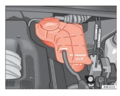
Fig. 175 Engine compartment: Liquid coolant deposit
