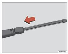
Fig. 180 Fit the rear window wiper blade
