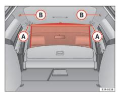
Fig. 121 Retainers for the partition grille
