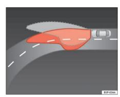
Fig. 91 Self-directing headlights when driving
