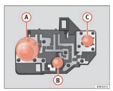
Fig. 229 Position of the bulbs in the bulb holder. Example: Rear lights in the tailgate
