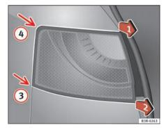
Fig. 220 Removing rear light from side panel
