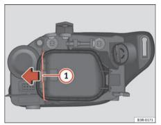
Fig. 208 Side light bulb (inside of vehicle)
