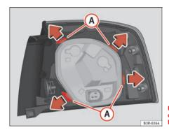
Fig. 221 Retaining tabs on reverse side of rear light
