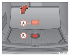
Fig. 185 Access to the toolbox and jack
