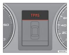
Fig. 45 Display: system fault
