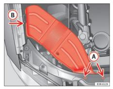
Fig. 199 Air duct on right side of vehicle
