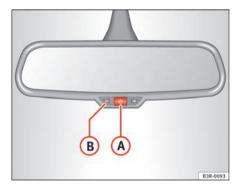
Fig. 104 Interior rear view mirror with antidazzle setting: Indicator lamp and on/off switch
