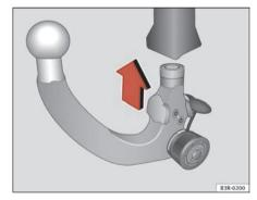
Fig. 161 Removable towing bracket: inserting the ball joint
