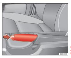
Fig. 149 Detail of the centre console: Handbrake applied
