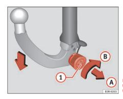
Fig. 164 Removable towing bracket: Removing the ball joint
