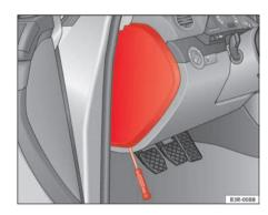
Fig. 196 Left side of dash panel: Fuse box cover
