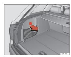
Fig. 126 Luggage compartment: Side trim with closed storage compartment
