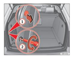
Fig. 219 Luggage compartment: Location of the bolt securing the rear light
