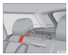
Fig. 35 Retainer strap: correct adjustment and fitting
