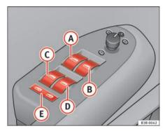
Fig. 80 Detail of the driver's door: Control switches
