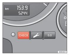
Fig. 43 Detailed view of the instrument panel: CHECK button
