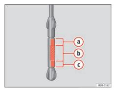
Fig. 173 Markings on oil dipstick
