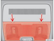
Fig. 83 Details of headliner: Points for applying screwdriver
