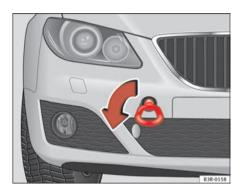
Fig. 238 Fitting the towing eye to front rear of the vehicle
