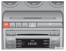
Fig. 146 Detail of the centre console: ESP button
