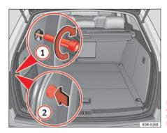
Fig. 225 Luggage compartment: Location of the bolt securing the rear light unit
