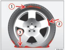
Fig. 194 The Tyre Mobility System is not suitable for repairing this type of damage to tyres.
