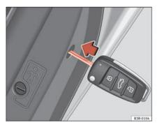
Fig. 73 Enabling manual locking
