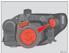
Fig. 201 Turn signal bulb
