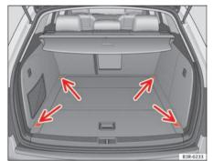
Fig. 117 Location of fastening rings in luggage compartment
