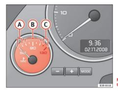
Fig. 38 Engine coolant temperature gauge
