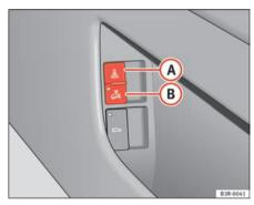
Fig. 79 Interior monitor switch
