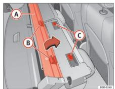
Fig. 123 Installing luggage compartment cover / partition grille
