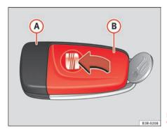
Fig. 69 Master key: Opening the cover
