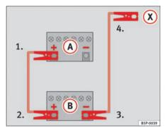
Fig. 237 How to connect the jump leads
