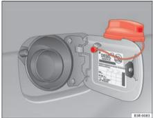
Fig. 168 Fuel tank flap with tank cap attached
