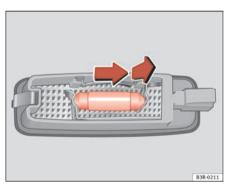
Fig. 236 Removing sun visor light
