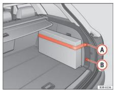
Fig. 119 Retaining strap attached to right-hand side lining
