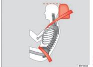
Fig. 4 Properly adjusted head restraint viewed from the side
