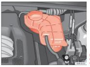
Fig. 181 Engine compartment: Liquid coolant deposit
