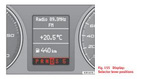
The current selector lever position is shown in the dash panel.
