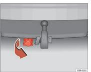
Fig. 169 Rear bumper: Pulling down the connecting socket
