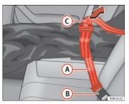
Fig. 129 Fastening the ski bag in the seatbelt buckle
