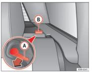
Fig. 127 Backrest release lever
