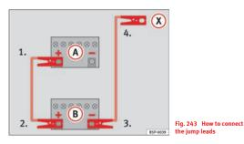
$\Rightarrow$  fig. 243 (A) shows the flat battery and (B) the charged battery.
