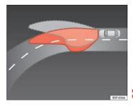
Fig. 91 Self-directing headlights when driving
