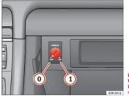
Fig. 27 In the glovebox: key for enabling and disabling front passenger airbag
