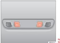
Fig. 96 Details of headliner: rear reading lights
