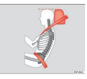
Fig. 13 Correct belt web and head restraint positions, viewed from side The following features are available to adjust the seat belt in the shoulder region:
