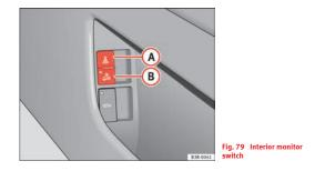
You should disable the interior monitor if there is a possibility that the alarm could be triggered, e.g. by a pet or by an object moving about inside the car  $\Rightarrow$   $\triangle$ . The tow-away protection feature, which is integrated into the alarm system, should be disabled if the car is being towed or transported (e.g. by rail or ship).
