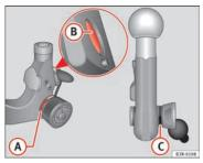
Fig. 165 Removable towing bracket: Ball joint
