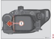
Fig. 214 Side light bulb (inside of vehicle)
