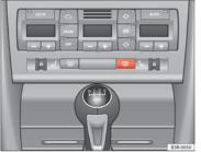
Fig. 98 Switch for heated rear window
