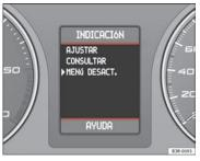
Fig. 62 Display: Main menu Some of your vehicle's functions can be adjusted, activated and controlled by **menus**. With the aid of the menus you can then also select the information you wish to see displayed on the DIS display. This is only possible when the ignition is on. The menu is enabled using the (Reset) button on the windscreen wiper lever  $\Rightarrow$  page 87, fig. 61.
