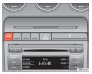
Fig. 146 Detail of the centre console: ESP button
