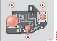
Fig. 235 Position of the bulbs in the bulb holder. Example: Rear lights in the tailgate The bulbs are secured with a bayonet fastener. The table below gives an overview of the bulb positions.
