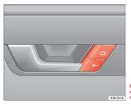
Fig. 71 Detail of driver door: Central locking switch
