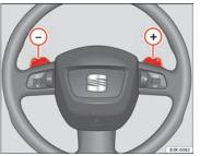
Fig. 159 Steering wheel: Tiptronic controls
