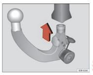
Fig. 167 Removable towing bracket: inserting the ball joint
