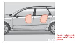
In some **side collisions**, the side airbag is triggered on the impact side of the vehicle  $\Rightarrow$  fig. 24.
