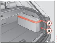
Fig. 119 Retaining strap attached to right-hand side lining
