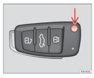
Fig. 67 Remote control key: Release button
