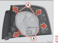
Fig. 227 Retaining tabs on reverse side of rear light
