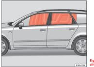
Fig. 26 Deployed curtain airbags
