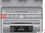
Fig. 160 Centre console with ESP switch
