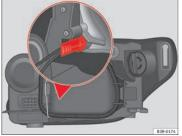
Fig. 215 Side lights. Bulb holder grip in vertical position
