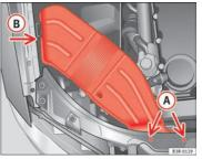
Fig. 204 Air duct on right side of vehicle
