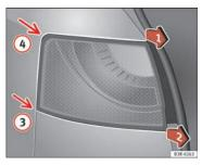
Fig. 226 Removing rear light from side panel
