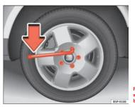
Fig. 195 Changing the wheel: Loosen the wheel bolts
