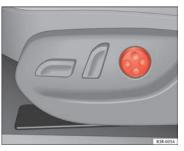
Fig. 110 Front seat: Adjuster switch for lumbar support
