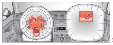
Fig. 20 Airbag covers reacting when the front airbags are triggered
