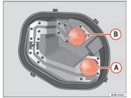
Fig. 228 Position of the bulbs in the bulb holder: Example: Outer left rear light
