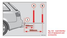
The equipment/accessories mounted must not protrude more than 700 mm from the ball joint (1).
