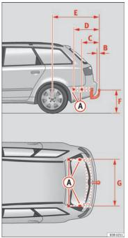
Fig. 172 Attachment points for towing bracket
