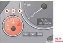
Fig. 38 Engine coolant temperature gauge
