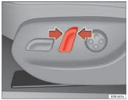
Fig. 109 Front seat: Backrest adjuster switch
