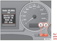
Fig. 52 Detail of the dash panel insert: Service indicator display
