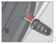
Fig. 73 Enabling manual locking
