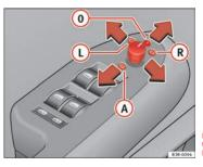
Fig. 105 Detailed view of the armrest: Adjuster knob
