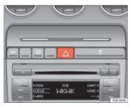
Fig. 92 Centre console: Switch for hazard warning lights Press the switch ▲ ⇒ page 122, fig. 92 to switch the hazard warning lights on or off.
