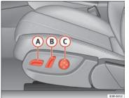
Fig. 107 Front seat: Adjuster controls
