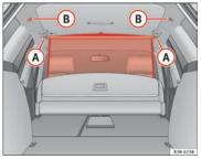
Fig. 121 Retainers for the partition grille
