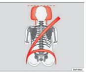
Fig. 12 Correct belt web and head restraint positions, viewed from front
