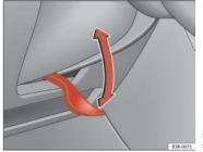
Fig. 145 Lever beneath steering column
