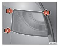
Fig. 230 Fitting the rear light unit
