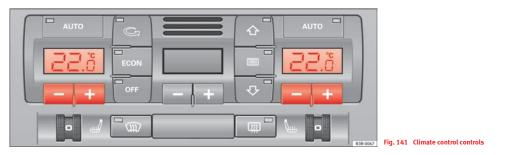
The left-hand display shows the temperature selected for the left-hand side and the right-hand display the temperature for the right-hand side.
