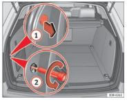
Fig. 225 Luggage compartment: Location of the bolt securing the rear light
