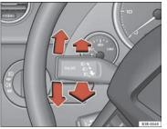
Fig. 93 Turn signal and main beam headlight lever
