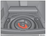
Fig. 162 Luggage compartment: Spare wheel with towing bracket
