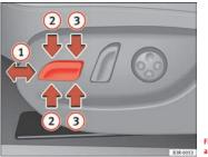
Fig. 108 Front seat: Seat adjustment switches
