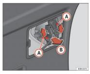
Fig. 234 Remove the bulb holder
