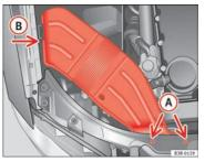
Fig. 216 Air duct on right side of vehicle
