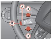
Fig. 152 Controls for the cruise control system
