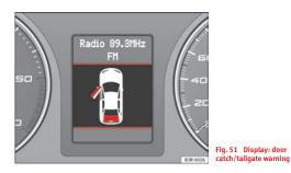
The door catch/tailgate warning symbol lights up if *one or more* of the doors, or the bonnet or tailgate are not properly closed when the ignition is on. The symbol also indicates *which* of these is not properly closed. The display in the illustration  $\Rightarrow$  fig. 51 shows that the front left door is open.
