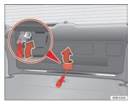
Fig. 76 Detail of the tailgate: emergency unlocking mechanism
