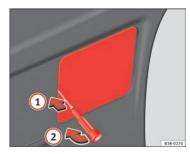
Fig. 233 Remove the cover of the tailgate trim
