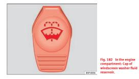
The container for the windscreen washer contains the cleaning fluid for the windscreen and the headlight washer system\*. The container is located in the engine compartment (front left). The filler cap is marked with the symbol  $\widehat{\Psi} \Rightarrow$  fig. 182.
