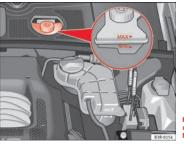
Fig. 187 Engine compartment: markings on brake fluid reservoir
