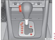
Fig. 154 Detail of the centre console: Selector lever with lock button
