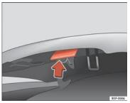
Fig. 177 Release catch under the bonnet
