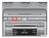
Fig. 28 Warning lamp for deactivated passenger airbag in centre console
