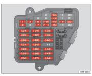
Fig. 203 Schematic drawing of fuse box at the left-hand end of instrument panel: Fuses (without fuse cover)
