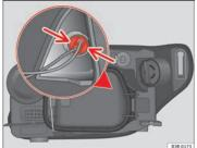
Fig. 213 Side light bulb (outside of vehicle)
