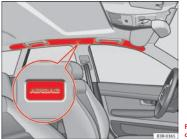
Fig. 25 Location of left curtain airbag
