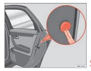
Fig. 72 Manual locking device
