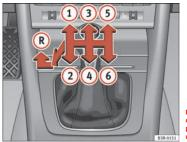
Fig. 153 Detail of the centre console: gear shift pattern of a 6-speed manual gearbox
