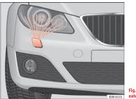
Fig. 103 Headlight with extended washer jet
