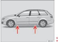
Fig. 196 Changing the wheel: The jacking points
