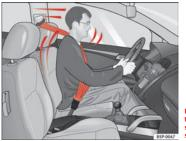
Fig. 10 A driver wearing the seat belt properly: is secured by the belt in sharp braking
