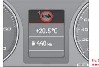
Fig. 56 Display: Speed warning function
