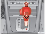
Fig. 157 Centre console: Manual gear selection (tiptronic mode)
