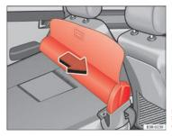
Fig. 122 Removing luggage compartment cover / partition grille
