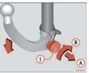
Fig. 170 Removable towing bracket: Removing the ball joint
