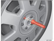
Fig. 198 Changing the wheel: Hexagonal socket in screwdriver handle to turn the wheel bolts After loosening the wheel bolts and raising the vehicle with the jack, change the wheel as described below:
