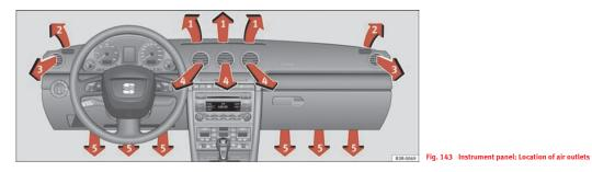
The air outlets  $\Rightarrow$  fig. 143 (3) and (4) can be operated as follows:
