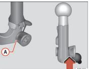
Fig. 168 Removable towing bracket: Safety check
