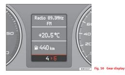
Use the gear display to save fuel. The display in the instrument cluster  $\Rightarrow$  fig. 50 recommends that you select the gear indicated by the arrow. It may also skip a gear, and recommend changing up from 4th gear to 6th gear, for example.
