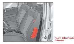
The front side airbags are located in the driver's seat and front passenger's seat backrests  $\Rightarrow$  fig. 23. The rear side airbags are located in the rear wheel housing lining. The locations are identified by the text "AIRBAG" in the upper region of the backrests and in the rear wheel housing lining.
