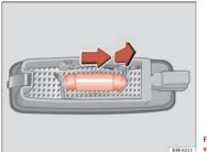
Fig. 242 Removing sun visor light
