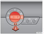
Fig. 85 Detailed view of the instrument panel: Light switch
