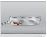
Fig. 241 Removing sun visor light
