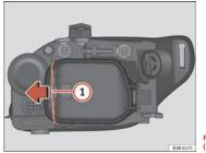
Fig. 212 Side light bulb (outside of vehicle)
