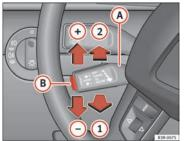
Fig. 151 Controls for the cruise control system
