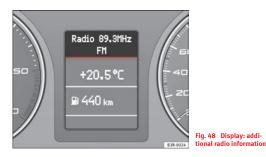
If the radio is switched on and no Priority 2 faults are indicated by the autocheck control, the "OK" symbol will go out and the display will show the name or frequency of the selected radio station and various other information, depending on the type of radio fitted.
