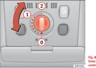
Fig. 82 Details of headliner: Rotary sun roof control
