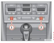
Fig. 144 Detailed view of instrument panel: Thumbwheel controls for seat heating
