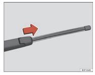
Fig. 185 Remove rear window wiper blade
