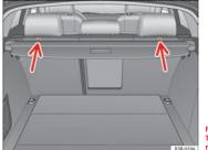
Fig. 34 Position of the Top Tether rings on the rear tray
