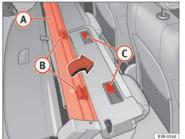
Fig. 123 Installing luggage compartment cover / partition grille
