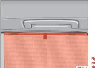
Fig. 100 Sun blind extended to cover rear side window
