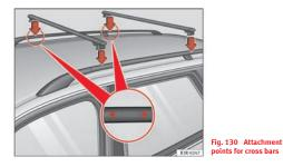
The cross-bars must be fitted exactly between the points marked on the roof railings  $\Rightarrow$  fig. 130. The markings are visible on the inside of the railings.
