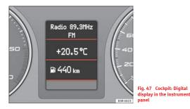
The display for the driver information system is in the centre of the instrument panel.
