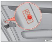
Fig. 77 Childproof lock on the rear doors The rear doors are equipped with childproof locks. These can be operated using the ignition key. The childproof locks are only visible with the doors open.
