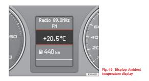
The ambient temperature is shown in the display when the ignition is switched on  $\Rightarrow$  fig. 49. On vehicles with an automatic gearbox, the display does not appear until the driver has engaged a gear.
