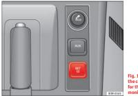
Fig. 188 Detailed view of the centre console: Button for the tyre pressure monitoring system
