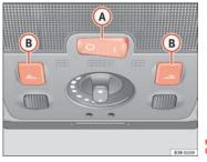
Fig. 94 Details of headliner: front interior lights
