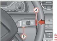
Fig. 58 Windscreen wiper lever: Function selector switch
