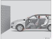
Fig. 6 Vehicle about to hit a wall: the occupants are not wearing seat belts
