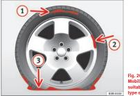
Fig. 200 The Tyre Mobility System is not suitable for repairing this type of damage to tyres.
