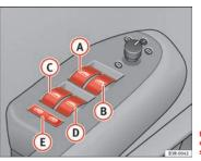
Fig. 80 Detail of the driver's door: Control switches
