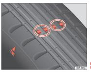
Fig. 189 Tyre tread wear indicators
