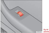
Fig. 81 Switch on front passenger's door
