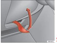
Fig. 145 Lever beneath steering column
