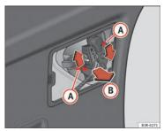
Fig. 235 Remove the bulb holder
