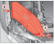
Fig. 214 Air duct on right side of vehicle
