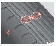
Fig. 187 Tyre tread wear indicators
