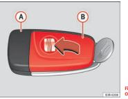
Fig. 69 Master key: Opening the cover
