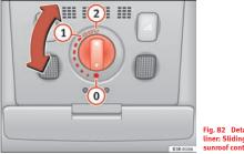
Fig. 82 Detail of headliner: Sliding/tilting sunroof control
