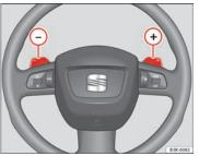
Fig. 159 Steering wheel: tiptronic controls
