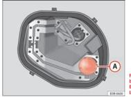
Fig. 228 Position of the bulbs in the bulb holder: Example: Outer left tail light
