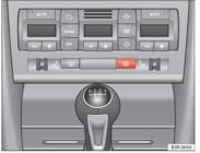
Fig. 98 Switch for heated rear window
