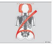
Fig. 12 Correct seat belt and head restraint positions, viewed from front
