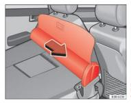
Fig. 122 Removing luggage compartment cover / net partition
