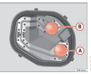
Fig. 227 Position of the bulbs in the bulb holder: Example: Outer left tail light
