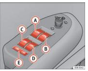
Fig. 80 Detail of the driver door: Control switches
