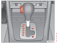
Fig. 154 Detailed view of the centre console: Selector lever with lock button
