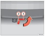
Fig. 171 Rear bumper: fitting the cover piece
