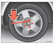
Fig. 193 Changing the wheel: Loosen the wheel bolts
