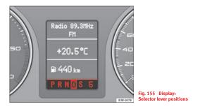
The current selector lever position is shown on the instrument panel display.
