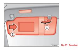
The sun visors ① for the driver and the front passenger can be pulled out of their mountings in the centre of the vehicle and turned towards the doors  $\Rightarrow$  fig. 99.
