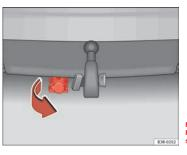
Fig. 169 Rear bumper: Pulling down the power socket
