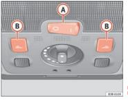
Fig. 94 Detail of headliner: front interior lights
