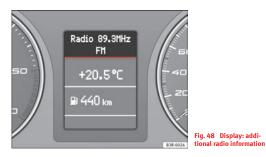
If the radio is switched on and no Priority 2 faults are indicated by the autocheck control, depending on the type of radio fitted, the display will show the name or frequency of the selected radio station and complementary information, once the "OK" symbol has gone out.
