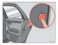
Fig. 72 Manual locking device
