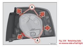
There are four securing tabs on the inside of the tail light unit.
