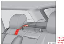
Fig. 35 Retainer strap: correct adjustment and fitting
