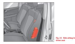
The front side airbags are located in the driver seat and front passenger seat backrest  $\Rightarrow$  fig. 23. The rear side airbags\* are located in the rear wheel housing lining. The locations are identified by the text "AIRBAG" in the upper region of the backrests and in the rear wheel housing lining.
