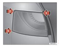
Fig. 230 Fitting the tail light unit
