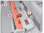
Fig. 123 Installing luggage compartment cover / net partition
