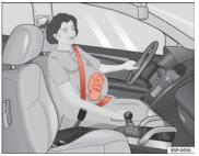
Fig. 14 Positioning seat belts during pregnancy
