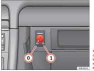
Fig. 27 In the glove compartment: switch for activating and deactivating the front passenger airbag
