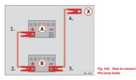
$On \Rightarrow fig. 245$  (A) shows the flat battery and (B) the charged battery.
