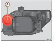
Fig. 206 Main beam headlights
