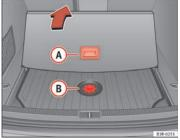
Fig. 189 Access to the toolbox and jack
