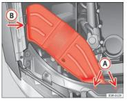
Fig. 202 Air duct on right side of vehicle
