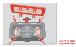
Remove the tulip-shaped fitting by pressing on its inside edge using the flat side of a screwdriver.  Remove the protective cover and remove the bulb from the housing.
