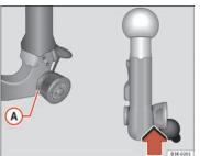
Fig. 168 Removable towing bracket: Safety check
