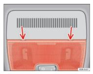
Fig. 83 Detail of headliner: Points for applying screwdriver
