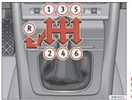
Fig. 153 Detailed view of the centre console: gear shift pattern of a 6-speed manual gearbox
