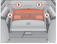
Fig. 121 Retainers for the net partition
