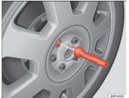
Fig. 196 Changing the wheel: Hexagonal socket in screwdriver handle to turn the wheel bolts
