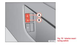
You should disable the interior monitoring if there is a possibility that the alarm could be triggered, e.g. by a pet or by an object moving inside the vehicle  $\Rightarrow$   $\triangle$ . The tow-away protection feature, which is integrated into the alarm system, should be disabled if the vehicle is being towed or transported (e.g. by rail or ship).
