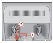
Fig. 84 Detail of headliner: Crank handle for manual operations
