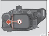
Fig. 212 Side light bulb (inside of vehicle)
