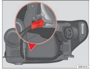
Fig. 213 Side lights. Bulb holder grip in vertical position
