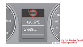
The speed warning function will warn the driver if a pre-set maximum speed is exceeded. The system gives an warning buzzer signal if the set speed is
