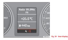
Use the gear display to save fuel. The display  $\Rightarrow$  fig. 50 on the instrument panel recommends that you select the gear indicated by the arrow. It may also skip a gear, and recommend changing up from 4th gear to 6th gear, for example.
