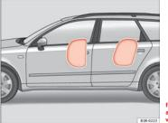
Fig. 24 Inflated side airbag on left side of vehicle
