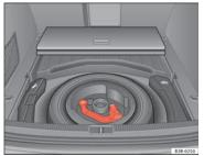
Fig. 162 Luggage compartment: Spare wheel with towing bracket
