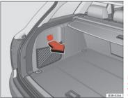
Fig. 126 Luggage compartment: Side trim with closed storage compartment
