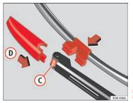
Fig. 182 Fitting the wiper blade
