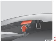
Fig. 176 Release catch under the bonnet
