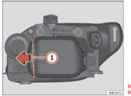
Fig. 210 Side light bulb (outside of vehicle)
