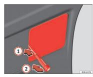
Fig. 234 Remove the cover of the tailgate trim
