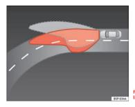
Fig. 91 Adaptive headlights when driving
