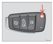
Fig. 67 Remote control key: Release button
