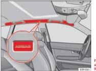
Fig. 25 Location of head airbags on the left side of the vehicle
