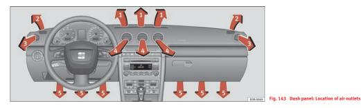
The air outlets  $\Rightarrow$  fig. 143 (3) and (4) can be operated as follows:
