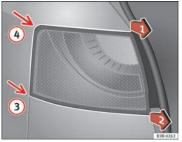
Fig. 225 Removing tail light from side panel
