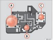
Fig. 236 Position of the bulbs in the bulb holder. Example: Tail lights on the tailgate
