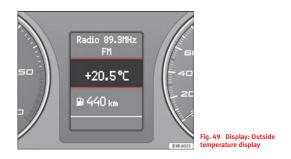
The outside temperature is shown in the display when the ignition is switched on  $\Rightarrow$  fig. 49. In vehicles with an automatic gearbox, the display does not appear until the driver has engaged a gear.
