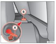
Fig. 127 Backrest release lever
