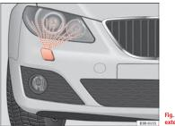
Fig. 103 Headlight with extended washer jet
