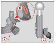
Fig. 165 Removable towing bracket: Ball joint
