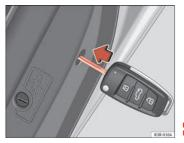
Fig. 73 Activating manual locking
