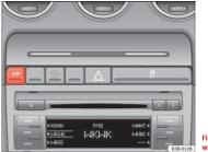
Fig. 160 Centre console with ESP switch
