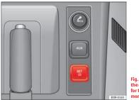
Fig. 186 Detailed view of the centre console: Button for the tyre pressure monitoring system
