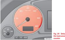
Fig. 39 Detailed view of the instrument panel: Rev
