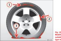
Fig. 198 The Tyre Mobility System is not suitable for repairing this type of damage to tyres.
