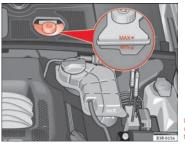
Fig. 185 Engine compartment: markings on brake fluid reservoir
