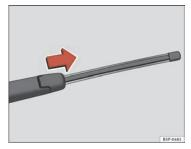
Fig. 183 Removing rear window wiper blade
