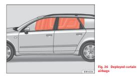
During some **side collisions** the curtain airbag is triggered on the impact side of the vehicle  $\Rightarrow$  fig. 26.
