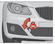
Fig. 246 Fitting the towing eye to front rear of the vehicle
