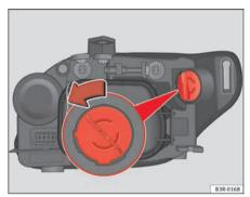
Fig. 190 Turn signal bulb
