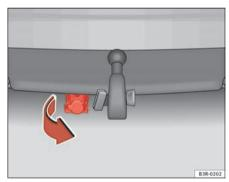
Fig. 155 Rear bumper: Pulling down the connecting socket
