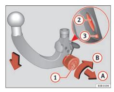
Fig. 152 Removable towing bracket: Setting the spring mechanism to the "ready" position
