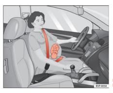
Fig. 14 Positioning seat belts during pregnancy
