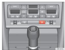
Fig. 96 Switch for heated rear window
