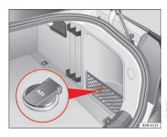
Fig. 128 Detailed view of the side trim in the luggage compartment: 12-yolt socket
