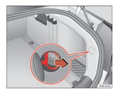
Fig. 161 Luggage compartment: Releasing the fuel tank flap by hand
