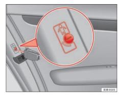
Fig. 75 Childproof lock on the rear doors
