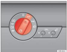
Fig. 84 Detailed view of instrument panel: Light switch
