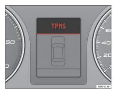
Fig. 45 Display: system fault
