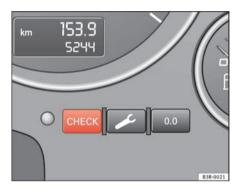
Fig. 52 Instrument panel: CHECK button
