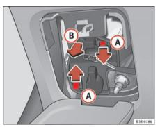
Fig. 216 Remove the bulb holder
