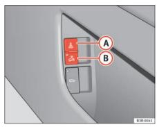
Fig. 77 Interior monitor switch
