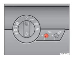
Fig. 88 Switch for daytime running lights
