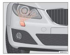
Fig. 101 Headlight with extended washer jet
