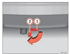
Fig. 149 Rear bumper: Open the cover piece
