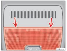
Fig. 81 Details of headliner: Points for applying screwdriver
