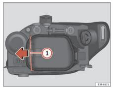
Fig. 197 Side light bulb (inside of vehicle)
