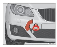
Fig. 226 Fitting the towing eye to front rear of the vehicle
