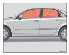
Fig. 26 Deployed curtain airbags
