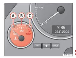
Fig. 38 Engine coolant temperature gauge
