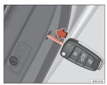
Fig. 72 Enabling manual locking
