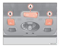
Fig. 92 Details of headliner: front interior lights
