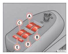
Fig. 78 Detail of the driver's door: Control switches
