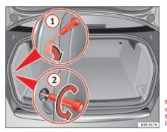
Fig. 208 Luggage compartment: Location of the bolt securing the rear light
