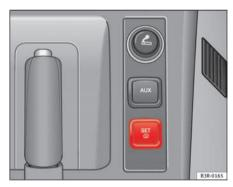
Fig. 172 Detailed view of the centre console: Button for the tyre pressure monitoring system
