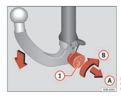
Fig. 156 Removable towing bracket: Removing the ball joint
