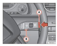
Fig. 59 Windscreen wiper lever: On-board computer controls
