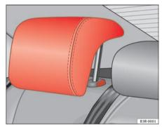
Fig. 5 Head restraints in correct position
