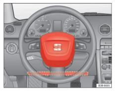
Fig. 17 Driver's Airbag in the steering wheel and kee airbag in the instrument panel
