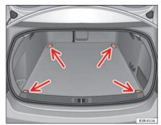
Fig. 115 Location of fastening rings in luggage compartment
