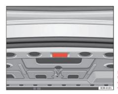
Fig. 95 Detailed view of the top of the luggage compartment: luggage compartment lighting
