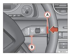
Fig. 62 Windscreen wiper lever: Reset button and rocker switch
