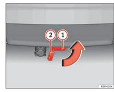
Fig. 157 Rear bumper: fitting the cover piece
