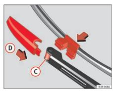
Fig. 170 Fitting the wiper
