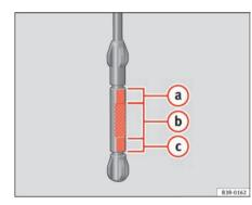
Fig. 165 Markings on oil dipstick
