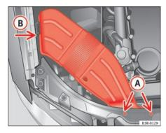
Fig. 187 Air duct on right side of vehicle
