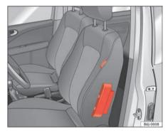
Fig. 23 Side airbag in driver seat
