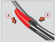
ig. 169 Removing the wiper blade
