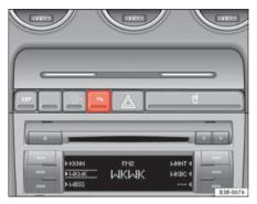
Fig. 142 Centre console: switch for parking aid
