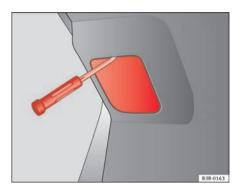
Fig. 215 Remove the cover in the tailgate
