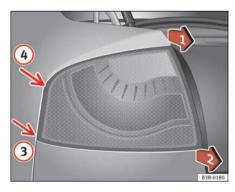
Fig. 209 Removing rear light from side panel
