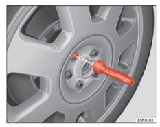
Fig. 181 Changing the wheel: Hexagonal socket in screwdriver handle to turn the wheel bolts
