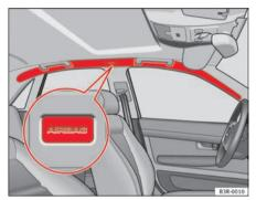
Fig. 25 Location of left curtain airbag
