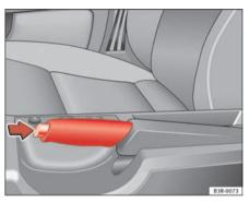
Fig. 141 Detail of the centre console: Handbrake applied
