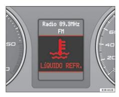
Fig. 53 Display: Coolant level warning
