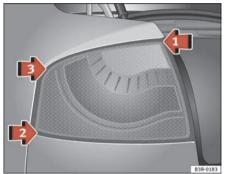
Fig. 212 Fitting the rear light unit
