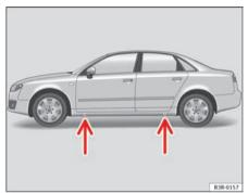
Fig. 179 Changing the wheel: The jacking points
