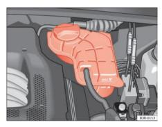
Fig. 167 Engine compartment: Liquid coolant deposit
