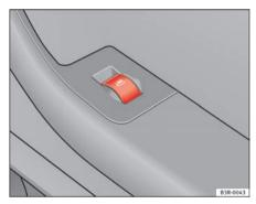
Fig. 79 Switch on front passenger's door
