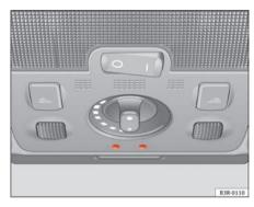
Fig. 93 Details of headliner: background lighting
