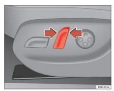
Fig. 107 Front seat: Backrest adjuster switch
