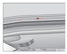
Fig. 122 Attachment points for carrier units
