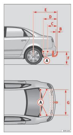
Fig. 158 Attachment points for towing bracket
