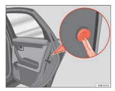
Fig. 71 Manual locking device
