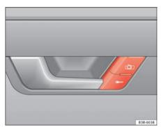
Fig. 70 Detail of driver door: Central locking switch
