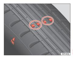
Fig. 173 Tyre tread wear indicators
