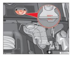
Fig. 171 Engine compartment: markings on brake fluid reservoir
