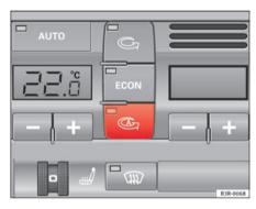
Fig. 134 Button for automatic air recirculation
