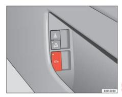
Fig. 73 Driver's door: Unlocking the tailgate
