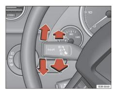
Fig. 91 Turn signal and main beam headlight
