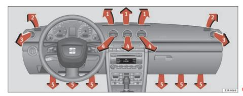
Fig. 135 Instrument panel: Location of air outlets
