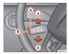
Fig. 144 Controls for the cruise control system
