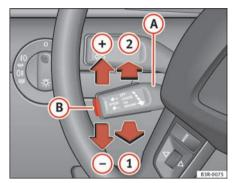
Fig. 143 Controls for the cruise control system
