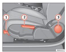
Fig. 104 Adjuster controls on driver's seat
