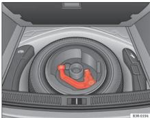
Fig. 148 Luggage compartment: Spare wheel with towing bracket
