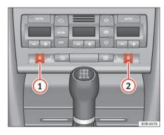
Fig. 136 Detailed view of instrument panel: Thumbwheel controls for seat heating
