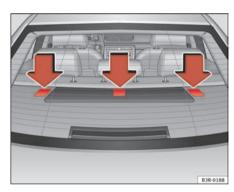
Fig. 34 Position of the three Top Tether rings on the rear tray
