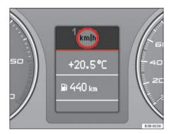
Fig. 55 Display: Speed warning function
