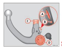
Fig. 150 Removable towing bracket: Ball joint
