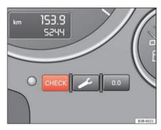
Fig. 56 Detailed view of the instrument panel: CHECK button
