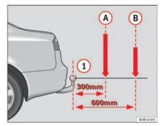
Fig. 147 Load distribution of equipment and accessories
