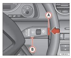
Fig. 57 Windscreen wiper lever: Function selector switch
