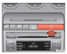
Fig. 123 Detailed view of instrument panel: Drink holders
