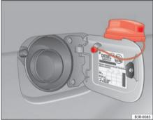
Fig. 160 Fuel tank flap with tank cap attached
