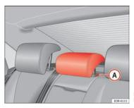
Fig. 113 Centre rear seat: Head restraints
