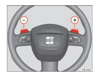
Fig. 150 Steering wheel: Tiptronic controls
