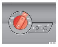
Fig. 85 Detailed view of instrument panel: Light switch
