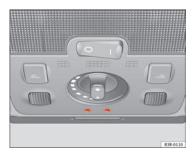
Fig. 94 Details of headliner: background lighting
