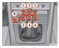
Fig. 144 Detail of the centre console: gear shift pattern of a 6-speed manual gearbox
