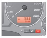
Fig. 42 Detail of the dash panel insert: Distance display
