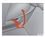
Fig. 136 Lever beneath steering column
