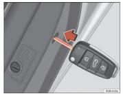
Fig. 73 Enabling manual locking
