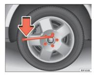
Fig. 183 Changing the wheel: Loosen the wheel bolts
