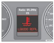
Fig. 54 Display: Coolant level warning
