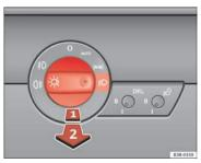
Fig. 84 Detailed view of the instrument panel: Light switch
