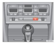
Fig. 97 Switch for heated rear window
