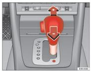
Fig. 148 Centre console: Manual gear selection (tiptronic mode)
