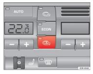
Fig. 133 Button for automatic air recirculation
