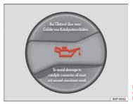
Fig. 171 In the engine compartment: Engine oil filler cap
