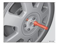
Fig. 186 Changing the wheel: Hexagonal socket in screwdriver handle to turn the wheel bolts
