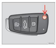
Fig. 67 Remote control key: Release button
