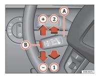
Fig. 142 Controls for the cruise control system
