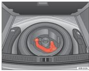
Fig. 153 Luggage compartment: Spare wheel with towing bracket
