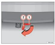
Fig. 154 Rear bumper: Open the cover piece
