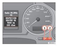
Fig. 52 Detail of the dash panel insert: Service indicator display
