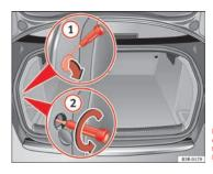
Fig. 213 Luggage compartment: Location of the bolt securing the rear light
