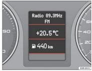
Fig. 47 Cockpit: Digital display in the instrument panel
