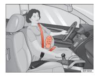
Fig. 14 Positioning seat belts during pregnancy
