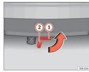
Fig. 162 Rear bumper: fitting the cover piece
