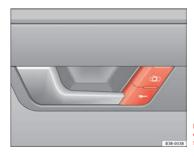
Fig. 71 Detail of driver door: Central locking
