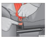
Fig. 15 Removing latch plate from buckle
