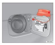
Fig. 165 Fuel tank flap with tank cap attached
