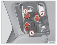
Fig. 221 Remove the bulb holder
