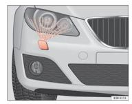
Fig. 102 Headlight with extended washer jet
