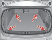
Fig. 116 Location of fastening rings in luggage compartment
