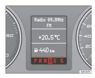
Fig. 146 Display: Selector lever positions
