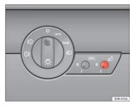
Fig. 86 Detailed view of the instrument panel: Coming home and leaving home functions
