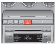
Fig. 91 Centre console: Switch for hazard warning lights
