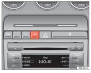
Fig. 141 Centre console: switch for parking aid
