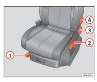
Fig. 105 Adjuster controls on driver's seat
