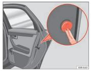
Fig. 72 Manual locking device
