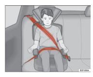
Fig. 31 Forward-facing child seat installed on rear seat.
