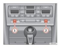
Fig. 135 Detailed view of instrument panel: Thumbwheel controls for seat heating
