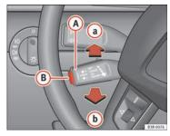
Fig. 143 Controls for the cruise control system
