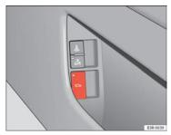
Fig. 74 Driver's door: Unlocking the tailgate
