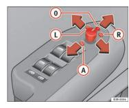
Fig. 104 Detailed view of the armrest: Adjuster knob
