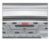
Fig. 96 Detailed view of the top of the luggage compartment: luggage compartment lighting
