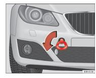
Fig. 231 Fitting the towing eye to front rear of the vehicle
