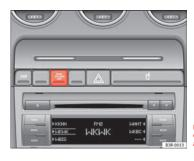
Fig. 28 Warning lamp for deactivated passenger airbag in centre console
