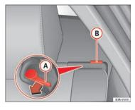
Fig. 118 Backrest release lever
