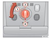
Fig. 81 Details of headliner: Rotary sun roof control
