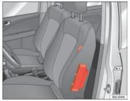
Fig. 23 Side airbag in driver seat
