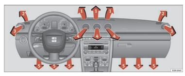
Fig. 134 Instrument panel: Location of air outlets
