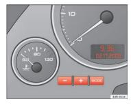
Fig. 40 Detail of the dash panel insert: Digital clock
