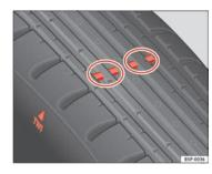
Fig. 178 Tyre tread wear indicators
