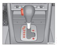
Fig. 145 Detail of the centre console: Selector lever with lock button
