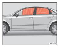
Fig. 26 Deployed curtain airbags
