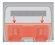
Fig. 82 Detail of headliner: Points for applying screwdriver
