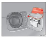
Fig. 163 Fuel tank flap with tank cap attached
