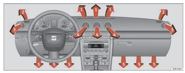
Fig. 132 Dash panel: Location of air outlets
