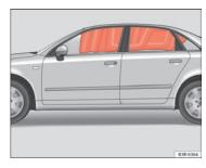
Fig. 26 Deployed curtain airbags
