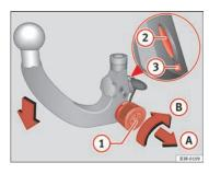
Fig. 155 Removable towing bracket: Setting the spring mechanism to the 'ready' position
