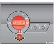
Fig. 84 Detailed view of the dash panel: Light switch
