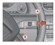
Fig. 60 Windscreen wiper lever: Onboard computer controls
