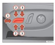
Fig. 107 Front seat: Seat adjustment switches
