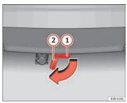
Fig. 152 Rear bumper: Open the cover piece
