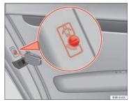
Fig. 76 Childproof lock on the rear doors
