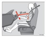
Fig. 1 The proper distance between driver and steering wheel
