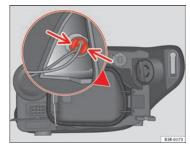
Fig. 197 Side light bulb (outside of vehicle)
