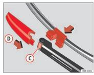
Fig. 171 Fitting the wiper blade
