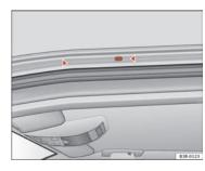
Fig. 119 Attachment points for basic support
