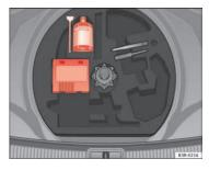
Fig. 177 Tyre Mobility System under floor panel in luggage compartment
