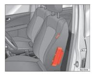
Fig. 23 Side airbag in driver seat
