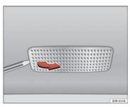
Fig. 228 Removing sun visor light
