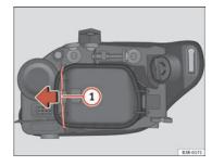
Fig. 196 Side light bulb (outside of vehicle)
