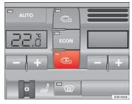
Fig. 131 Button for automatic air recirculation
