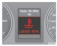
Fig. 54 Display: Coolant level warning
