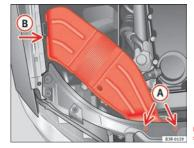
Fig. 200 Air duct on right side of vehicle
