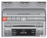
Fig. 149 Centre console with ESP switch
