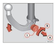
Fig. 159 Removable towing bracket: Removing the ball joint
