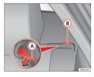
Fig. 116 Backrest release lever
