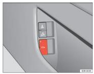
Fig. 74 Driver door: Unlocking the tailgate
