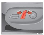
Fig. 108 Front seat: Backrest adjuster switch
