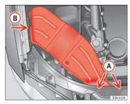
Fig. 201 Air duct on right side of vehicle
