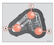
Fig. 213 Position of the bulbs in the bulb holder. Example: Left tail light in side panel
