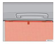
Fig. 99 Sun blind extended to cover rear side window
