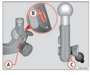
Fig. 154 Removable towing bracket: Ball joint
