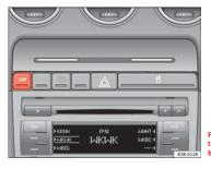
Fig. 135 Detailed view of the centre console: ESP button
