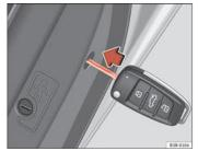
Fig. 73 Activating manual locking
