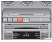
Fig. 139 Centre console: switch for parking aid
