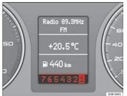
Fig. 147 Display: Manual gear selection (tiptronic mode)
