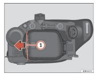
Fig. 198 Side light bulb (inside of vehicle)
