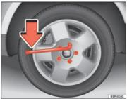
Fig. 179 Changing the wheel: Loosen the wheel
