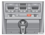
Fig. 97 Switch for heated rear window
