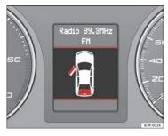
Fig. 51 Display: Door and tailgate warning
