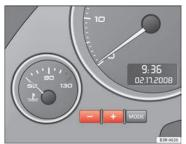
Fig. 87 Instrument panel lighting
