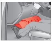
Fig. 22 Inflated airbags protect in a frontal collision.
