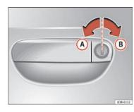
Fig. 70 Turning the key to enable the open and close
