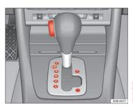
Fig. 143 Detailed view of the centre console: Selector lever with lock button
