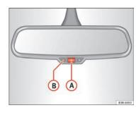
Fig. 103 Interior mirror with anti-dazzle setting: Indicator lamp and on/off switch
