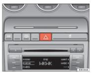
Fig. 91 Centre console: Switch for hazard warning lights
