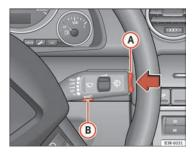
Fig. 63 Windscreen wiper lever: Reset button and rocker switch
