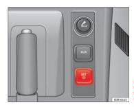
Fig. 173 Detailed view of the centre console: Button for the tyre pressure monitoring system
