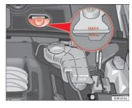
Fig. 172 Engine compartment: markings on brake fluid reservoir
