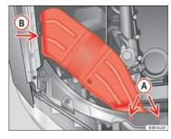
Fig. 189 Air duct on right side of vehicle
