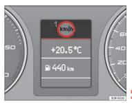
Fig. 56 Display: Speed warning function
