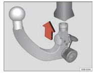
Fig. 156 Removable towing bracket: Inserting the ball joint
