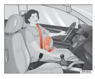
Fig. 14 Positioning seat belts during pregnancy
