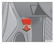
Fig. 164 Detail of footwell area on driver side: lever for unlocking the bonnet.
