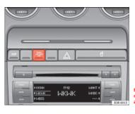
Fig. 28 Warning lamp for deactivated passenger airbag in centre console
