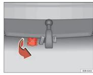
Fig. 158 Rear bumper: Pulling down the power socket
