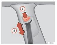
Fig. 16 Belt height adjuster
