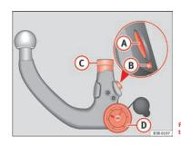
Fig. 153 Removable towing bracket: Ball joint
