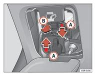
Fig. 220 Remove the bulb holder
