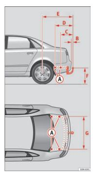
Fig. 161 Attachment points for towing bracket
