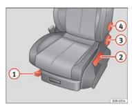
Fig. 105 Adjuster controls on driver seat
