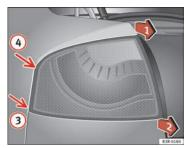
Fig. 211 Removing tail light from side panel
