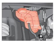
Fig. 168 Engine compartment: Coolant fluid deposit
