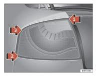
Fig. 215 Fitting the tail light unit
