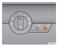
Fig. 86 Detailed view of the dash panel: Coming home and leaving home functions
