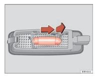
Fig. 229 Removing sun visor light
