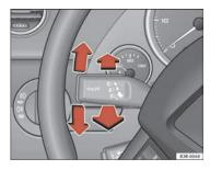
Fig. 92 Turn signal and main beam headlight
