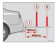
Fig. 150 Load distribution of equipment and accessories
