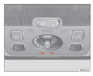
Fig. 94 Detail of headliner: ambient lighting
