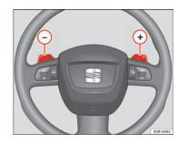
Fig. 148 Steering wheel: tiptronic controls
