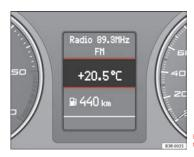
Fig. 49 Display: Outside temperature display
