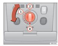
Fig. 81 Detail of headliner: Sliding/tilting sunroof control
