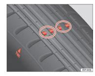
Fig. 174 Tyre tread wear indicators
