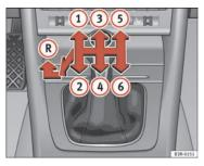
Fig. 142 Detailed view of the centre console: gear shift pattern of a 6-speed manual gearbox
