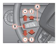
Fig. 140 Controls for the cruise control system
