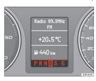
Fig. 144 Display: Selector lever positions
