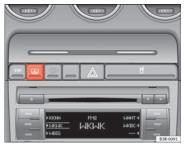
Fig. 100 Switch for electric sun blind on rear window
