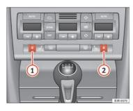
Fig. 133 Detailed view of the dash panel: Thumbwheel controls for seat heating
