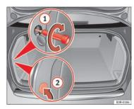
Fig. 216 Luggage compartment: Location of the bolt securing the tail light unit
