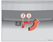
Fig. 160 Rear bumper: fitting the cover piece
