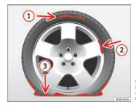
Fig. 184 The Tyre Mobility System is not suitable for repairing this type of damage to tyres.
