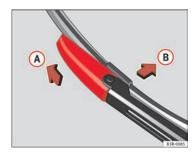
Fig. 170 Removing the wiper blade
