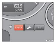
Fig. 53 Instrument panel: CHECK button
