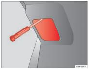
Fig. 219 Remove the cover from the tailgate
