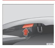
Fig. 165 Release catch under the bonnet
