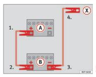
Fig. 230 How to connect the jump leads
