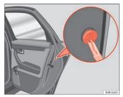
Fig. 72 Manual locking device
