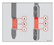
Fig. 166 Markings on oil dipstick
