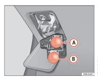
Fig. 221 Position of the bulbs in the bulb holder. Example: Tail lights on the tailgate
