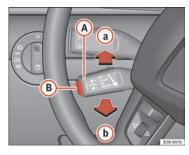
Fig. 141 Controls for the cruise control system
