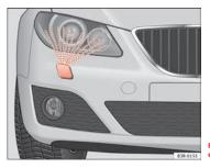
Fig. 102 Headlight with extended washer jet
