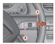
Fig. 58 Windscreen wiper lever: Function selector switch
