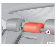
Fig. 113 Centre rear seat: Head restraints
