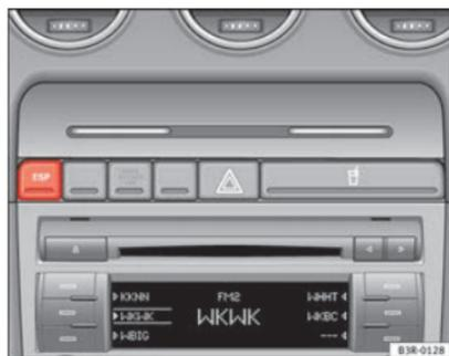
**Fig. 149** Consola central com interruptor do ESP
