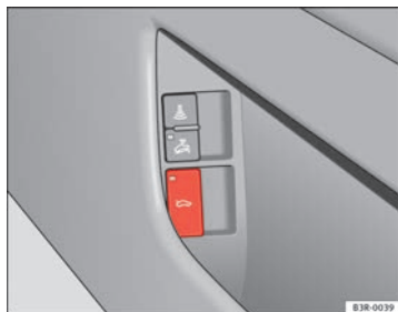
Fig. 74 Driver door: Unlocking the tailgate
