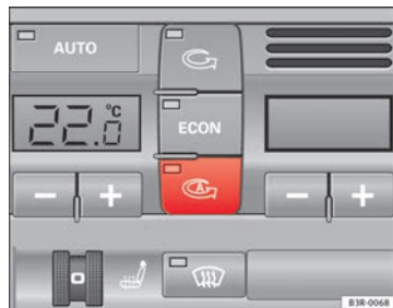
Fig. 131 Button for automatic air recirculation
