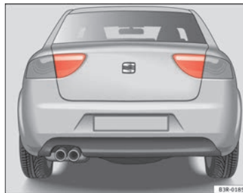
Fig. 214 Overview of tail lights
