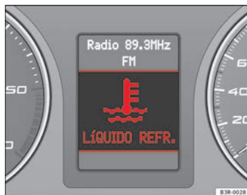
Fig. 54 Display: Coolant level warning
