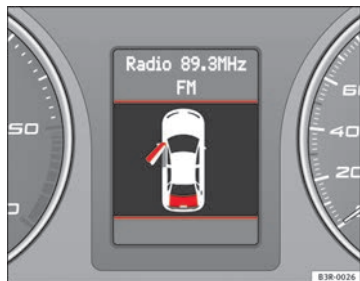
Fig. 51 Display: Door and tailgate warning
