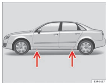
Fig. 180 Changing the wheel: Jack position points
