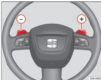
Fig. 148 Steering wheel: tiptronic controls
