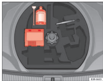
Fig. 177 Tyre Mobility System under floor panel in luggage compartment
