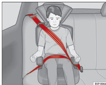
Fig. 31 Forward-facing child seat installed on rear seat.
