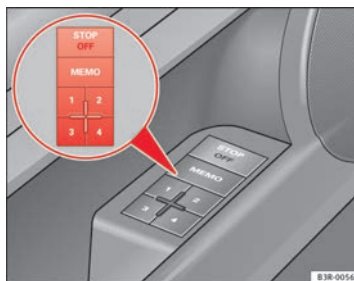
Fig. 110 Driver door: Memory system
