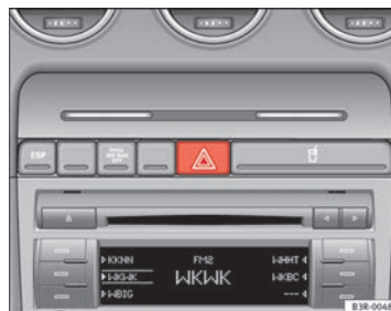
Fig. 91 Centre console: Switch for hazard warning lights
