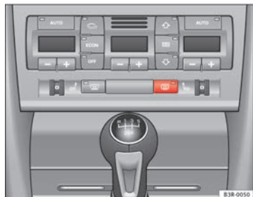
Fig. 97 Switch for heated rear window
