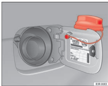
Fig. 163 Fuel tank flap with tank cap attached
