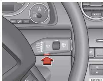
Fig. 61 Windscreen wiper lever: Menu selection button
