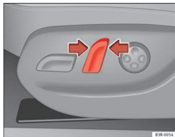
Fig. 108 Front seat: Backrest adjuster switch
