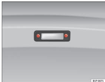
Fig. 222 Number plate light
