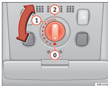
Fig. 81 Detail of headliner: Sliding/tilting sunroof control
