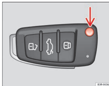
Fig. 67 Remote control key: Release button
