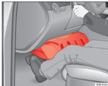
Fig. 22 Inflated airbags protect in a frontal collision.
