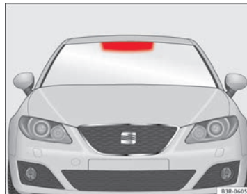
Fig. 162 Location of the electronic toll collection system
