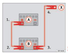
Fig. 156 How to connect the jump leads
