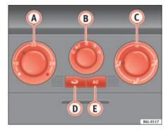
Fig. 86 On the instrument panel: air conditioner controls
