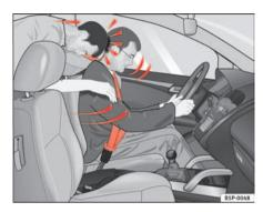
Fig. 9 The unbelted rear passenger is thrown forward violently, hitting the driver wearing a seat
