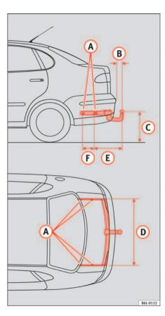
Fig. 116 Attachment points for towing bracket
