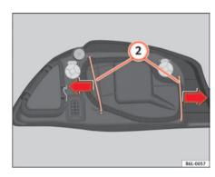
Fig. 140 Dipped headlight lamp
