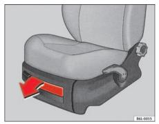
Fig. 77 Stowage compartment under the front passenger seat
