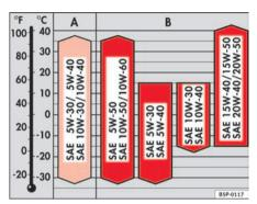
Fig. 119 Types of oil according to temperature
