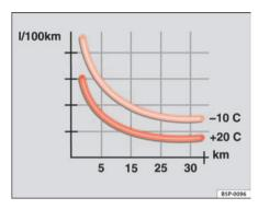
Fig. 115 Fuel consumption in litres per 100 km at two different ambient temperatures
