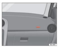
Fig. 18 Front passenger airbag located in dash panel
