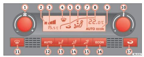
Fig. 88 On the instrument panel; Climatronic controls
