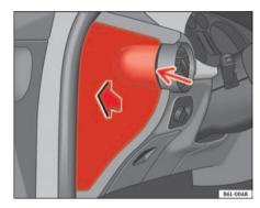
Fig. 136 Fuses in the dash panel
