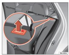
Fig. 74 Button for unlocking the rear back-rest
