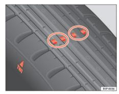
Fig. 127 Tyre tread wear indicators
