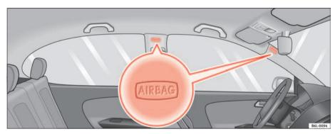
Fig. 23 Location of left curtain airbag
