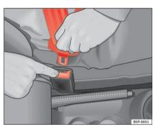
Fig. 15 Removing latch plate from buckle
