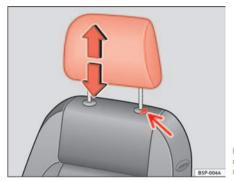
Fig. 70 Adjusting and removing the head restraints
