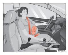
Fig. 14 Positioning seat belts during pregnancy
