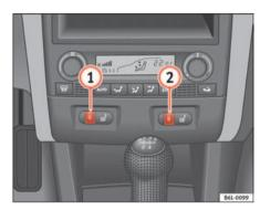
Fig. 72 Thumb wheel for the front seat heating
