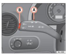
Fig. 102 Turn signal and main beam lever: switch and rocker switch for CCS
