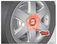
Fig. 129 Changing a wheel: Removing the wheel trim
