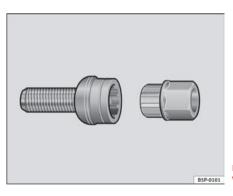
Fig. 135 Theft inhibiting wheel bolts
