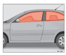
Fig. 24 Deployed curtain airbags
