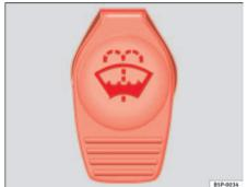
Fig. 123 In the engine compartment: Cap of windscreen washer fluid reservoir.
