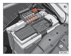
Fig. 137 Fuse box above battery
