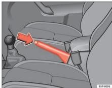
Fig. 97 Handbrake between the front seats
