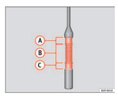
Fig. 120 Engine oil dipstick.
