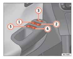
Fig. 52 Section of the driver door: controls for the front and rear windows
