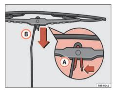
Fig. 125 Changing the rear window wiper blade
