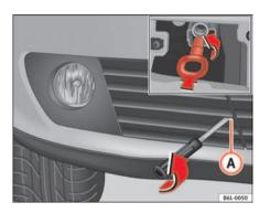
Fig. 157 Towing eye at the front of the vehicle
