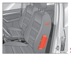
Fig. 21 Side airbag in driver seat
