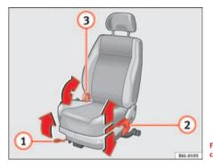
Fig. 71 Front left seat controls
