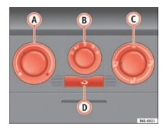
Fig. 84 On the dash panel: Heater controls
