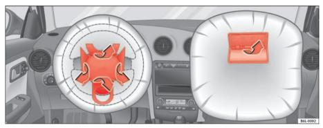
Fig. 20 Airbag covers reacting when the airbags are trig-
