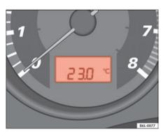
Fig. 38 Digital screen on the instrument panel: outside temperature display
