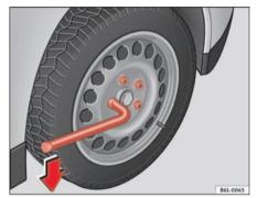
Fig. 131 Changing the wheel: Loosening the wheel bolts
