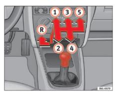
Fig. 93 Central Console: diagram of 5-speed manual gearbox
