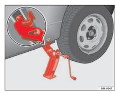
Fig. 133 Fitting the jack
