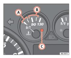
Fig. 33 Engine coolant temperature
