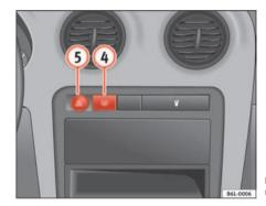
Fig. 58 Instrument panel: rear window heater switch
