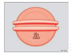
Fig. 122 In the engine compartment: Coolant expansion tank cap
