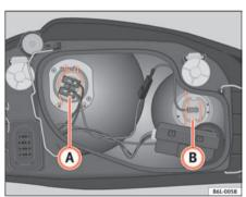
Fig. 143 Main beam lamp
