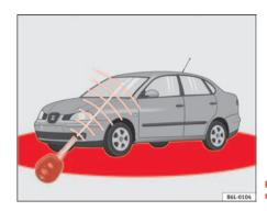
Fig. 49 Range of the remote control
