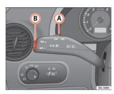
Fig. 99 Turn signal and main beam lever: switch and rocker switch for CCS
