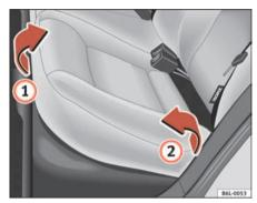
Fig. 73 Folding up the rear seat cushion
