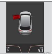
**Fig. 50** On the instrument panel display: door open.
