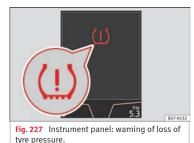
The tyre monitor indicator compares wheel revolutions and, with this information, the tread of each wheel using the ABS sensors. If the rolling circumference of one or more wheels has changed, the tyre monitoring indicator will indicate this on the instrument panel through a warning lamp and a warning to the driver **w** Fig. 227. When only one specific tyre is affected, its position within the vehicle will be indicated.
