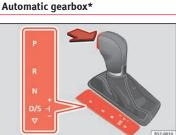
Fig. 53 Automatic gearbox: selector lever positions.
