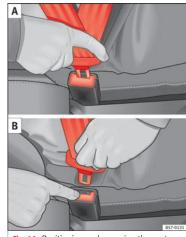
Fig. 16 Positioning and removing the seat belt buckle.
