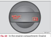
**Fig. 60** In the engine compartment: Engine oil filler cap
