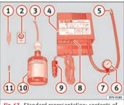
**Fig. 67** Standard representation: contents of the anti-puncture kit.
