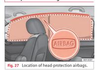
The head-protection airbags are located on both sides in the interior above the doors **w Fig. 27** and are identified with the text "AIRBAG".
