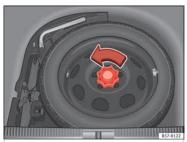
**Fig. 228** Compact temporary spare wheel: raised floor panel.
