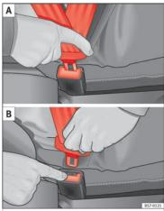
**Fig. 90** Positioning and removing the seat belt buckle.
