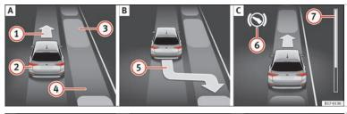
Fig. 203 On the instrument panel display: parallel parking. A Finding a parking space. B Parking position. C Manoeuvring.
