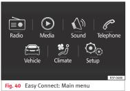
To select the settings menus, press the Easy Connect (CAR) button and the (Setup) function button.
