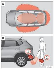
Fig. 123 Keyless Access locking and ignition system: A In the proximity of the car. B Opening the rear lid with sensor-controlled opening (Easy Open)
