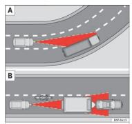
Fig. 182 (A) Vehicle on a bend. (B) Motorcyclist ahead out of range of the radar sensor.
