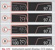
Fig. 171 Instrument panel display: CCS statu indications
