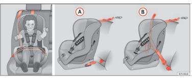
Fig. 30 On the rear seats: Possible installations for the child seat.
