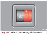
Fig. 136 Next to the steering wheel: Hea light range control
