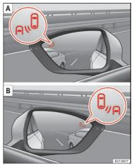
**Fig. 192** In the exterior mirrors: indication of the blind spot detector.
