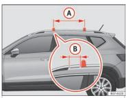
**Fig. 160** Attachment points for the roof railings for the roof carrier system.
