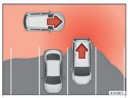
Fig. 211 Schematic representation of the rear cross traffic alert: zone monitored around the vehicle exiting the parking space.
