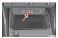
Fig. 124 Centre console: USB/AUX-IN input.
