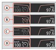
Fig. 186 Instrument panel display: CCS status indications.
