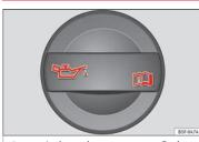
Fig. 241 In the engine compartment: Engine oil filler cap.
