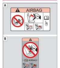
Fig. 29 Airbag stickers - version 1: on the passenger-side sun blind A and on the rear frame of the front passenger's door B.
