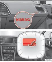
Fig. 21 Front passenger airbag located in dash panel.
