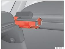
Fig. 121 Removing the stowage compartment tray
