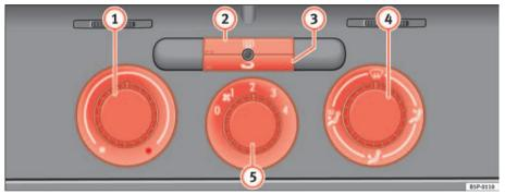
Fig. 122 On the dash panel: Heater controls
