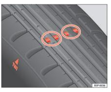
Fig. 168 Tyre tread wear indicators
