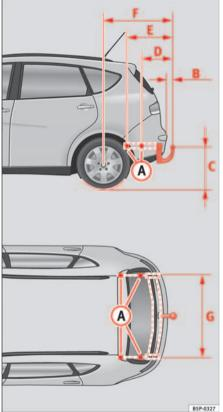
Fig. 155 Attachment points for towing bracket
