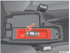
Fig. 119 USB\* connection in the central armrest
