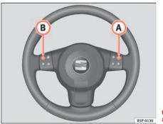
Fig. 58 Steering wheel audio version controls
