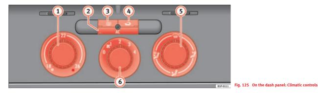
Air recirculation mode  $\Rightarrow$  page 153, fig. 125  $\bigcirc$  prevents strong odours in the outside air from entering the vehicle interior, for example when passing through a tunnel or in queuing traffic.
