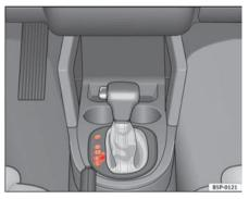
Fig. 134 Section of centre console: selector lever on cars with an automatic gearbox / direct shift gearbox
