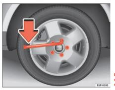
Fig. 172 Changing the wheel: Loosening the wheel bolts
