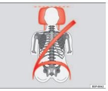
Fig. 13 Correct belt web and head rest positions, viewed from front
