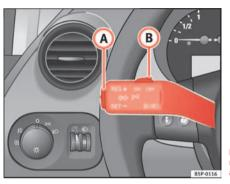
Fig. 141 Turn signal and main beam lever: Switch and rocker switch for CCS
