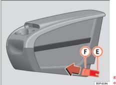
Fig. 109 Mobile stowage compartment Installation
