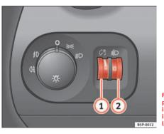
Fig. 75 Detail of the dash panel: Regulation for instrument and switch illumination and headlight range control
