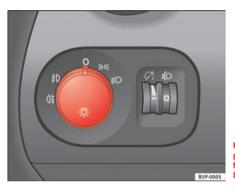
Fig. 73 Detail of the dash panel: Switch for lights, fog lights and rear fog light
