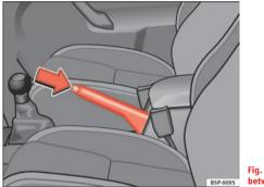
Fig. 140 Handbrake between the front seats
