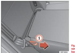
Fig. 98 Folding or opening the front seat backrests
