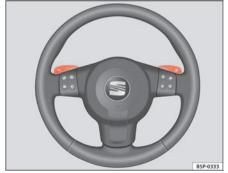
Fig. 139 Steering wheel with levers for automatic gearboxes
