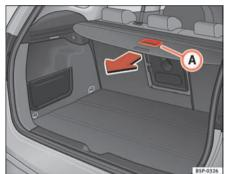
Fig. 120 Operating the stowage compartment tray
