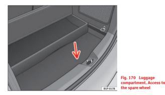
The temporary spare wheel is stored under the floor panel in the luggage compartment and is attached by a thumbnut.
