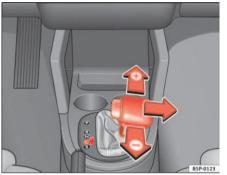
Fig. 138 Changing gear with Tiptronic
