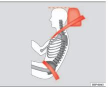
Fig. 14 Correct belt web and head rest positions, viewed from side
