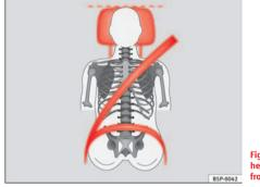
Fig. 3 Properly adjusted head restraint viewed from the front
