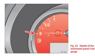
Details of the instrument panel: Fuel gauge
