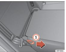
Fig. 97 Folding or opening the rear seat backrests
