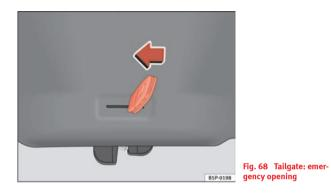
There is a groove in the boot allowing access to the emergency opening mechanism.
