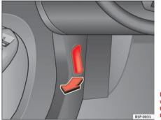
Fig. 157 Detail of the foot well: The release lever for the bonnet is located in the driver side foot well
