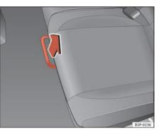
Fig. 95 Unlocking bar for the rear seat
