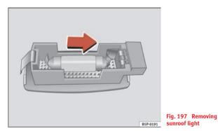
Remove the lamp, moving it in the direction of the arrow and outwards ⇒ fig. 197.
