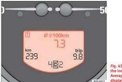
Fig. 42 Digital screen on the instrument panel: Average fuel consumption display
