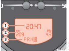
Fig. 36 Detail of the instrument panel: Screen with various displays
