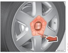
Fig. 171 Changing a wheel: Removing the wheel trim
