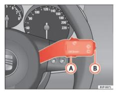
Fig. 45 Windscreen wiper lever: button A to confirm the menu point and rocker switch B to change the menu
