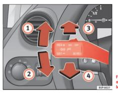
Fig. 77 Turn signal and main beam headlight lever
