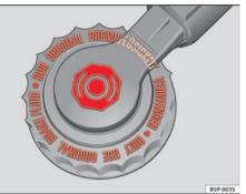
Fig. 167 In the engine compartment: Brake fluid reservoir cover
