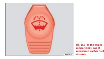
The **windscreen washer** and the **headlight washing system** are supplied with fluid from the windscreen washer fluid container in the engine compartment.
