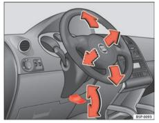
Fig. 128 Adjusting the steering wheel position
