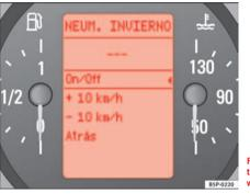
Fig. 46 Digital screen on the instrument panel: winter tyre display
