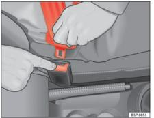
Fig. 16 Removing latch plate from buckle
