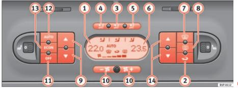
Fig. 127 On the dash panel: 2C Climatronic controls
