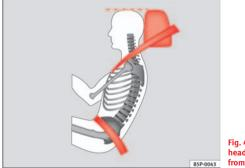
Fig. 4 Properly adjusted head restraint viewed from the side Adjust the head restraint properly to achieve maximum protection.
