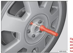
Fig. 175 Wheel change: Hexagon socket in screwdriver handle to turn the wheel bolts after they have been loosened
