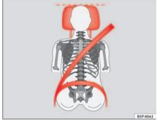
Fig. 90 Viewed from in front: Properly adjusted headrests and proper belt adjustment
