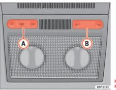
Fig. 78 Detail of the roof: Front reading light
