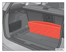
Fig. 103 Variable stowage area in the luggage compartment floor
