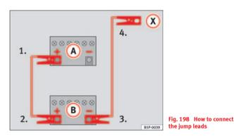
In  $\Rightarrow$  fig. 198, the flat battery is (A) and the charged battery (B).
