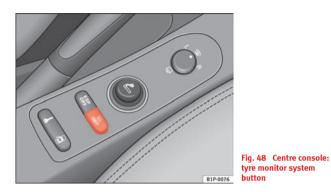
The tyre monitor indicator compares wheel revolutions and uses this information to compare the diameter of each wheel using the ABS sensors. If the diameter of a wheel changes, the tyre monitor indicator lights (1). The wheel diameter changes when:
