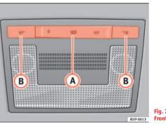
Fig. 79 Detail of the roof: Front reading light
