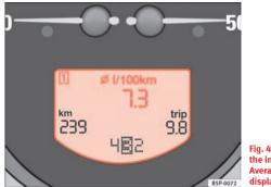
Fig. 40 Digital screen on the instrument panel: Average fuel consumption display
