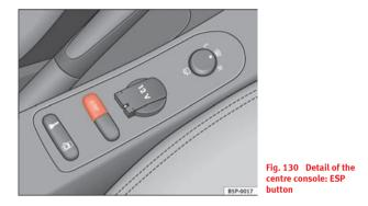
The Electronic Stabilisation Program (ESP) contains the electronic differential lock (EDL) and the traction control system (TCS). The ESP function works in conjunction with the ABS. Both warning lamps will light up if the ESP or ABS systems are faulty.
