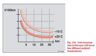
The engine and catalytic converter need to reach their proper **working temperature** in order to minimise fuel consumption and emissions.
