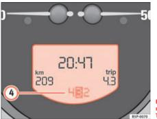
Fig. 37 Detail of instrument panel: Display with Tiptronic gear selection
