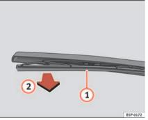
Fig. 166 Changing the rear window wiper blade
