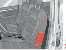
Fig. 22 Side airbag in driver seat
