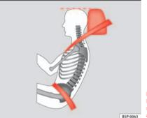
Fig. 91 Viewed from side: Properly adjusted headrests and proper belt adjustment
