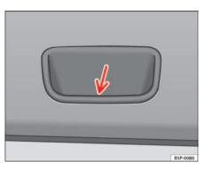
Fig. 67 Detail of the tailgate inner trim: recessed handle for closing the tailgate
