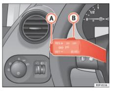
Fig. 145 Turn signal and main beam lever: switch and rocker switch for CCS
