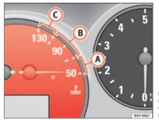
Fig. 35 Details of the instrument panel: Engine coolant temperature gauge
