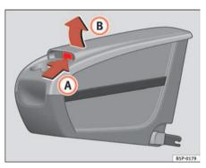
Fig. 111 Mobile stowage compartment Opening
