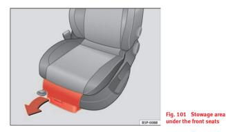
The drawer\*  $\Rightarrow$  fig. 101 (A) is opened by pushing the button and putting the cover back.
