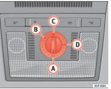
Fig. 70 Detail of the sunroof: rotary button for sliding/tilting sunroof
