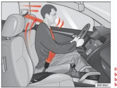
Fig. 11 Driver protected by the properly worn seat belt during a sudden braking manoeuvre.
