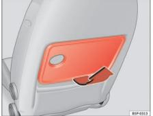
Fig. 102 Folding table for the front left seat
