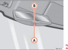
Fig. 88 Automatic antidazzle interior mirror.
