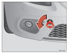
Fig. 207 Front towing eye for vehicles with fourwheel drive
