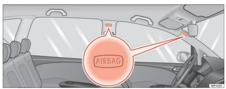
Fig. 24 Location of left curtain airbag
