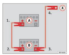
Fig. 204 How to connect the jump leads
