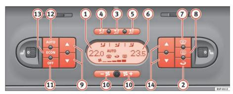
Fig. 133 On the dash panel: 2C Climatronic controls
