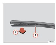
Fig. 171 Changing the rear window wiper blade
