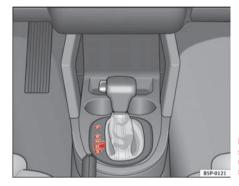
Fig. 140 Central console: selector lever for automatic gearbox / direct shift gearbox DSG
