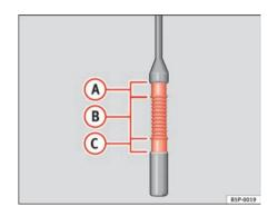
Fig. 165 Engine oil dipstick.
