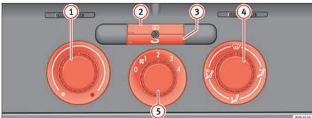
B5P-0110 Fig. 128 On the dash panel: Heater controls
