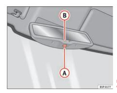
Fig. 90 Automatic antidazzle interior mirror.
