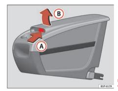
Fig. 114 Mobile stowage compartment Opening
