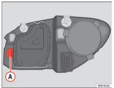
Fig. 186 Turn signal lamps
