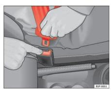
Fig. 16 Removing latch plate from buckle
