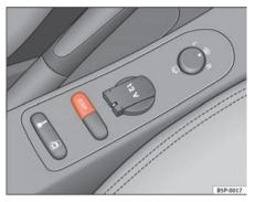
Fig. 136 Detail of the centre console: ESP button
