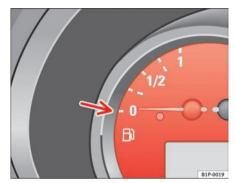
Fig. 34 Instrument panel: fuel gauge
