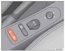
Fig. 60 Detail of the centre console: central locking system button
