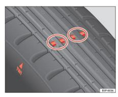
Fig. 173 Tyre tread wear indicators
