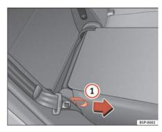
Fig. 99 Folding or opening the rear seat backrests
