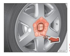
Fig. 176 Changing the wheel: Removing a hub
