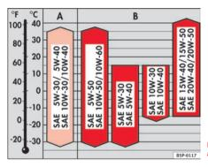
Fig. 164 Types of oil according to temperature
