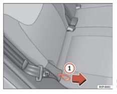
Fig. 98 Rear seat backrest angle adjustment
