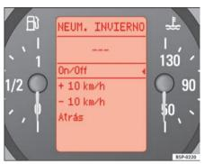
Fig. 46 Digital instrument panel display: winter tyres indicator
