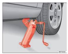
Fig. 179 Fitting the jack
