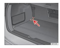
Fig. 127 Fastening rings to tighten the divider net
