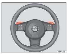
Fig. 145 Steering wheel with levers for automatic gearbox
