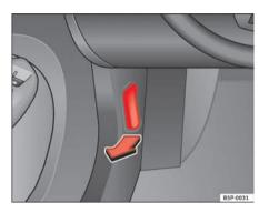
Fig. 162 Detail of footwell area on driver's side: lever for unlocking the bonnet.
