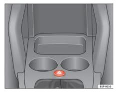
Fig. 77 Instrument panel: switch for hazard warning lights
