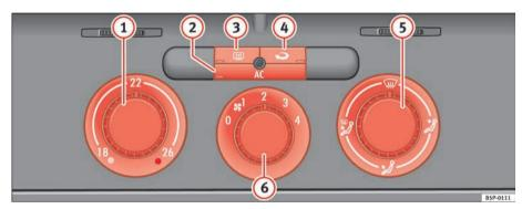
Fig. 130 On the dash panel: Climatic controls
