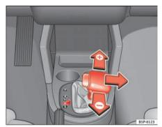
Fig. 144 Changing gear with Tiptronic
