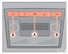
Fig. 82 Interior roof trim: front reading lights, type 2
