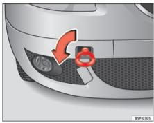
Fig. 205 The front right section of the vehicle: Fitting the front towing eye
