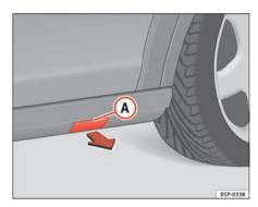
Fig. 180 Plastic sill panel with a cover for the jack anchor
