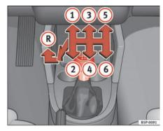
Fig. 139 Detail of the centre console: gear shift pattern of a 6-speed manual gearbox
