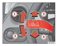
Fig. 78 Turn signal and main beam headlight lever
