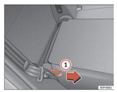
Fig. 100 Folding or opening the front seat backrests
