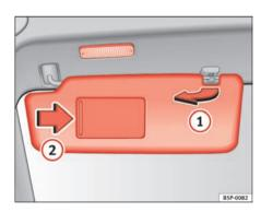
Fig. 84 Sun visor on the driver side
