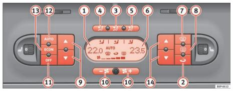
Fig. 132 On the dash panel: 2C Climatronic controls
