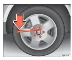
Fig. 177 Changing the wheel: loosen the wheel
