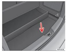
Fig. 175 Luggage compartment. Access to the spare wheel
