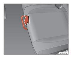
Fig. 97 For unlocking the rear seat
