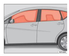
Fig. 25 Deployed curtain airbags
