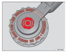
Fig. 172 In the engine compartment: Brake fluid reservoir cover
