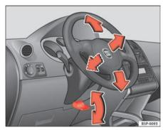
Fig. 134 Adjusting the steering wheel position
