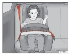
Fig. 29 A category 1 forward-facing child seat fitted on the rear seat.
