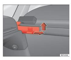
Fig. 125 Removing the luggage compartment cover
