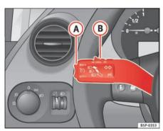
Fig. 150 Turn signal and main beam headlight lever switch and rocker switch for the cruise control
