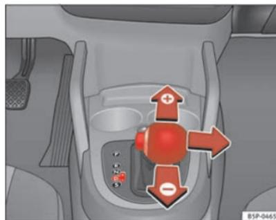
**Fig. 149** Mudar com tiptronic
