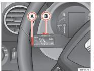
Fig. 156 Turn signal and main beam headlight lever: switch and rocker switch for the cruise control
