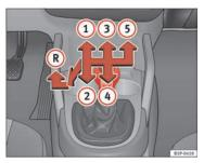
Fig. 143 Detailed view of the centre console: gear shift pattern of a 5-speed manual gearbox
