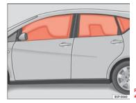
Fig. 25 Deployed curtain airbags
