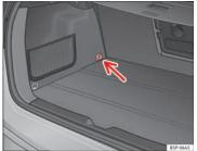
Fig. 32 Top Tether\* securing ring When removing or fitting the child seat, please be sure to follow the manufacturer's instructions.
