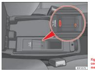
Fig. 123 Connection in central armrest compartment
