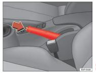
Fig. 151 Handbrake between the front seats
