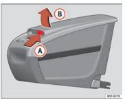
Fig. 115 Mobile storage compartment. Opening
