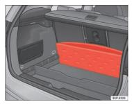
Fig. 107 Variable luggage compartment floor storage compartment
