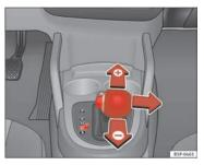
Fig. 149 Changing gear with tiptronic
