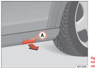
Fig. 181 Plastic sill panel trim with jack allotment cover
