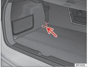
Fig. 127 Anchor rings for the separation net
