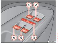
Fig. 69 Detail of the driver door: controls for the front and rear windows
