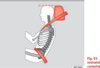
Fig. 93 Side view: head restraints and seat belts correctly adjusted
