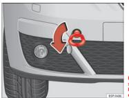
Fig. 207 The front right section of the vehicle: Fitting the front towing eye
