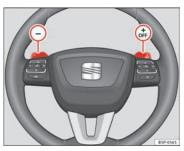
Fig. 150 Steering wheel with levers for automatic gearbox
