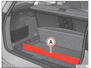
Fig. 108 Variable luggage compartment floor storage compartment
