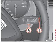
Fig. 45 Windscreen wiper lever: button A to confirm the menu selection and rocker switch B to change the menu
