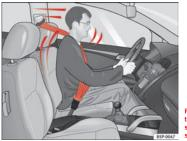
Fig. 11 A driver wearing the seat belt properly is secured by the belt in sharp braking
