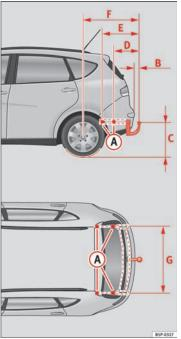
Fig. 159 Attachment points for towing bracket
