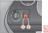
Fig. 75 Dash panel: regulation for instrument and switch illumination and headlight range control
