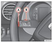
Fig. 155 Turn signal and main beam headlight lever: switch and rocker switch for the cruise control
