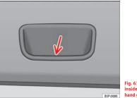
Fig. 67 Detail of the inside of the tailgate: hand grip
