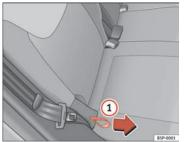
Fig. 99 Rear seat backrest angle adjustment The seats may be moved forwards or backwards independently. The movement can be 1/3 or 2/3 of the seat. There are various possible positions.
