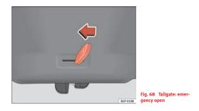
There is a groove in the luggage compartment allowing access to the emergency opening mechanism.
