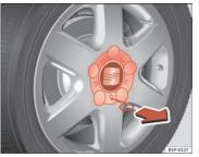
Fig. 177 Changing the wheel: Removing a hub cap
