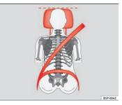
Fig. 13 Correct seat belt and head restraint positions, viewed from front
