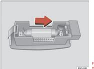
Fig. 204 Removing sun visor light
