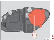
Fig. 190 Main beam headlights
