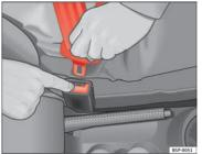
Fig. 16 Removing latch plate from buckle
