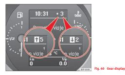
Use the gear display to save fuel. If you are driving in the correct gear, a dot will be shown next to the gear display. If you are not in the correct gear, an arrow will appear next to the gear display indicating whether you should change up or down.
