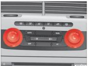
Fig. 97 Front seat heating with Climatronic
