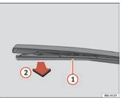
Fig. 172 Changing the rear window wiper blade
