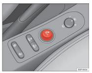
Fig. 118 The cigarette lighter is located in the power socket on the front of the centre console
