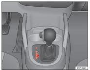
Fig. 145 Centre console: Selector lever for automatic gearbox / DSG automatic gearbox
