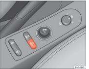
Fig. 52 Centre console: tyre monitor system button
