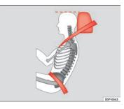
Fig. 14 Correct seat belt and head restraint positions, viewed from side The following features are available to adjust the seat belt in the shoulder region:
