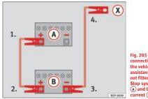
Fig. 205 Diagram for connecting jump leads if the vehicle providing assistance the current is not fitted with the Start-Stop system: flat battery (A) and battery providing current (B).
