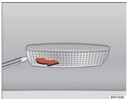
Fig. 203 Removing sun visor light
