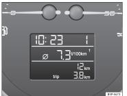
The multifunction system uses two automatic memories: **1** - **Actual memory** and **2** - **Total memory**. The selected memory will be shown in the upper right-hand corner of the display.
