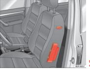
Fig. 22 Side airbag in driver seat
