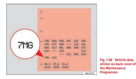
Your vehicle is fitted with a DPF (Diesel particulate filter) if the vehicle data sticker (back cover of the "Maintenance Programme") lists the PR code 7GG or 7MG  $\Rightarrow$  fig. 158.
