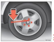
Fig. 178 Changing the wheel: loosen the wheel bolts
