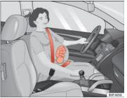
Fig. 15 Positioning seat belts during pregnancy
