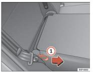
Fig. 101 Folding or opening the front seat backrests
