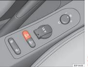
Fig. 138 Detailed view of the centre console: ESP button
