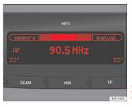
Fig. 134 Radio display with information about Climatronic
