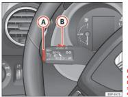
Fig. 154 Turn signal and main beam headlight lever: switch and rocker switch for the cruise control
