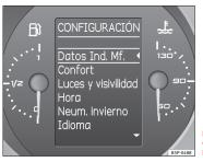
Fig. 49 Multifunction display (MFI) instrument panel display.
