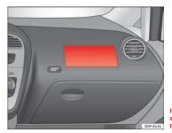
Fig. 19 Front passenger airbag located in dash panel The front airbag for the driver is located in the steering wheel  $\Rightarrow$  fig. 18 and the airbag for the front passenger is located in the dash panel  $\Rightarrow$  fig. 19. Airbags are identified by the word "AIRBAG".
