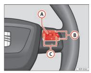
Fig. 46 Steering wheel controls: button A to confirm the menu selection and switch B to change the menu
