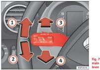
Fig. 78 Turn signal and main beam headlight lever
