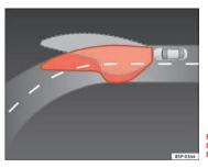
Fig. 76 Cornering lighting using adaptive headlights
