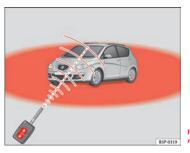
Fig. 65 Range of the remote control
