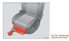
The drawer\*  $\Rightarrow$  fig. 104 (A) is opened by pushing the button and putting the cover back.
