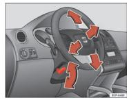
Fig. 136 Adjusting the steering wheel position
