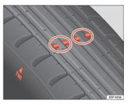
Fig. 174 Tyre tread wear indicators
