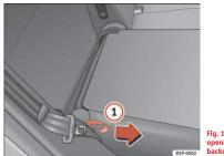
Fig. 100 Folding or opening the rear seat backrests
