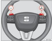
Fig. 150 Steering wheel with levers for automatic gearbox
