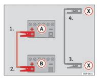
Fig. 206 Diagram for connecting jump leads if the vehicle providing assistance is fitted with the Start-Stop system: flat battery (a) and battery providing current (a).
