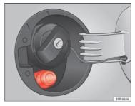
Fig. 164 Fuel tank flap open with EURO-type connector.
