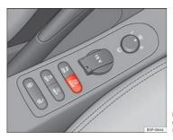
Fig. 140 Centre console: gas system control switch.
