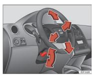
Fig. 136 Adjusting the steering wheel position
