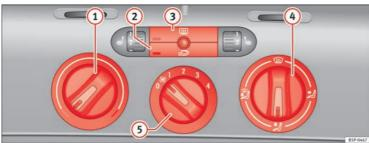
Fig. 128 Heating controls on the dash panel
