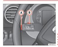
Fig. 156 Turn signal and main beam headlight lever: switch and rocker switch for the cruise con-
