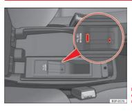
Fig. 123 Connection in central armrest compartment
