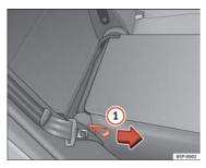
Fig. 100 Folding or opening the rear seat hackrests
