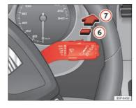
Fig. 89 Windscreen wiper and windscreen wash lever: rear window wiper
