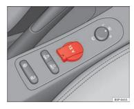
Fig. 119 Power socket in front centre console
