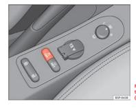
Fig. 138 Detailed view of the centre console: ESC (ESP) button
