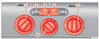
Fig. 129 On the dash panel: Climatic controls
