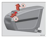
Fig. 115 Mobile storage compartment. Opening
