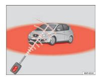
Fig. 65 Range of the remote control
