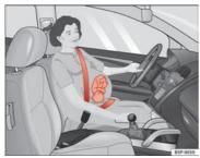
Fig. 15 Positioning seat belts during pregnancy
