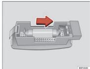
Fig. 204 Removing sun visor light
