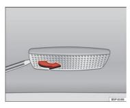
Fig. 203 Removing sun visor light
