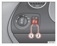
Fig. 75 Dash panel: regulation for instrument and switch illumination and headlight range control
