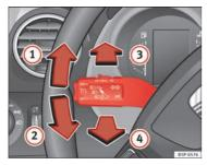
Fig. 78 Turn signal and main beam headlight lever
