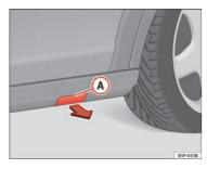
Fig. 182 Plastic sill panel trim with jack allotment cover
