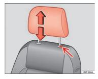
Fig. 94 Adjusting and removing the head restraints
