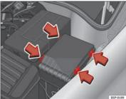
Fig. 185 Fuse box cover in engine compartment
