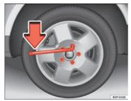
Fig. 179 Changing the wheel: loosen the wheel bolts
