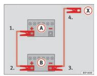
Fig. 205 Diagram for connecting jump leads if the vehicle providing assistance the current is not fitted with the Start-Stop system: flat battery providing current (a).
