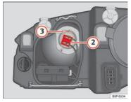
Fig. 189 Dipped beam headlights
