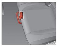
Fig. 98 For unlocking the rear seat
