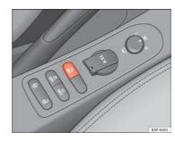
Fig. 152 Centre console: Switch for parking aid
