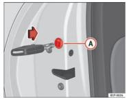
Fig. 60 Locking the doors manually
