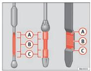
Fig. 167 Engine oil dipstick
