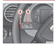
Fig. 157 Turn signal and main beam headlight lever: switch and rocker switch for the cruise control
