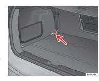
Fig. 127 Anchor rings for the separation net
