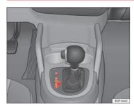
Fig. 145 Centre console: Selector lever for automatic gearbox / DSG automatic gearbox
