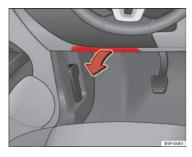
Fig. 184 Left side of dash panel: Fuse box cover
