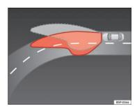
Fig. 76 Cornering lighting using adaptive headlights
