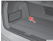
Fig. 32 Top Tether\* securing ring
