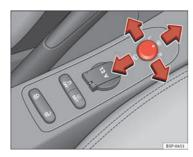
Fig. 91 Controls of exterior mirrors
