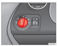
Fig. 73 Detailed view of the dash panel: lights, fog lights and rear fog light switch
