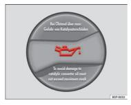
Fig. 168 In the engine compartment: Engine oil filler cap
