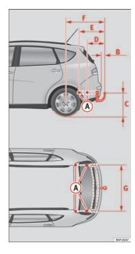
Fig. 159 Attachment points for towing bracket
