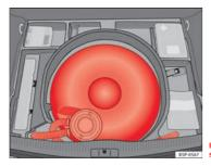
Fig. 162 LPG tank in spare wheel well
