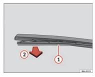
Fig. 173 Changing the rear window wiper blade
