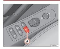
Fig. 141 The Start-Stop function button
