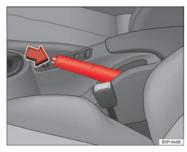
Fig. 151 Handbrake between the front seats
