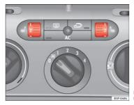
Fig. 96 Thumb wheel for the front seat heating
