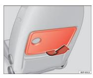
Fig. 105 Folding tray on the front left seat
