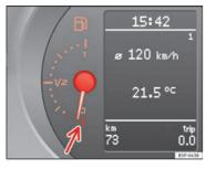
Fig. 35 Instrument panel: fuel gauge
