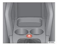
Fig. 77 Dash panel: switch for hazard warning lights
