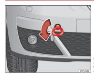
Fig. 207 The front right section of the vehicle: Fitting the front towing eye
