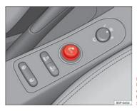
Fig. 118 The cigarette lighter is located in the electric socket on the front of the centre console
