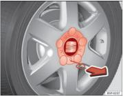
Fig. 178 Changing the wheel: Removing a hub cap
