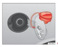
Fig. 160 Tank flap open
