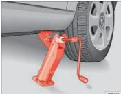
Fig. 181 Fitting the jack
