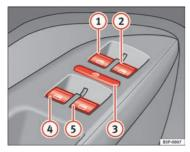
Fig. 69 Detail of the driver door: controls for the front and rear windows
