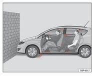
Fig. 7 Vehicle about to hit a wall: the occupants are not wearing seat belts
