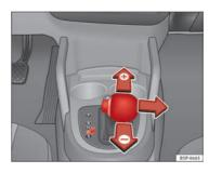
Fig. 149 Changing gear with tiptronic
