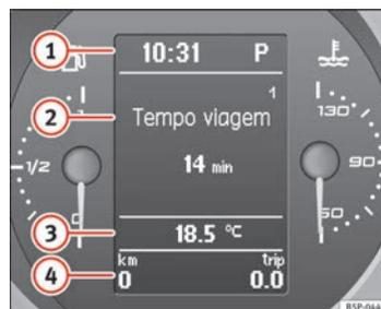
**Fig. 39** Visor digital do painel de instrumentos
