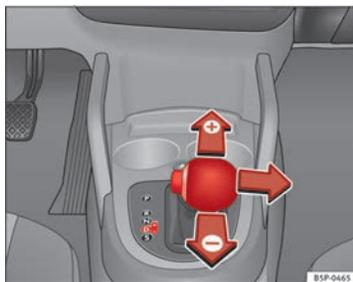
Fig. 148 Engrenar com tiptronic
