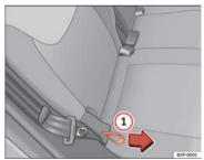
Fig. 98 Rear seat backrest angle adjustment
