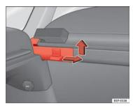
Fig. 124 Removing the rear shelf
