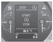
Fig. 141 Display on the instrument panel during Start-Stop function operation.
