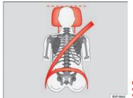
Fig. 91 Front view: head restraints and seat belts correctly adjusted
