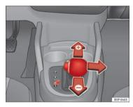
Fig. 148 Changing gear with tiptronic
