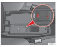
Fig. 122 Connection in central armrest compartment
