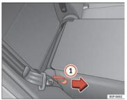
Fig. 99 Folding or opening the rear seat backrests
