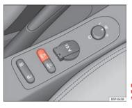
Fig. 137 Detailed view of the centre console: ESC switch.
