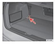
Fig. 126 Fastening rings for the separation net
