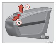
Fig. 114 Mobile storage compartment. Opening
