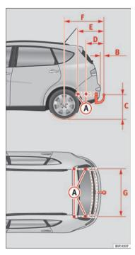
Fig. 158 Attachment points for towing bracket
