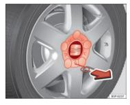
Fig. 177 Changing a wheel: Removing a hub
