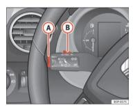
Fig. 154 Turn signal and main beam headlight lever: switch and rocker switch for the cruise control
