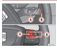
Fig. 43 Rocker buttons A and B. Steering wheel controls.
