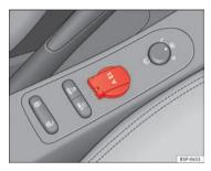
Fig. 118 Power socket in front centre console
