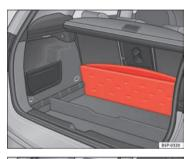
Fig. 106 Variable luggage compartment floor storage compartment
