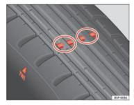
Fig. 174 Tyre tread wear indicators
