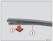
Fig. 172 Changing the rear window wiper blade
