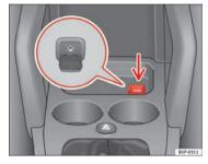
Fig. 120 Auxiliary audio connection
