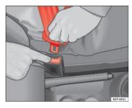
Fig. 16 Remove latch plate from buckle
