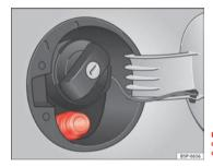
Fig. 163 Fuel tank flap open with EURO-type connector.
