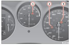
Fig. 51 Instrument panel control and warning lamps in vehicles with LPG.
