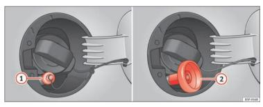
Fig. 160  $\,$  Fuel tank open with LPG filler neck and adapter.
