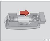
Fig. 203 Removing sun visor light
