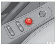
Fig. 117 The cigarette lighter is located in the power socket on the front of the centre console
