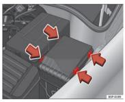
Fig. 184 Fuse box cover in engine compartment
