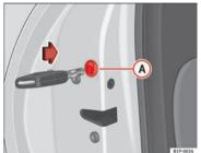
Fig. 60 Locking the doors manually
