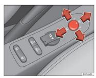
Fig. 90 Controls of exterior mirrors
