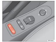
Fig. 59 Detailed view of the centre console: central lock button
