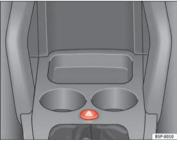
Fig. 76 Dash panel: switch for hazard warning lights
