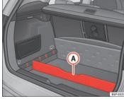
Fig. 107 Variable luggage compartment floor storage compartment
