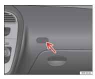
Fig. 27 Control lamp for deactivated front passenger airbag in centre console
