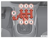
Fig. 143 Detailed view of the centre console: gear shift pattern of a 6-speed manual gearbox
