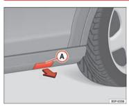
Fig. 181 Plastic sill panel trim with jack allotment cover
