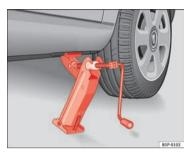
Fig. 180 Fitting the jack
