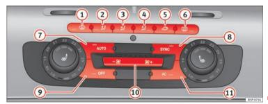
Fig. 134 On the dash panel: 2C Climatronic controls.
