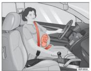
Fig. 15 Positioning seat belts during pregnancy
