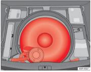
Fig. 161 LPG tank in spare wheel well
