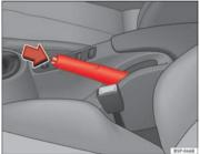
Fig. 150 Handbrake between the front seats
