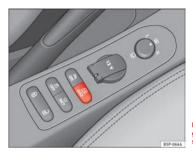
Fig. 139 Centre console: gas system control switch.
