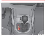
Fig. 144 Centre console: Selector lever for automatic gearbox / DSG automatic gearbox
