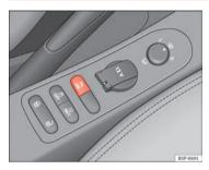
Fig. 151 Centre console: Switch for parking aid
