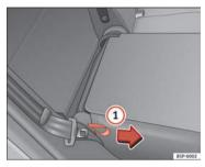
Fig. 100 Folding or opening the rear seat backrest
