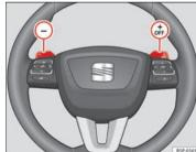
Fig. 149 Steering wheel with levers for automatic gearbox
