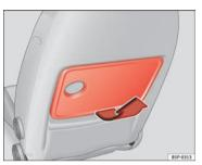
Fig. 104 Folding tray on the front left seat
