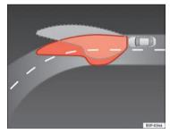
Fig. 75 Cornering lighting using adaptive headlights
