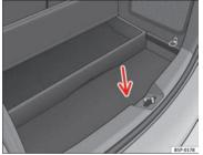
Fig. 176 Luggage compartment. Access to the spare wheel
