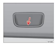
Fig. 67 Close-up of the inside trim of the rear lid: hand grip
