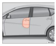
Fig. 23 Inflated side airbag on left side of vehicle
