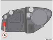
Fig. 186 Turn signal bulb
