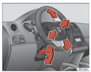
Fig. 135 Adjusting the steering wheel position
