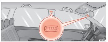
Fig. 24 Location of head airbags on the left side of the vehicle
