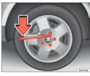
Fig. 178 Changing a wheel: loosen the wheel bolts
