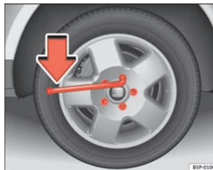
Fig. 178 Changing the wheel: loosen the wheel bolts
