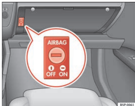
Fig. 26 In the glove compartment: key for enabling and disabling front passenger airbag
