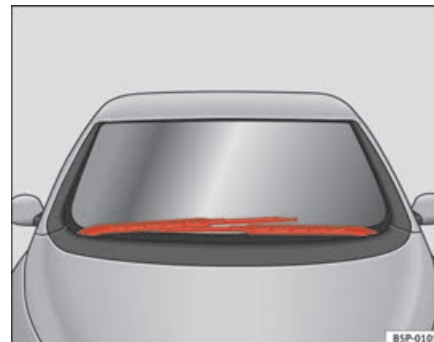
Fig. 170 Windscreen wipers in the service position
