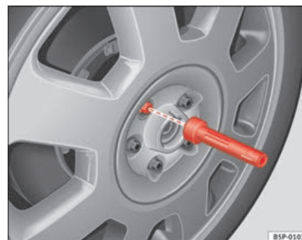
Fig. 182 Changing the wheel: hexagonal socket in screwdriver handle to turn the wheel bolts after they have been loosened
