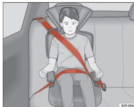
Fig. 30 Forward-facing child seat installed on rear seat.
