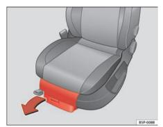
Fig. 103 Stowage area under the front seats
