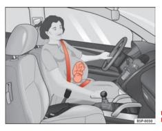
Fig. 15 Positioning seat belts during pregnancy
