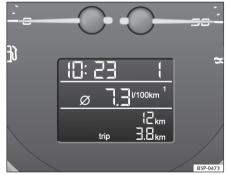
Fig. 40 Digital display in the instrument panel
