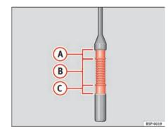
Fig. 158 Engine oil dipstick.
