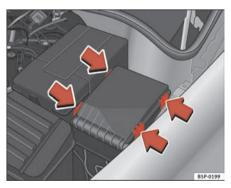
Fig. 178 Fuse box cover in engine compartment
