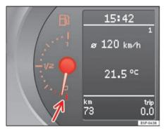
Fig. 34 Instrument panel: fuel gauge
