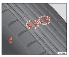
Fig. 167 Tyre tread wear indicators
