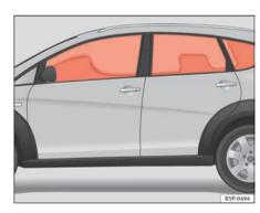
Fig. 25 Deployed curtain airbags
