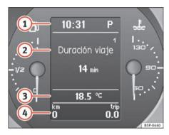
Fig. 37 Digital display in the instrument panel
