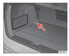
Fig. 126 Anchor rings for the separation net
