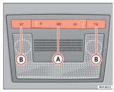
Fig. 81 Interior roof trim: front reading lights, type 2
