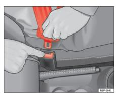
Fig. 16 Removing latch plate from buckle
