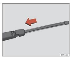
Fig. 165 Mount rear window wiper blade
