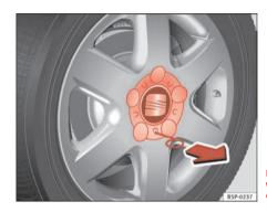
Fig. 170 Changing the wheel: Removing a hub
