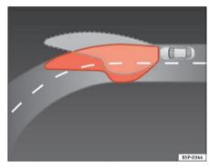
Fig. 75 Cornering lighting using self-directional headlights
