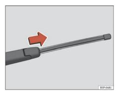
Fig. 164 Remove rear window wiper blade
