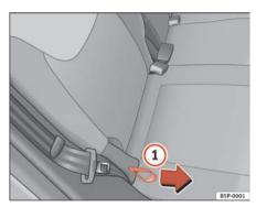
Fig. 98 Rear seat backrest angle adjustment
