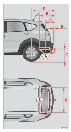
Fig. 153 Attachment points for towing bracket
