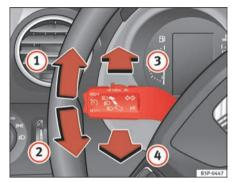
Fig. 77 Indicator and main beam headlight lever
