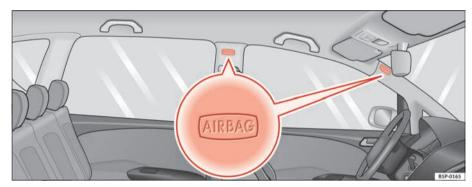
Fig. 24 Location of left curtain airbag
