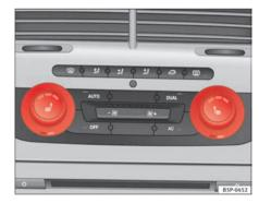
Fig. 96 Front seat heating with Climatronic
