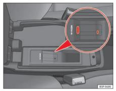
Fig. 122 Connection in central armrest compartment
