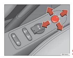
Fig. 90 Controls of exterior mirrors
