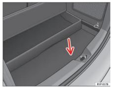
Fig. 169 Luggage compartment. Access to the spare wheel
