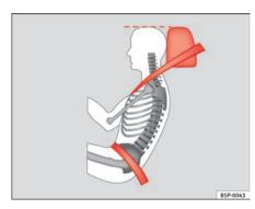
Fig. 92 Side view: head restraints and seat belts correctly adjusted
