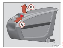
Fig. 114 Mobile stowage compartment Opening
