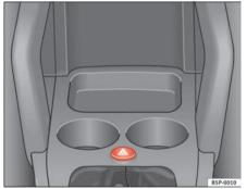
Fig. 76 Instrument panel: switch for hazard warning lights
