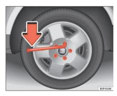
Fig. 171 Changing the wheel: loosen the wheel holts
