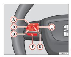
Fig. 52 Controls on the steering wheel
