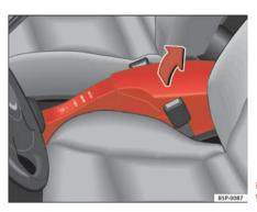
Fig. 102 Front armrest with stowage area
