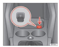
Fig. 120 Auxiliary audio connection
