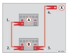
Fig. 198 How to connect the jump leads
