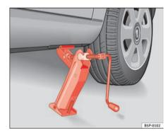
Fig. 173 Fitting the jack
