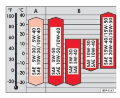
Fig. 157 Types of oil according to temperature
