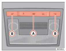
Fig. 79 Interior roof trim: front interior lights
