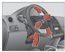
Fig. 135 Adjusting the steering wheel position
