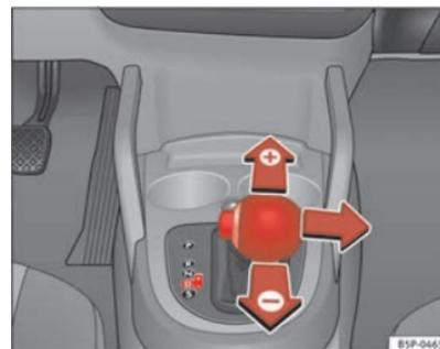
**Fig. 144 Mudar com tiptronic**
