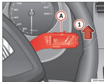
Fig. 86 Windscreen wiper lever
