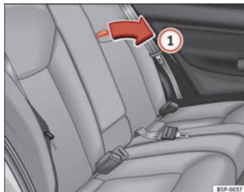
Fig. 109 Opening the rear drink holders
