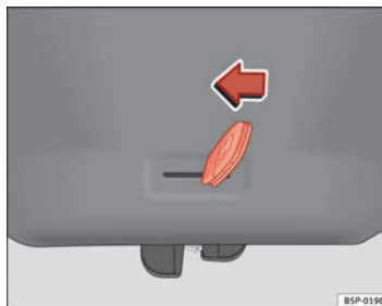
Fig. 66 Tailgate: emergency open
