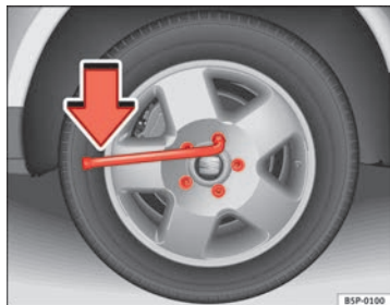
Fig. 171 Changing the wheel: loosen the wheel bolts
