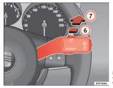
Fig. 88 Window wash and wipe lever: Rear window wiper
