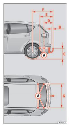
Fig. 149 Attachment points for towing bracket
