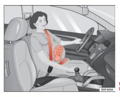
Fig. 15 Positioning seat belts during pregnancy
