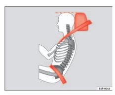
Fig. 92 Viewed from side: Properly adjusted head restraints and proper belt adjustment
