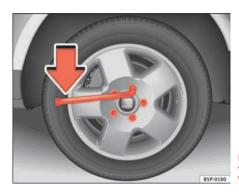
Fig. 166 Changing the wheel: Loosening the wheel bolts
