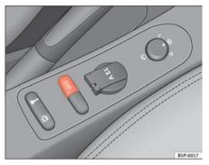
Fig. 129 Detail of the centre console: ESP button
