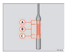
Fig. 154 Engine oil dipstick.
