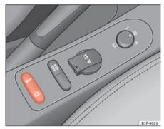
Fig. 60 Detail of rear left door central locking button
