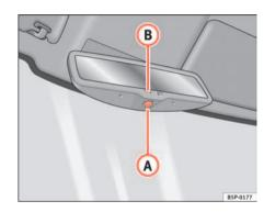
Fig. 89 Automatic antidazzle interior mirror.
