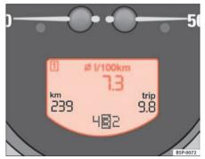
Fig. 40 Digital screen on the instrument panel: Average fuel consumption display
