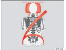
Fig. 91 Viewed from in front: Properly adjusted head restraints and proper belt adjustment
