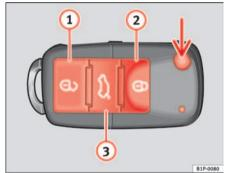
Fig. 64 Assignment of buttons on the remote control key
