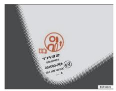
Fig. 6 Head restraint position warning label
