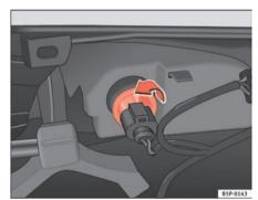
Fig. 185 Lamp on interior side of bumper
