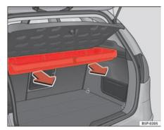
Fig. 120 Removing storage shelf
