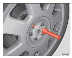
Fig. 169 Wheel change: Hexagon socket in screwdriver handle to turn the wheel bolts after they have been loosened
