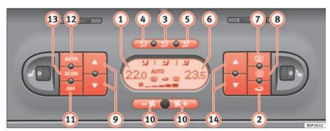
Fig. 126 On the dash panel: 2C Climatronic controls
