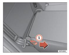
Fig. 98 Folding or opening the rear seat backrests
