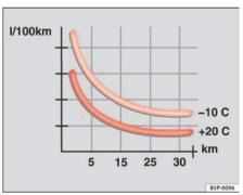
Fig. 148 Fuel consumption in litres per 100 km at two different ambient temperatures
