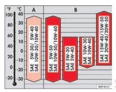
Fig. 153 Types of oil according to temperature
