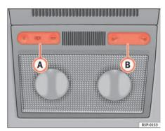
Fig. 79 Detail of the roof: Front reading light
