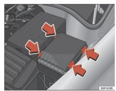
Fig. 172 Fuse box cover in engine compartment
