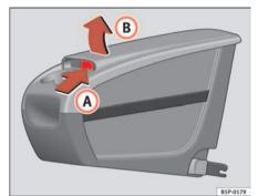
Fig. 111 Mobile stowage compartment Opening
