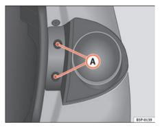
Fig. 181 Side lights and brake lights
