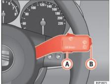
Fig. 39 Windscreen wiper and washer lever: Button A and rocker switch B
