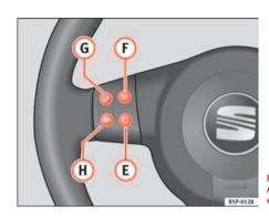
Fig. 56 Steering wheel Audio + Telephone controls
