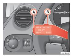
Fig. 142 Turn signal and main beam lever: switch and rocker switch for CCS
