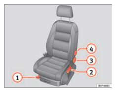
Fig. 94 Front left seat controls
