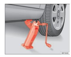
Fig. 168 Fitting the jack
