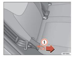
Fig. 97 Rear seat backrest angle adjustment
