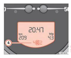
Fig. 37 Detail of instrument panel: Display with Tiptronic gear selection
