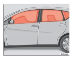
Fig. 25 Deployed curtain airbags
