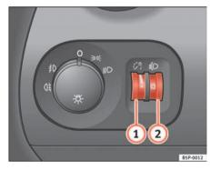
Fig. 76 Detail of the dash panel: Regulation for instrument and switch illumination and headlight range control
