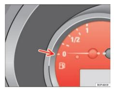
Fig. 34 Details of the instrument panel: Fuel gauge
