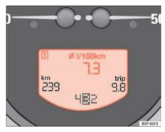
Fig. 42 Digital screen on the instrument panel: Average fuel consumption display
