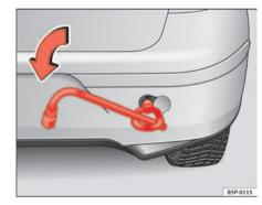
Fig. 195 Fitting the towing eve to the rear of the vehicle
