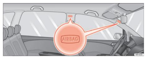
Fig. 24 Location of left curtain airbag
