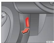
Fig. 151 Detail of the foot well: The release lever for the bonnet is located in the driver side foot well
