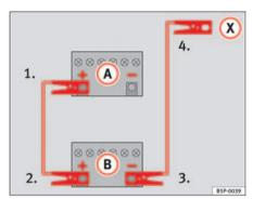
Fig. 193 How to connect the jump leads
