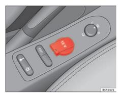
Fig. 115 Socket, centre console, front
