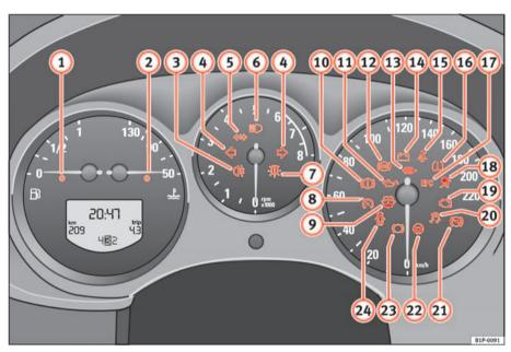
Fig. 47 Instrument panel with warning lamps. Some of the warning lamps listed in this section are only fitted on certain models or are optional extras.
