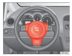
Fig. 18 Driver airbag located in steering wheel
