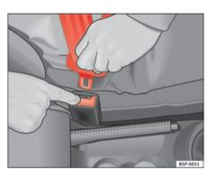
Fig. 16 Removing latch plate from buckle
