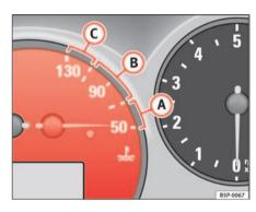
Fig. 35 Details of the instrument panel: Engine coolant temperature gauge
