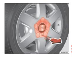
Fig. 165 Changing a wheel: Removing the wheel trim
