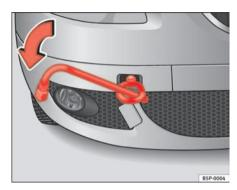
Fig. 194 The front right section of the vehicle: Fitting the front towing
