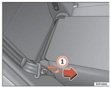
Fig. 99 Folding or opening the front seat backrests
