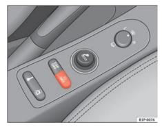
Fig. 48 Centre console: tyre monitor system button
