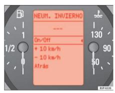
Fig. 46 Digital screen on the instrument panel: winter tyre display
