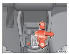
Fig. 137 Changing gear with Tiptronic
