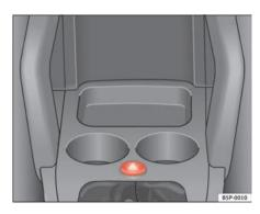
Fig. 77 Detail of the dash panel: Hazard warning light switch
