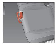
Fig. 96 For unlocking the rear seat
