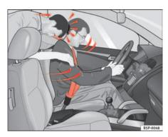
Fig. 10 The unbelted rear passenger is thrown forward violently, hitting the driver wearing a seat
