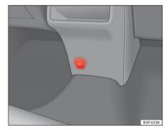
Fig. 116 Socket, centre console, rear
