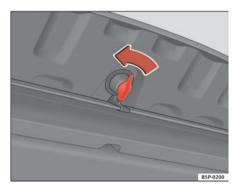
Fig. 118 Opening the storage compartment
