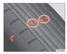
Fig. 162 Tyre tread wear indicators
