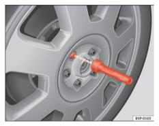
Fig. 176 Wheel change: Hexagon socket in screwdriver handle to turn the wheel bolts after they have been loosened
