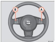
Fig. 57 Steering wheel Audio + Telephone version controls
