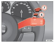
Fig. 87 Window wash and wipe lever: Rear window wiper
