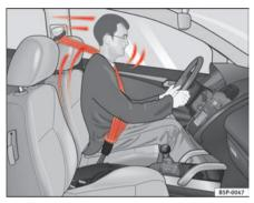
Fig. 11 Driver protected by the properly worn seat belt during a sudden braking manoeuvre.
