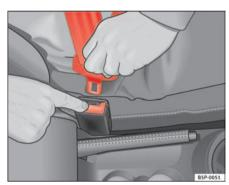
Fig. 16 Removing latch plate from buckle
