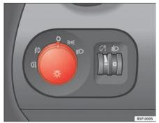
Fig. 73 Detail of the dash panel: Switch for lights, fog lights and rear fog light
