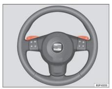
Fig. 140 Steering wheel with levers for the automatic gearbox
