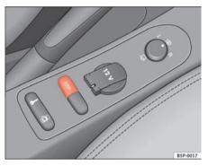
Fig. 131 Detail of the centre console: ESP button
