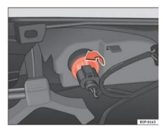
Fig. 192 Lamp on interior side of bumper
