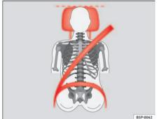
Fig. 90 Viewed from in front: Properly adjusted head restraints and proper belt adjustment
