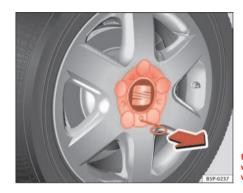
Fig. 172 Changing a wheel: Removing the wheel trim
