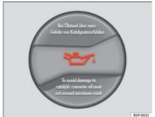
Fig. 162 In the engine compartment: Engine oil filler cap
