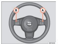
Fig. 58 Steering wheel audio version controls
