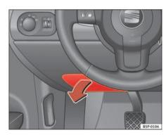
Fig. 178 Left side of dash panel: Fuse box cover
