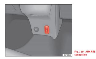
This connector may be used as an audio input (red and white connectors) or audio and video connector (red, white and yellow connectors). For more details about the use of this audio and video source, see the RSE manual.
