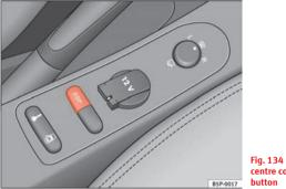
Fig. 134 Detail of the centre console: ESP button
