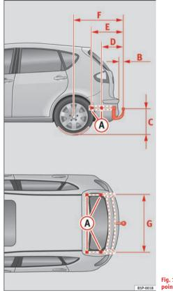
Fig. 158 Attachment points for towing bracket
