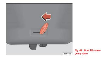
There is a groove in the boot allowing access to the emergency opening mechanism.
