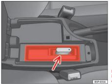
Fig. 120 iPod connection in central armrest compartment.
