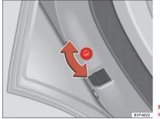
Fig. 61 Child safety lock on the left hand side door
