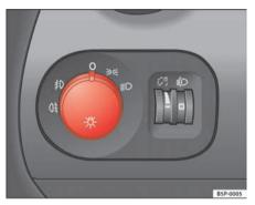
Fig. 73 Detailed view of dash panel lights, fog light and rear fog light control
