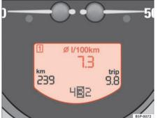
Fig. 40 Digital instrument panel display: average fuel consumption indicator
