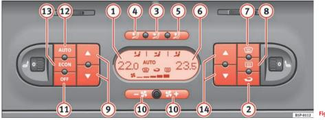
Fig. 131 On the dash panel: 2C Climatronic controls
