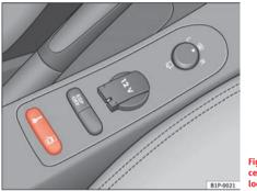
Fig. 60 Detail of the centre console: central locking system button
