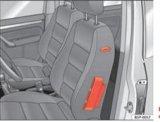
Fig. 22 Side airbag in driver seat
