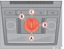
Fig. 71 Roof lining description: rotary sun roof control
