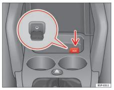
Fig. 118 Auxiliary audio connection
