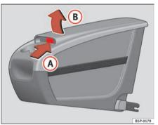
Fig. 113 Mobile stowage compartment Opening
