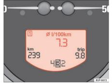
Fig. 42 Digital instrument panel display: average fuel consumption indicator.
