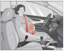
Fig. 15 Positioning seat belts during pregnancy
