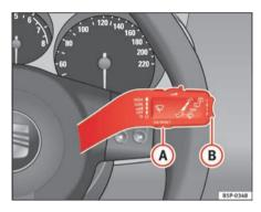
Fig. 41 Windscreen wiper and windscreen wash lever: button A and rocker switch B
