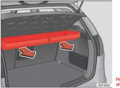
Fig. 125 Removing storage shelf
