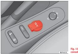
Fig. 117 Socket, centre console, front
