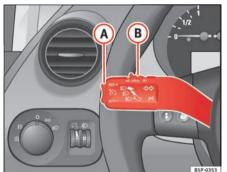
Fig. 148 Turn signal and main beam headlight lever switch and rocker switch for the cruise control
