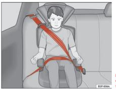
Fig. 30 Forward-facing child seat installed on rear seat.
