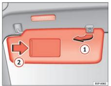
Fig. 84 Sun visor on the driver side
