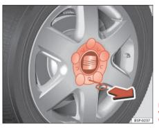
Fig. 174 Changing the wheel: Removing a hub cap
