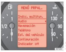
Fig. 44 Digital instrument panel display: Main menu
