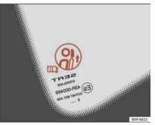
Fig. 6 Head restraint position warning label
