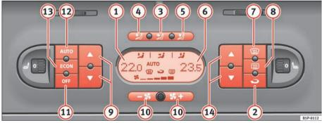
Fig. 130 On the dash panel: 2C Climatronic controls
