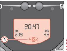
Fig. 37 Detail of the instrument cluster: screen with Tiptronic gear indicator
