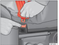
Fig. 16 Removing latch plate from buckle
