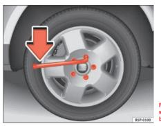
Fig. 175 Changing the wheel: loosen the wheel bolts
