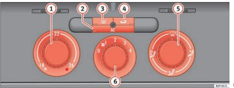
Fig. 127 On the dash panel: Climatic controls
