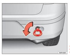
Fig. 204 Fitting the towing eye to the rear of the vehicle
