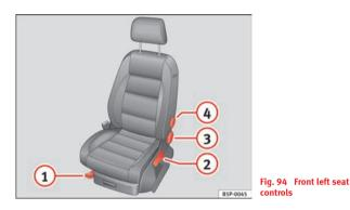
The control elements in  $\Rightarrow$  fig. 94 are mirrored for the front righthand seat.
