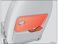
Fig. 103 Folding table of front left seat
