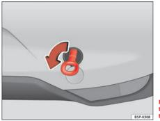
Fig. 208 Fitting the towing eye to the rear of the vehicle
