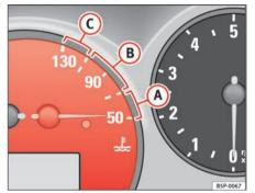
Fig. 35 Instrument panel: engine coolant temperature gauge
