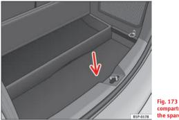
Fig. 173 Luggage compartment. Access to the spare wheel
