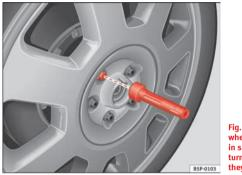
Fig. 178 Changing the wheel: hexagonal socket in screwdriver handle to turn the wheel bolts after they have been loosened
