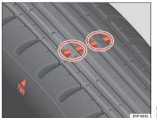
Fig. 171 Tyre tread wear indicators
