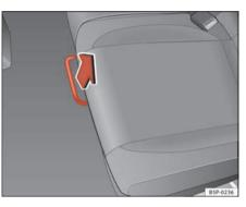
Fig. 96 For unlocking the rear seat
