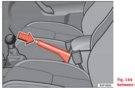
Fig. 144 Handbrake between the front seats
