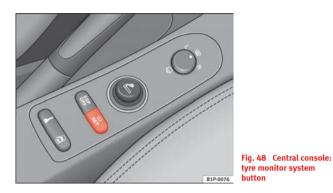
The tyre monitor<sup>14)</sup> compares wheel revolutions and with this information, the diameter of each wheel using the ESP sensors. If the diameter of a wheel changes, the tyre monitor indicator lights (1). The wheel diameter changes when:
