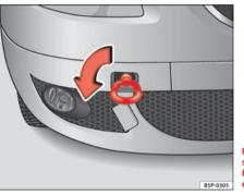
Fig. 203 The front right section of the vehicle: Fitting the front towing eve
