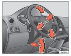
Fig. 132 Adjusting the steering wheel position
