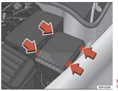
Fig. 181 Fuse box cover in engine compartment
