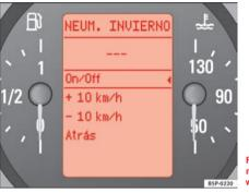
Fig. 46 Digital instrument panel display: winter tyres indicator
