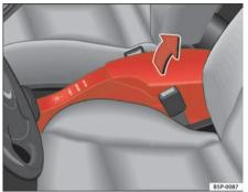
Fig. 101 Front armrest with stowage area
