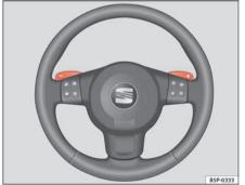
Fig. 143 Steering wheel with levers for automatic gearbox
