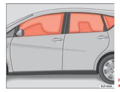
Fig. 25 Deployed curtain airbags
