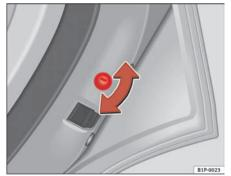
Fig. 62 Child safety lock on the right hand side door This function is independent of the electronic opening and locking systems of the vehicle. It only affects the rear doors. It is only possible to activate it and deactivate it manually, as described below:
