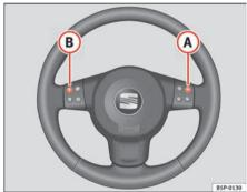
Fig. 58 Steering wheel audio version controls
