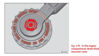
Read off the fluid level at the transparent brake fluid reservoir. It should always be between the "MIN" and "MAX" marks.
