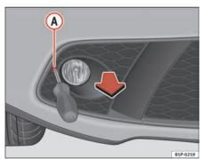
Fig. 205 Access to towing eve housing
