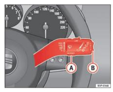
Fig. 45 Windscreen wiper lever: button A to confirm the menu selection and rocker switch B to change the menu
