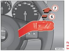
Fig. 88 Windscreen wiper and windscreen wash lever: rear window wiper
