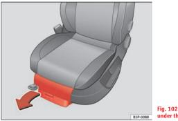
Fig. 102 Stowage area under the front seats
