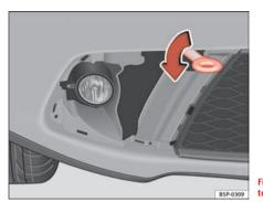
Fig. 206 Attachment for towing eve
