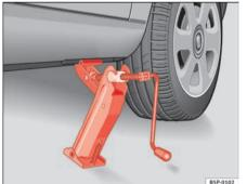
Fig. 177 Fitting the jack
