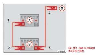
In  $\Rightarrow$  fig. 202, the flat battery is (A) and the charged battery (B).
