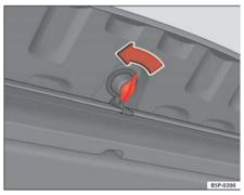
The warning triangle\* is located in a stowage box under the luggage compartment cover  $\Rightarrow$  page 146, fig. 122. To open this storage compartment, turn the knob 90° fig.  $\Rightarrow$  page 146, fig. 123.
