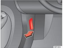
Fig. 160 Detail of footwell area on driver's side: lever for unlocking the bonnet.
