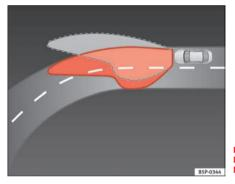
Fig. 76 Cornering lighting using directional headlights
