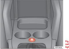
Fig. 77 Instrument panel: switch for hazard warning lights
