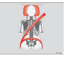
Fig. 13 Correct belt web and head restraint positions, viewed from front
