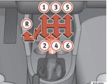
Fig. 137 Detail of the centre console: gear shift pattern of a 6-speed manual gearbox
