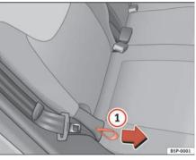
Fig. 97 Rear seat backrest angle adjustment The seats may be moved forwards or backwards independently. The movement can be 1/3 or 2/3 of the seat. There are various possible positions.
