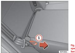
Fig. 99 Folding or opening the front seat backrests
