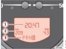
Fig. 36 Detail of the instrument cluster: screen with different indicators
