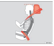
Fig. 14 Correct belt web and head restraint positions, viewed from side The following features are available to adjust the seat belt in the shoulder region:
