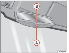
Fig. 89 Automatic antidazzle interior mirror.
