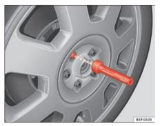
Fig. 173 Changing the wheel: Hexagonal socket in screwdriver handle to turn the wheel bolts
