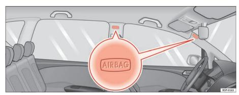
Fig. 24 Location of left curtain airbag
