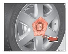
Fig. 169 Changing the wheel: Removing a hub
