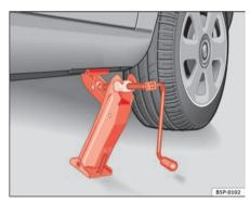
Fig. 172 Fitting the jack
