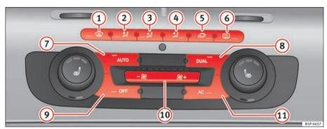
Fig. 129 On the dash panel: 2C Climatronic controls
