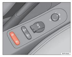
Fig. 58 Detail of the centre console: central locking system button
