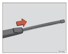
Fig. 163 Remove rear window wiper blade
