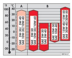
Fig. 156 Types of oil according to temperature
