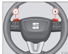
Fig. 144 Steering wheel with levers for automatic gearbox
