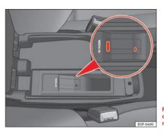
Fig. 120 Connection in central armrest compartment
