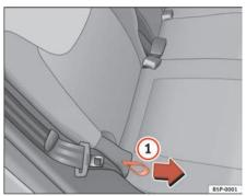
Fig. 97 Rear seat backrest angle adjustment
