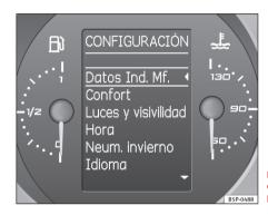
Fig. 47 Multifunction display (MFD) instrument panel display.
