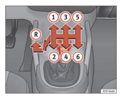
Fig. 138 Detail of the centre console: gear shift pattern of a 6-speed manual gearbox
