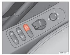
Fig. 146 Centre console: Switch for parking aid
