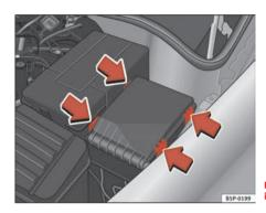
Fig. 176 Fuse box cover in engine compartment
