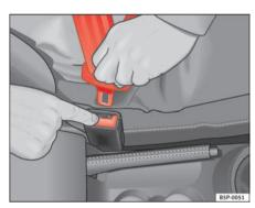
Fig. 16 Removing latch plate from buckle
