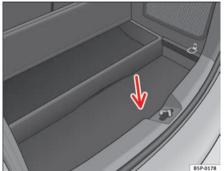
Fig. 168 Luggage compartment. Access to the spare wheel
