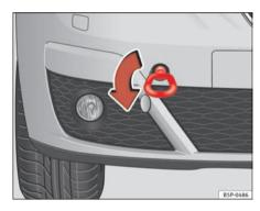
Fig. 198 The front right section of the vehicle: Fitting the front towing eve
