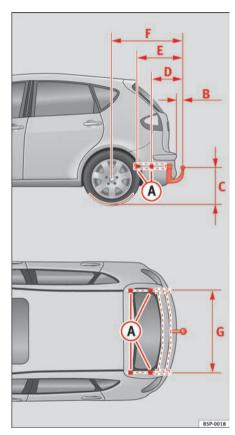
Fig. 152 Attachment points for towing bracket
