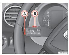
Fig. 147 Indicator and main beam headlight lever: switch and rocker switch for the cruise control
