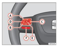
Fig. 54 Controls on the steering wheel
