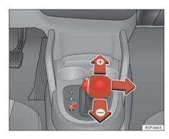
Fig. 143 Changing gear with Tiptronic
