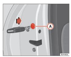
Fig. 59 Locking the doors manually
