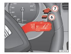
Fig. 87 Windscreen wiper and windscreen wash lever: rear window wiper
