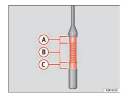
Fig. 157 Engine oil dipstick.
