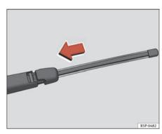
Fig. 164 Mount rear window wiper blade
