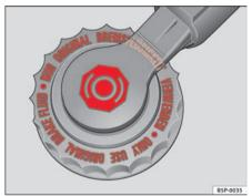
Fig. 165 In the engine compartment: Brake fluid reservoir cover
