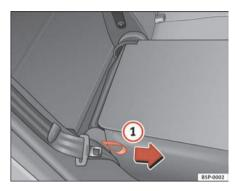
Fig. 99 Folding or opening the front seat backrests
