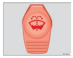
Fig. 160 In the engine compartment: Cap of windscreen washer fluid reservoir.
