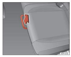
Fig. 96 For unlocking the rear seat
