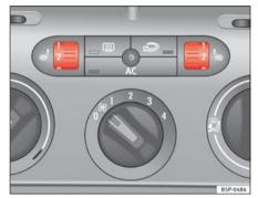
Fig. 94 Thumb wheel for the front seat heating
