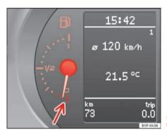
Fig. 34 Instrument panel: fuel gauge
