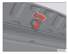
Fig. 122 Opening the storage compartment
