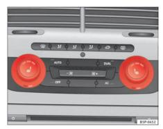
Fig. 95 Front seat heating with Climatronic
