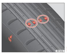
Fig. 166 Tyre tread wear indicators
