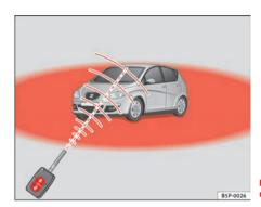
Fig. 64 Range of the remote control:
