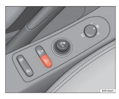
Fig. 49 Centre console: tyre monitor system button
