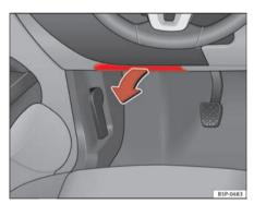
Fig. 175 Left side of dash panel: Fuse box cover
