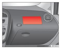
Fig. 19 Front passenger airbag located in dash panel
