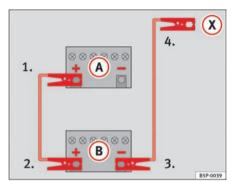
Fig. 197 How to connect the jump leads
