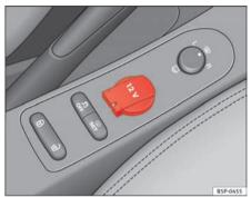
Fig. 117 Socket, centre console, front
