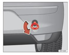
Fig. 199 Fitting the towing eye to the rear of the vehicle
