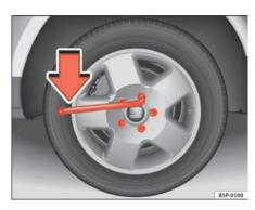
Fig. 170 Changing the wheel: loosen the wheel holts
