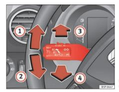
Fig. 77 Indicator and main beam lever
