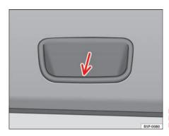
Fig. 66 Detail of the inside of the tailgate: hand grip
