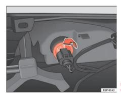
Fig. 189 Lamp on interior side of bumper
