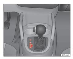
Fig. 139 Centre console: selector lever for automatic gearbox / direct shift gearbox DSG
