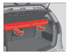
Fig. 124 Removing storage shelf
