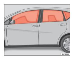
Fig. 25 Deployed curtain airbags
