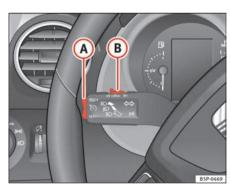
Fig. 151 Indicator and main beam headlight lever: switch and rocker switch for the cruise control
